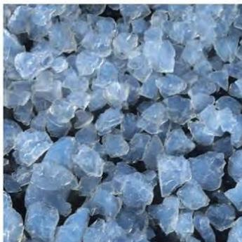
The superior properties of translucent Lumira aerogel, make it the obvious choice for insulating a wide variety of daylighting systems from glass to polycarbonate. Its light transmitting nature and superior thermal mean enhanced energy efficiency while enabling a wide range of commercial and residential building design choices. Benefits include:
