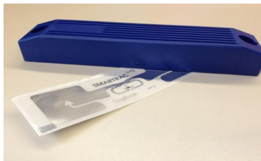
Figure 13: Size difference between passive and active tags
