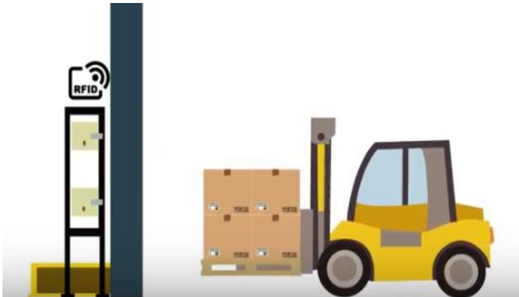
Figure 20: RFID reader receiving the information sent by the RFID tags at the inbound gate
