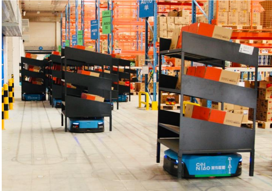
Figure 50: Quicktron robots moving shelves to the operators
