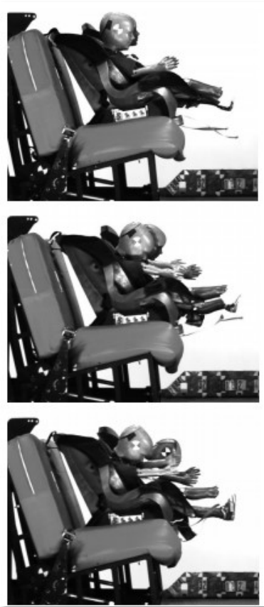
Figure 25 – Head excursion of children with tethered (front) and untethered (rear) top strap of the LATCH [41]
