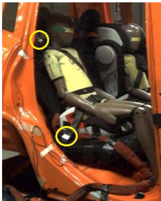
Figure 109 – Location of lap and shoulder belt tensiometers
