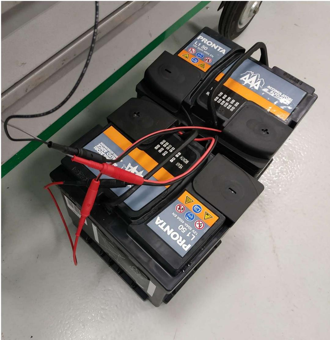
**Figura 5.2– Batterie collegate in serie**
