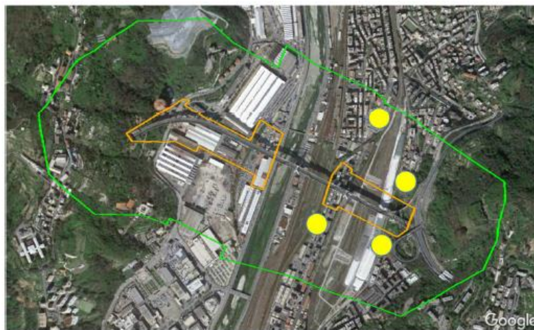
Figure 27: Location of airborne fibers monitoring points - Eastern part [47]
