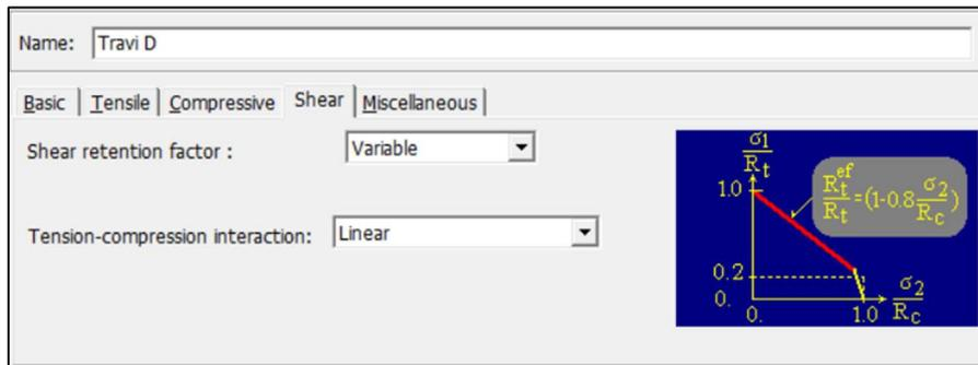
Figure 4.8: Shear tab (tension-compression interaction) for *SBeta Material*
