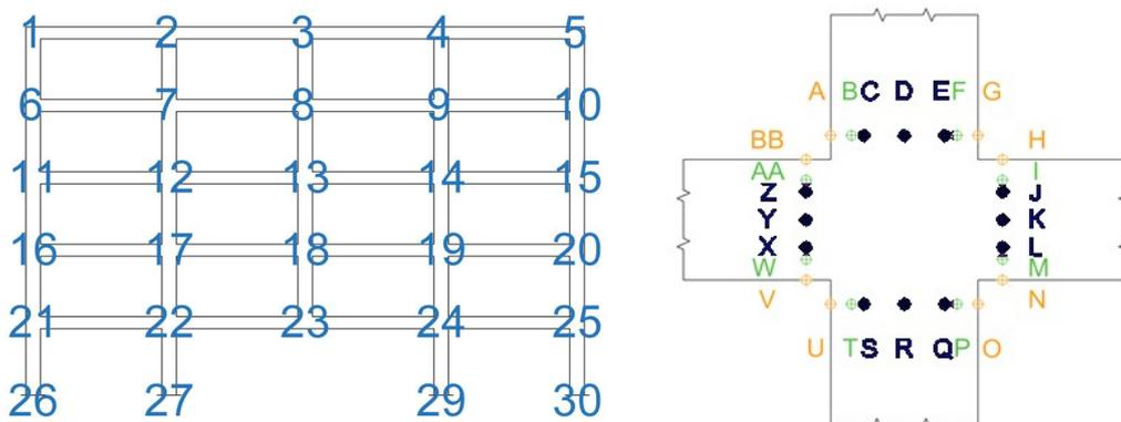
Figure 5.30: Scheme for the strains evaluation: a) location of the sections; b) location of the nodes per each section
