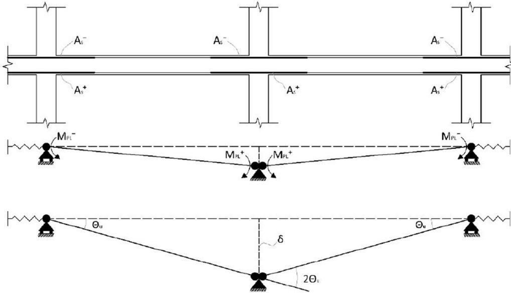
Figure 1.11: Symbols and conventions moments and rotations in the plastic hinges (CNR-DT 214 2018)
