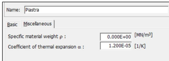
Figure 4.13: Miscellaneous tab for *Plane Stress Elastic Isotropic*
