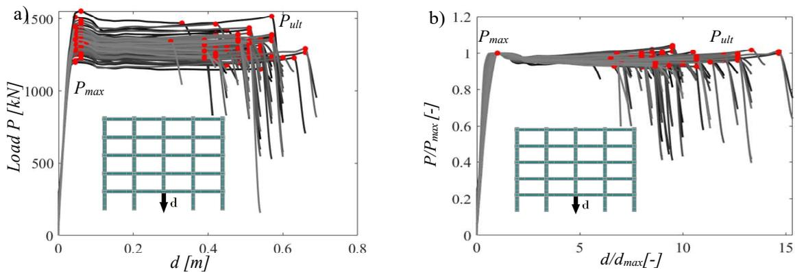
Figure 5.22: Results of pushdown analysis on the  $N$  simulations, showing the collapse branch: a) curve displacement-load; b) capacity curve non-dimensional with respect to the peak values
