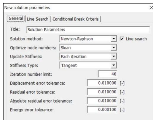
Figure 4.42: *New solution parameters* (General section)
