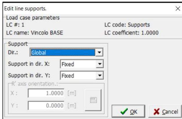
Figure 4.26: Application of *Supports* load case to the lines of the columns' basis
