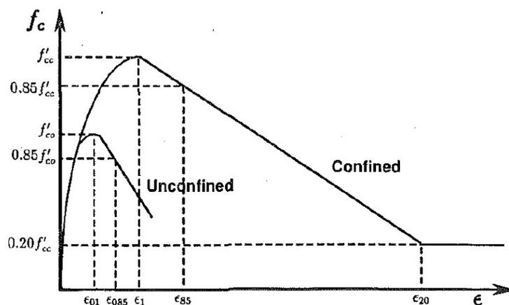
Figure 5.14: Stress-strain Relationship, unconfined vs confined concrete (Saatcioglu and Razvi [32])
