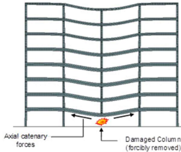
Figure 1.2: Formation of catenary action in a damaged building (<http://www-personal.umich.edu/~eltawil/catenary-action.html>)
