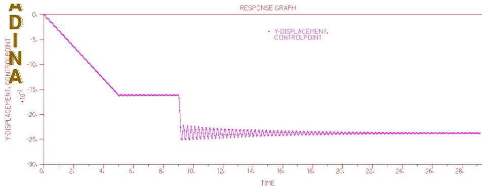
Figure 5.29: Output of the Dynamic Linear analysis on ADINA: displacement versus time
