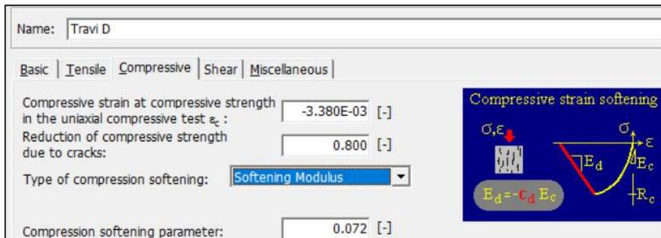
Figure 4.6: Compressive tab for *SBeta Material*
