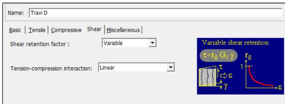
Figure 4.7: Shear tab (retention factor) for *SBeta Material*
