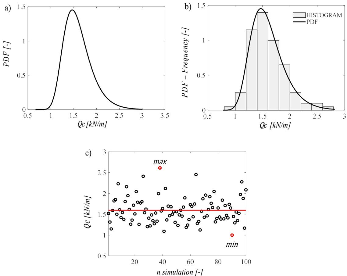
Figure 5.12: Roofing variable load - Gumbel distribution: a) Probability density function; b) Histogram and Distribution fit; c) Scatter plot
