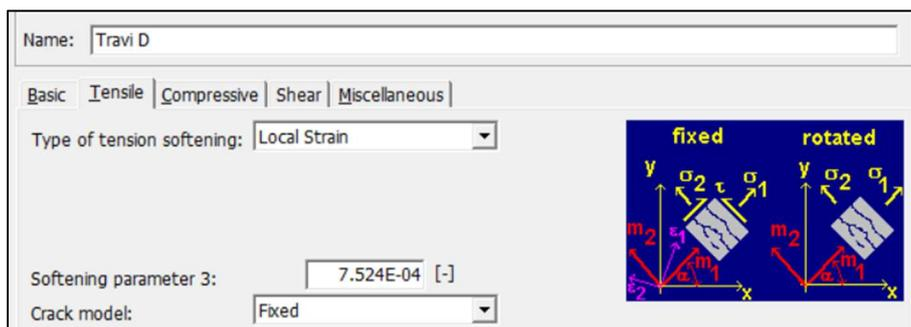
Figure 4.5: Tensile tab (crack model) for *SBeta Material*
