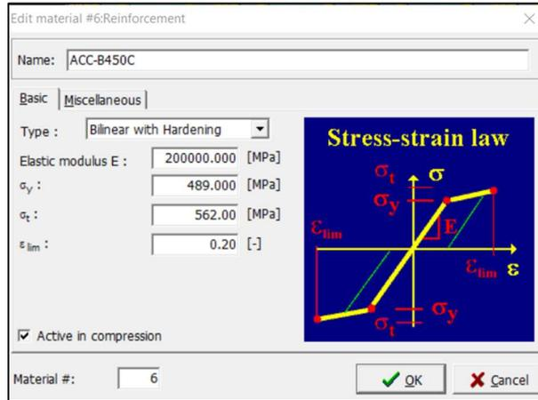
Figure 4.10: Basic tab for *Reinforcement*
