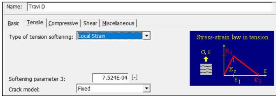
Figure 4.4: Tensile tab (type of tension softening) for *SBeta Material*
