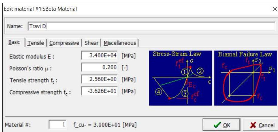
Figure 4.3: Basic tab for *SBeta Material*
