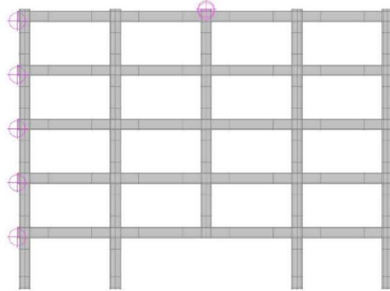
Figure 5.21: Location of the monitoring points on the 2D frame for the Analysis 2 - Pushdown Analysis
