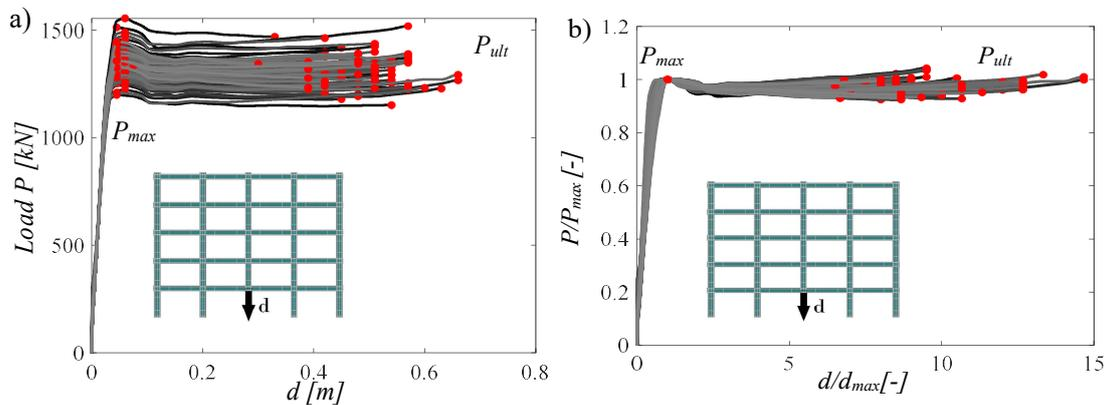
Figure 5.23: Results of pushdown analysis on the  $N$  simulations, stopped at the ultimate value: a) curve displacement-load; b) capacity curve non-dimensional with respect to the peak values
