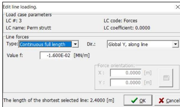
Figure 4.32: Application of *Forces load case* to the lines of the beams
