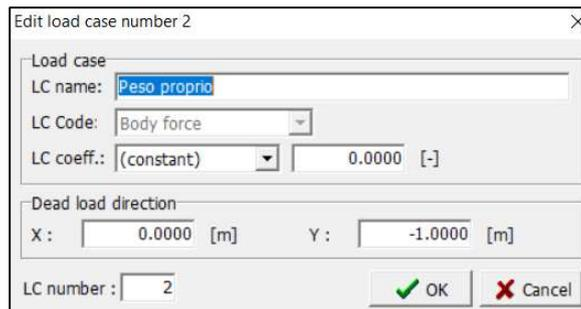
Figure 4.29: Definition of *Body force load case* through load case tab
