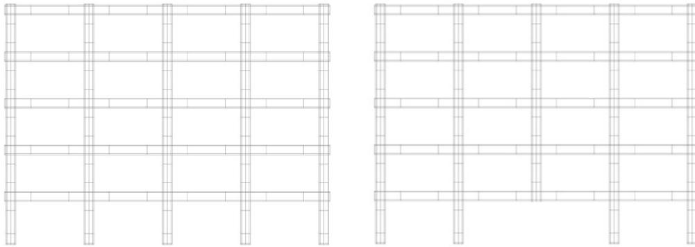
Figure 5.17: Lines representation of the 2D frame: in the left model with column, in the right, model without the column
