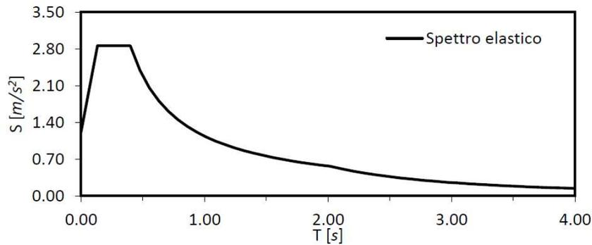
Figure 3.6: Response spectrum at SLS
