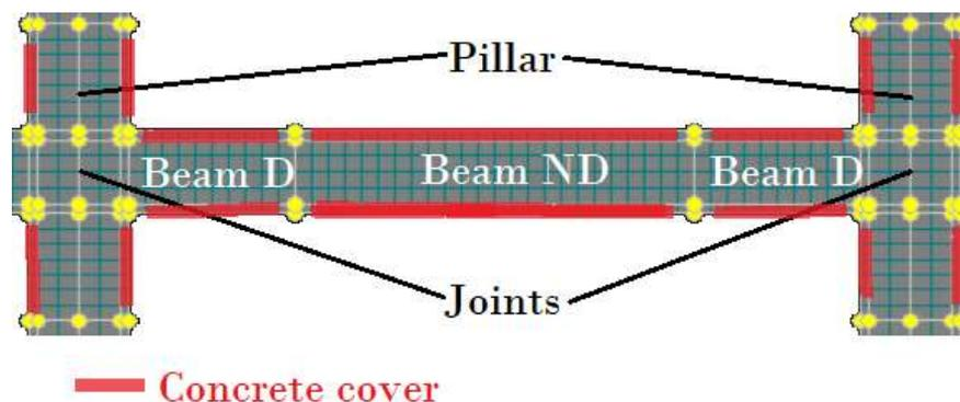
Figure 5.13: Scheme for Material 1 (Beam D), Material 2 (Beam ND), Material 3 (Column) and Material 4 (Joints) and Material 5 (NC Concrete)
