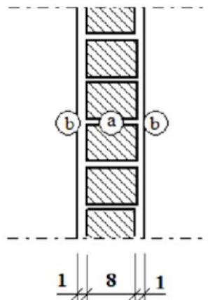
Figure 3.4: Scheme of the internal walls (dimensions in cm)
