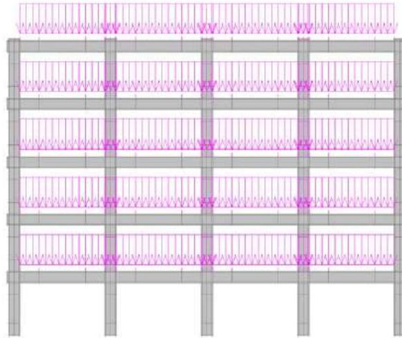
Figure 4.34: Representation of the 2D frame with distributed line loads on the beams
