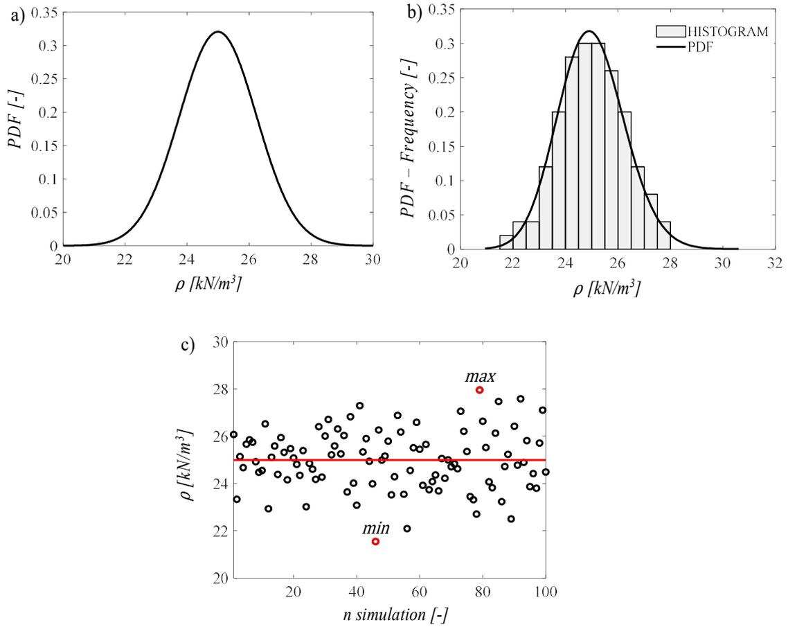
Figure 5.7: Reinforced concrete specific-weight - Normal distribution: a) Probability density function; b) Histogram and Distribution fit; c) Scatter plot
