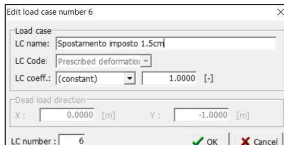
Figure 4.35: Definition of *Prescribed deformation load case* through load case tab
