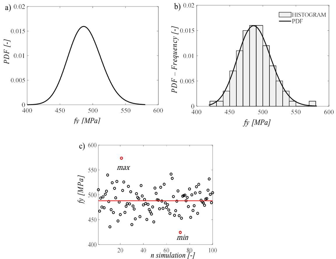
Figure 5.2: Steel yield strength - Lognormal distribution: a) Probability density function; b) Histogram and Distribution fit; c) Scatter plot
