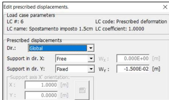
Figure 4.36: Application of *Prescribed deformation load case* to the joint on top of the central column
