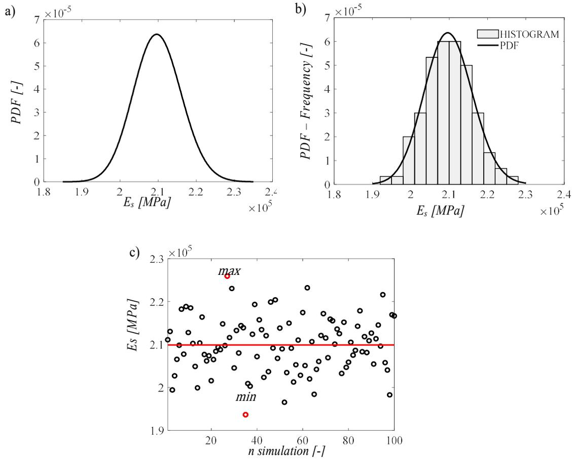
Figure 5.5: Steel Elastic Modulus - Lognormal distribution: a) Probability density function; b) Histogram and Distribution fit; c) Scatter plot
