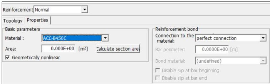
Figure 4.23: Reinforcement definition through *Reinforcement* tab (property section)
