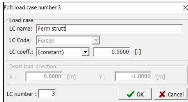
Figure 4.31: Definition of *Forces load case* through load case tab
