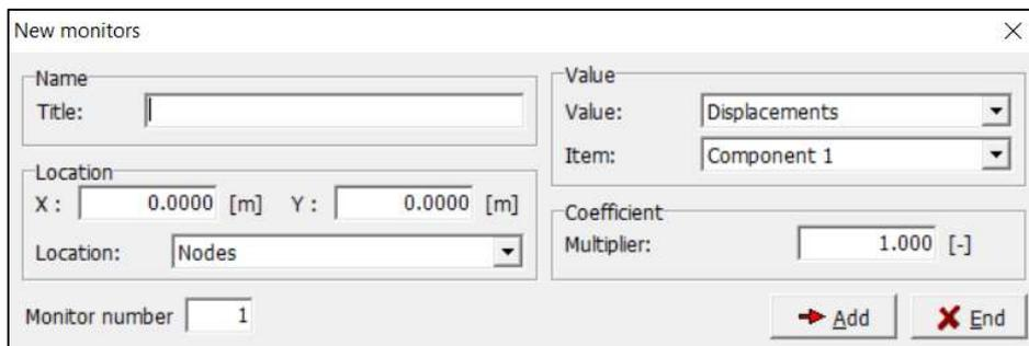
Figure 4.40: Definition of monitoring points through *Monitoring point tab*
