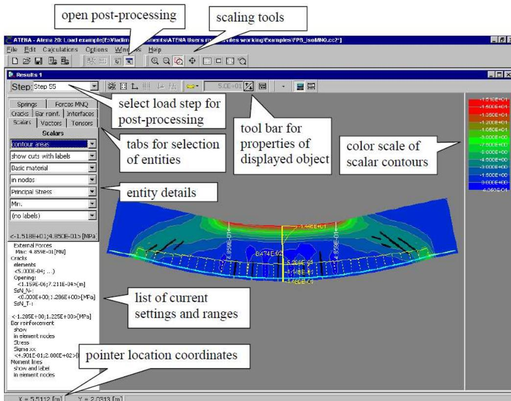
Figure 4.44: View of the post processing mode (User's Manual for ATENA2D [34])
