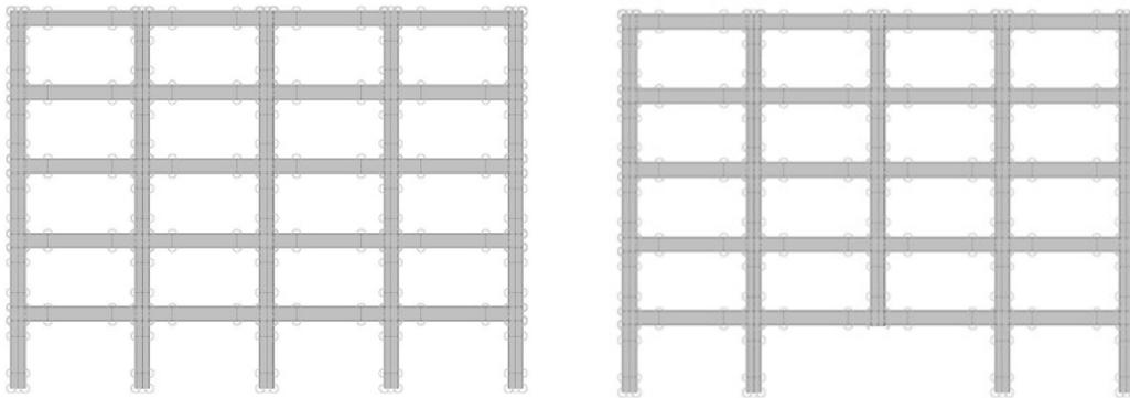
Figure 5.18: Representation of the 2D frame with joints, lines and macro-elements: in the left model with column, in the right, model without the column
