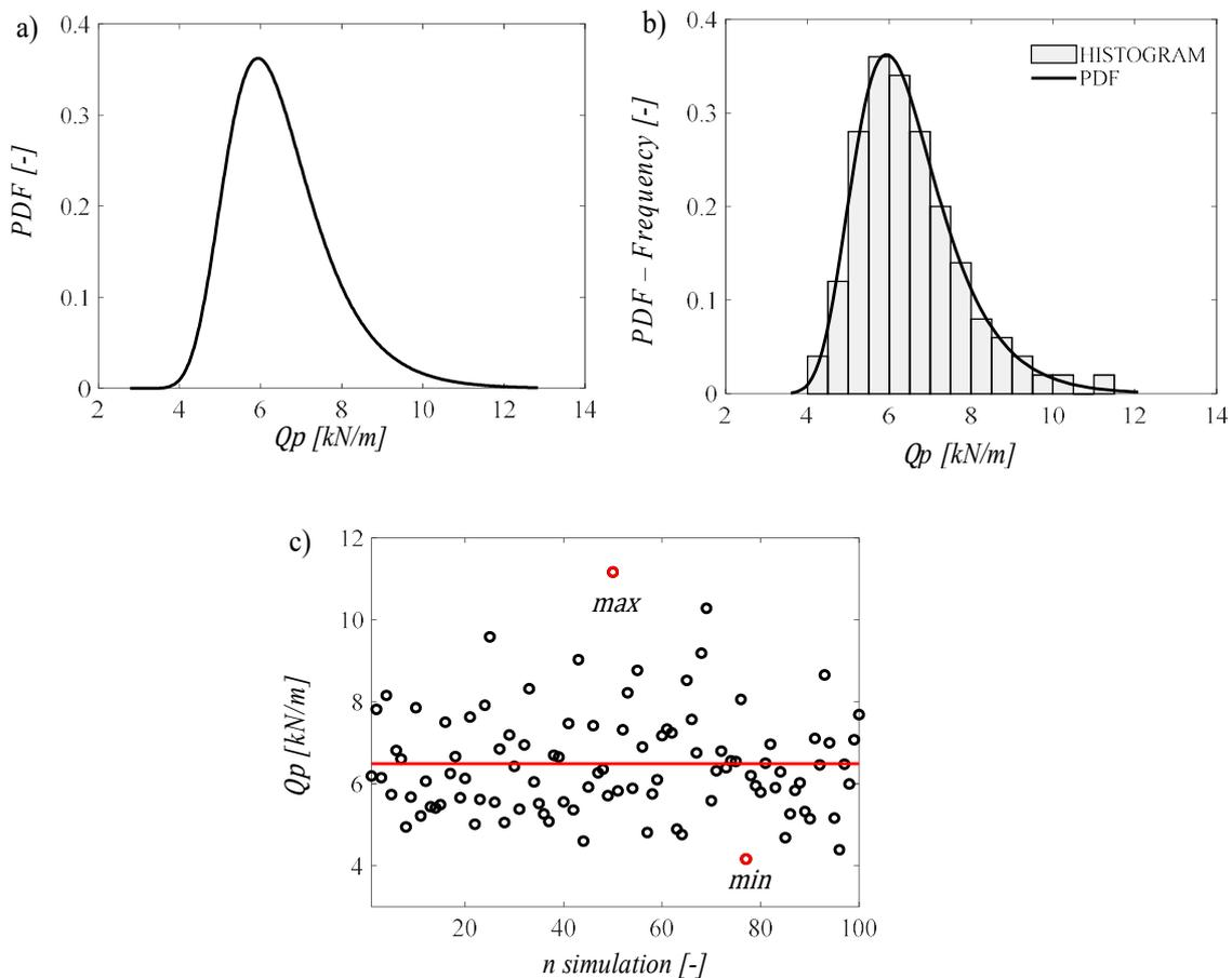
Figure 5.11: Floor variable load - Gumbel distribution: a) Probability density function; b) Histogram and Distribution fit; c) Scatter plot
