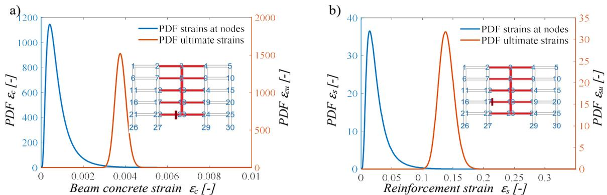
Figure 5.32: Convolution integral for the maximum  $P_f$  of directly affected sub-sections: a) beam confined concrete strain; b) beam reinforcement strain
