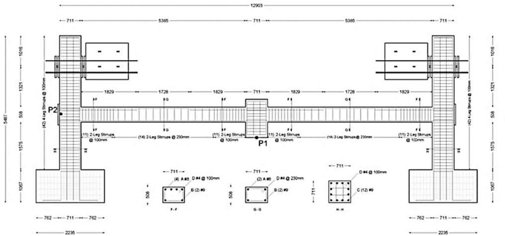
Figure 1.8: Two-dimensional reinforced concrete frame (Lew et al. [19])
