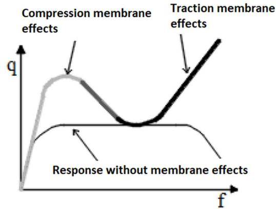
Figure 1.7: Load-displacement curve (CNR-DT 214 2018)
