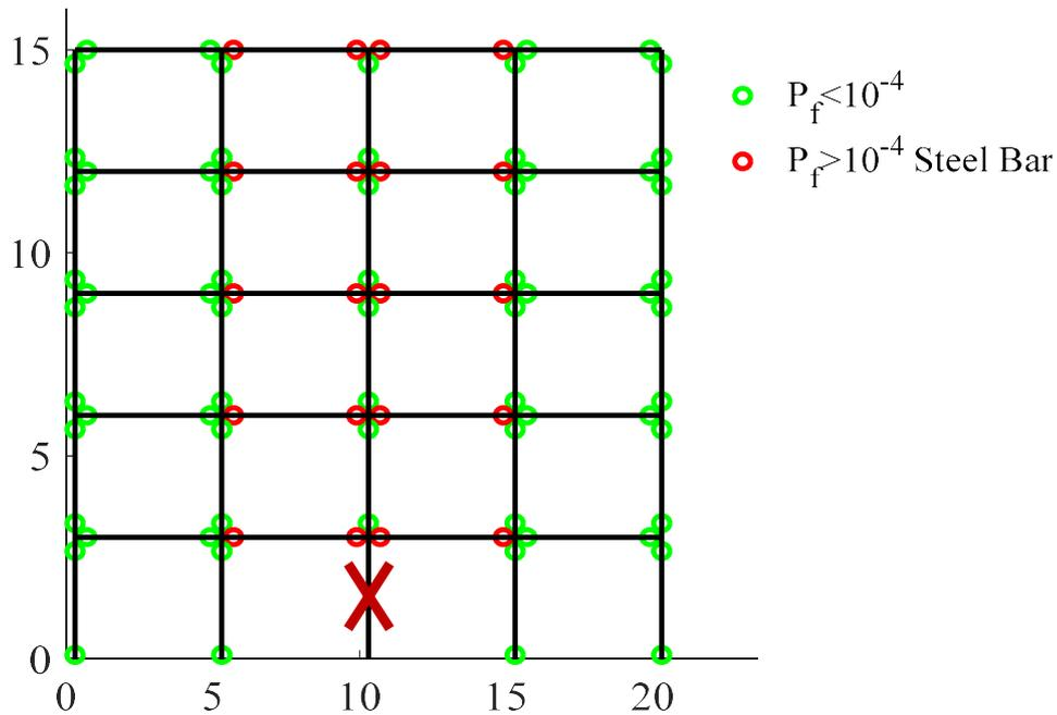
Figure 5.33: Scheme of the failure probabilities at each sub-section
