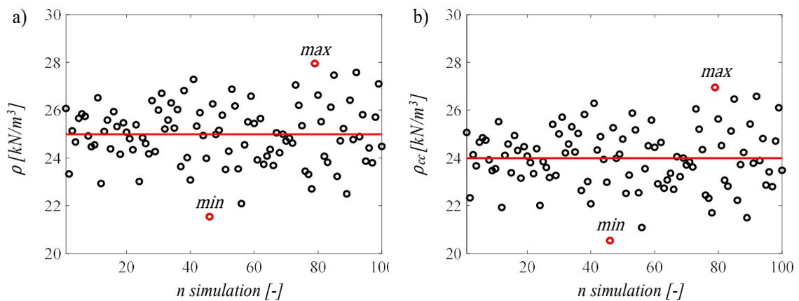
Figure 5.8: Scatterplots for specific weight: a) reinforced concrete (independent sampled variable); b) concrete cover (dependent variable)
