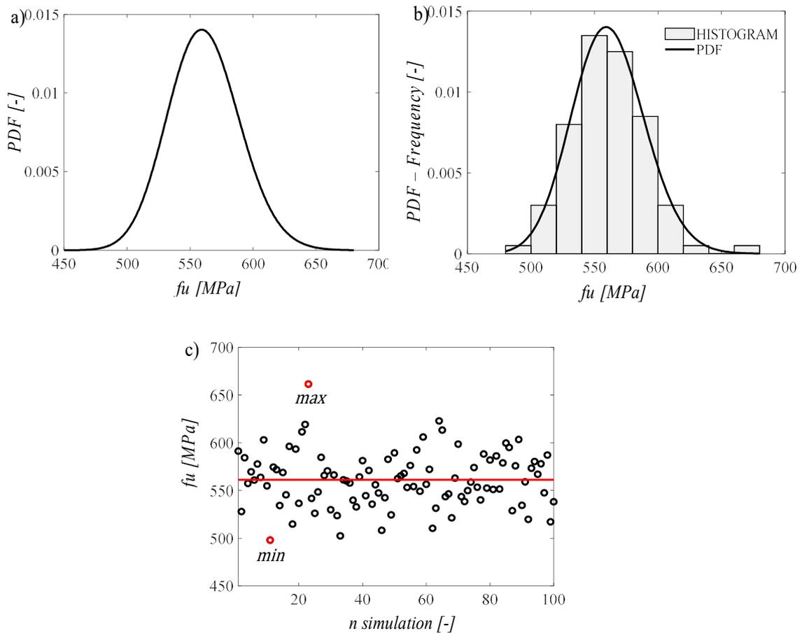
Figure 5.3: Steel ultimate strength - Lognormal distribution: a) Probability density function; b) Histogram and Distribution fit c) Scatter plot
