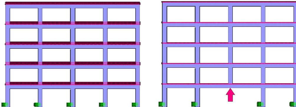
Figure 5.28: Frame modelled in ADINA Structures: on the left hand side model with the column; on the right hand side model without the column and reaction at the centre of the first floor
