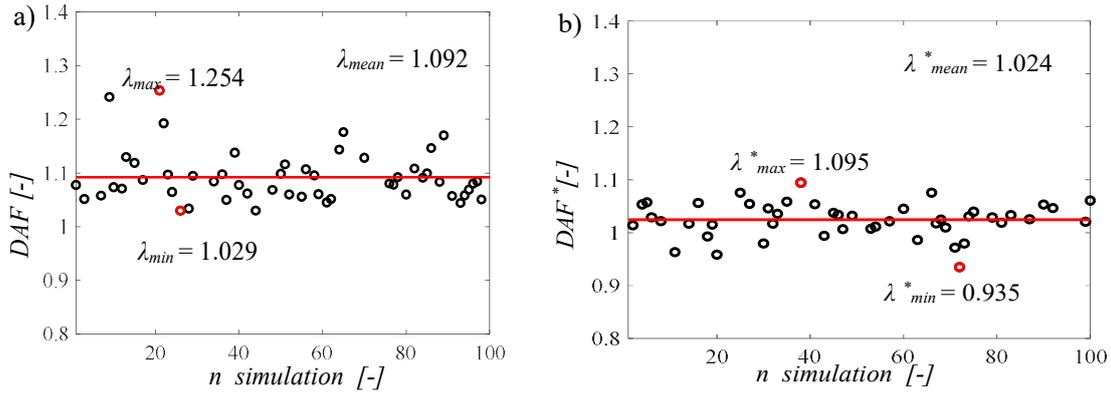
Figure 5.27: Dynamic Amplification factors for the  $N$  simulations: a) DAFs for the 53 simulations where equilibrium is reached; b) DAF\*s for the 47 simulations where equilibrium is not reached
