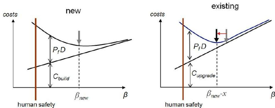
Figure 2.6: Target value identification: differences for the design of new structures versus upgrading of existing structures (fib Bulletin 80).
