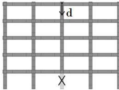
Figure 5.20: Scheme of the pushdown analysis
