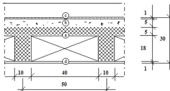
Figure 3.3: Slab scheme (dimensions in cm)
