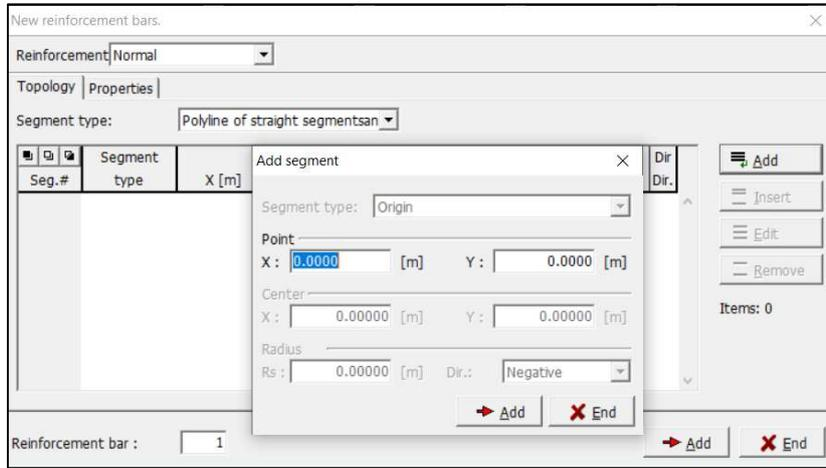
Figure 4.22: Reinforcement definition through *Reinforcement* tab (topology section)
