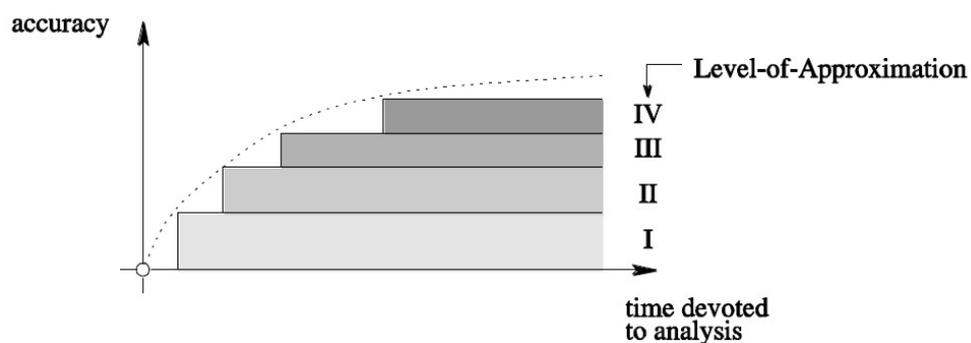
Figure 2.1: Accuracy on the estimate of the actual behaviour versus time devoted to the analysis for various LoA (fib MC 2010)
