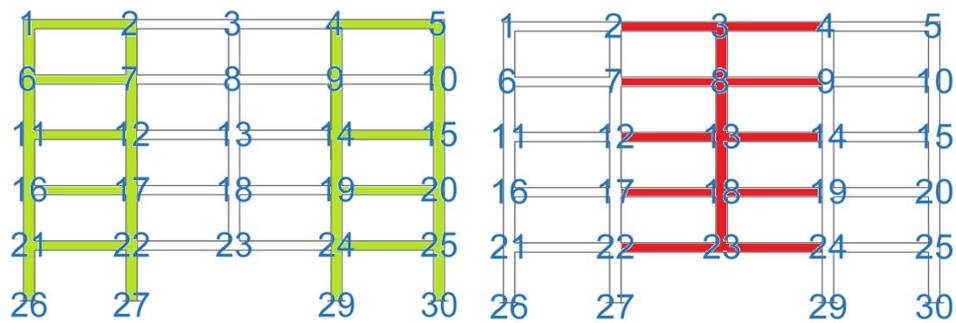
Figure 5.31: Scheme of the sections: a) directly affected members; b) indirectly affected members
