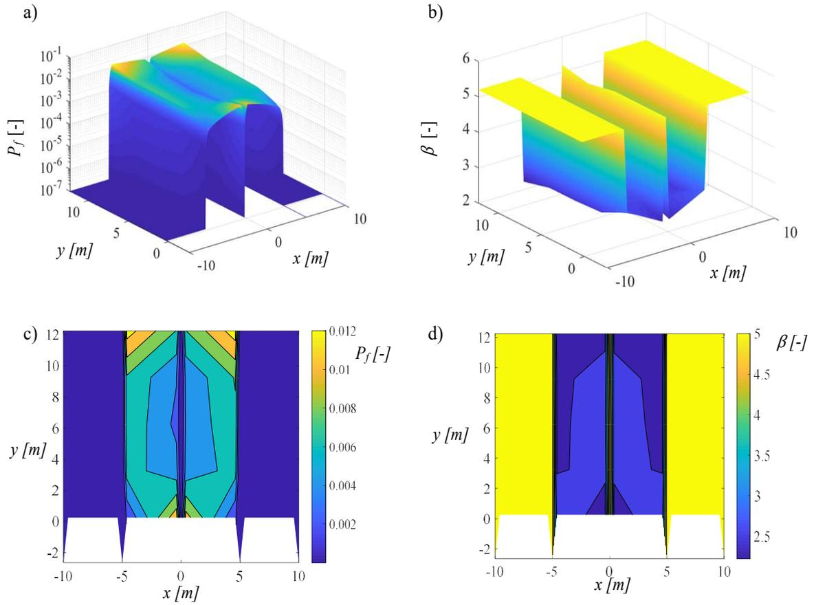
Figure 5.34: Failure probabilities and reliability indices of the nodes located at a distance  $(x, y)$  from the point where the column is removed: a) 3D plot of  $P_f$ ; b) 3D plot of  $\beta$ ; c) Contour plot of  $P_f$ ; d) Contour plot of  $\beta$
