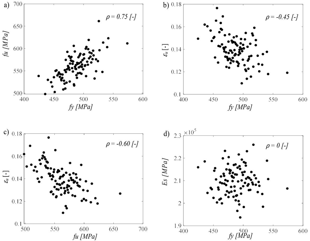
Figure 5.6: Correlation between reinforcement basic variables: a) correlation between  $f_y$  and  $f_u$ ; b) correlation between  $f_y$  and  $\epsilon_u$ ; c) correlation between  $f_u$  and  $\epsilon_u$ ; d) correlation between  $f_y$  and  $E_s$
