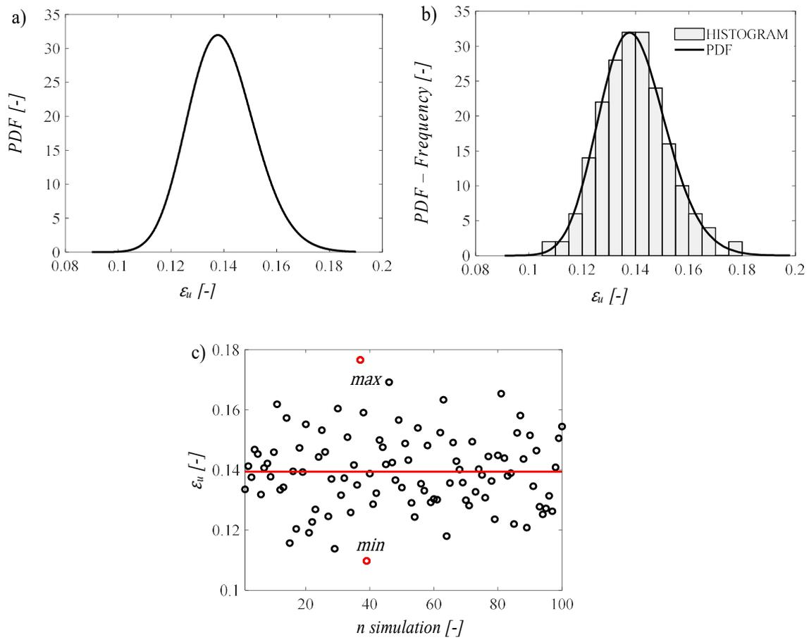
Figure 5.4: Steel ultimate strain - Lognormal distribution: a) Probability density function; b) Histogram and Distribution fit; c) Scatter plot
