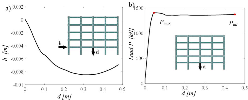
Figure 5.24: Pushdown analysis results for a generic simulation: a) vertical displacement of the central column vs horizontal displacement of the lateral column; b) vertical displacement of the central column vs load
