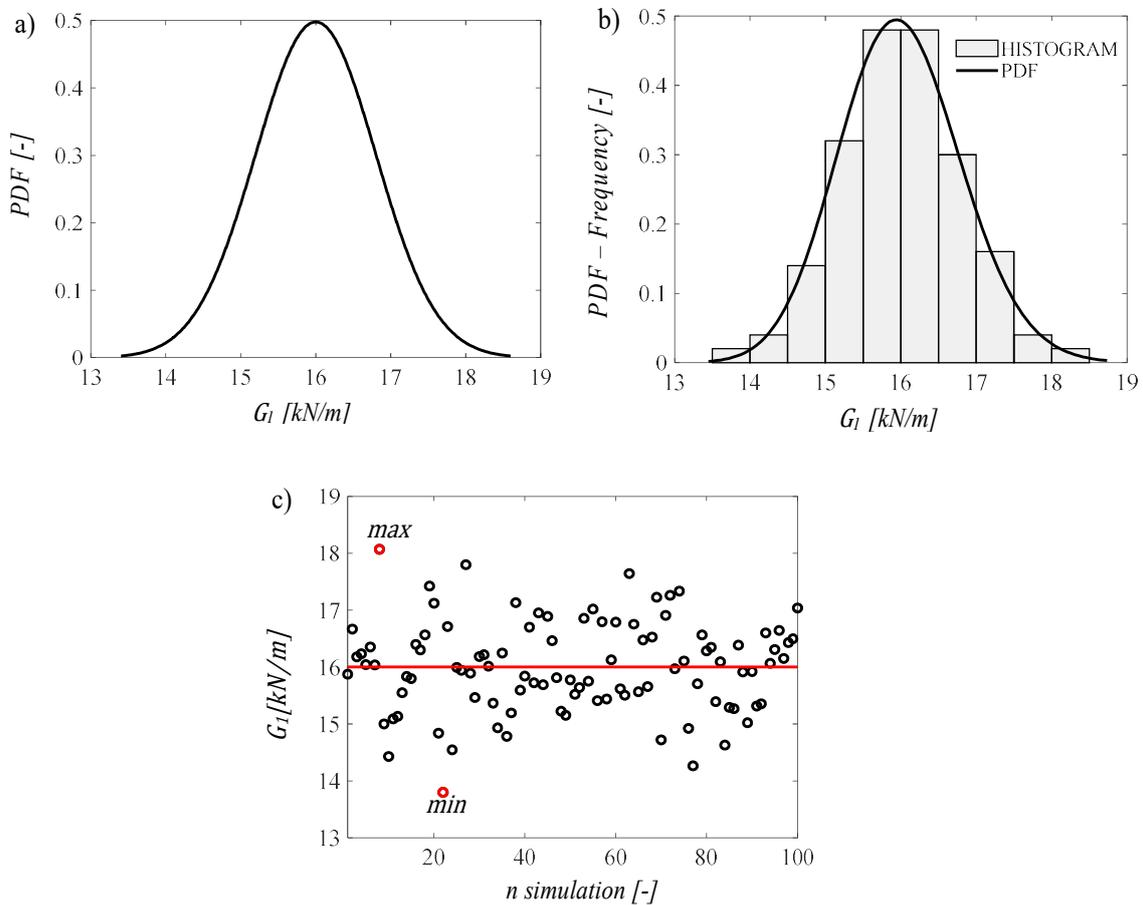
Figure 5.9: Permanent structural load - Normal distribution: a) Probability density function; b) Histogram and Distribution fit; c) Scatter plot
