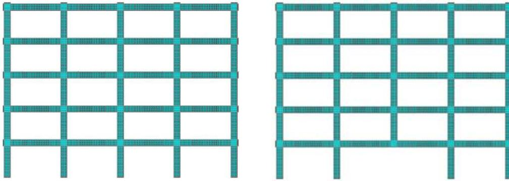
Figure 5.19: Representation of the 2D frame with longitudinal and transversal reinforcement: in the left model with column, in the right, model without the column
