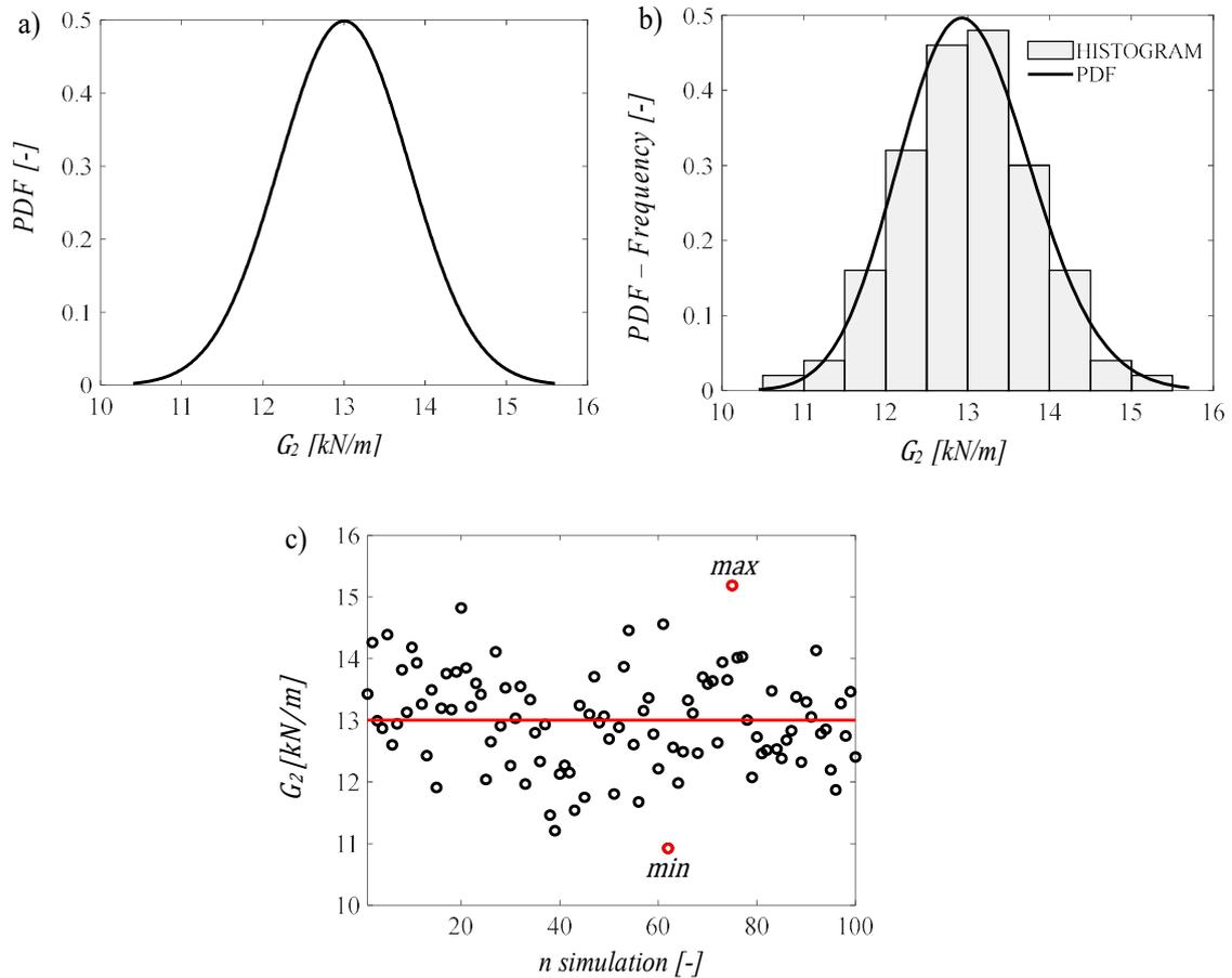
Figure 5.10: Permanent non-structural load - Normal distribution: a) Probability density function; b) Histogram and Distribution fit; c) Scatter plot
