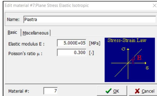
Figure 4.12: Basic tab for *Plane Stress Elastic Isotropic*
