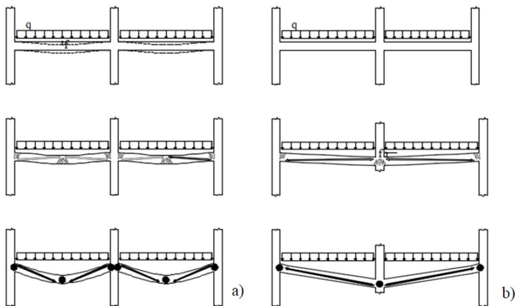
Figure 1.6: Membrane stresses (CNR-DT 214 2018)
