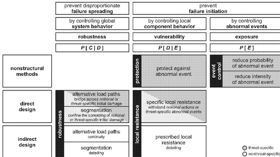
Figure 1.4: Methods for designing collapse-resistant structures (Haberland and Starossek 2009 [17])
