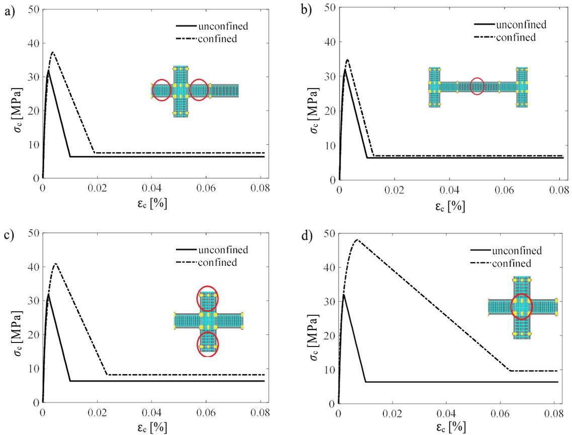
Figure 5.15: Stress-strain Relationship, unconfined vs confined concrete (Saatcioglu and Razvi [32]): a) beam dissipative area; b) beam non dissipative area; c) column; d) joints
