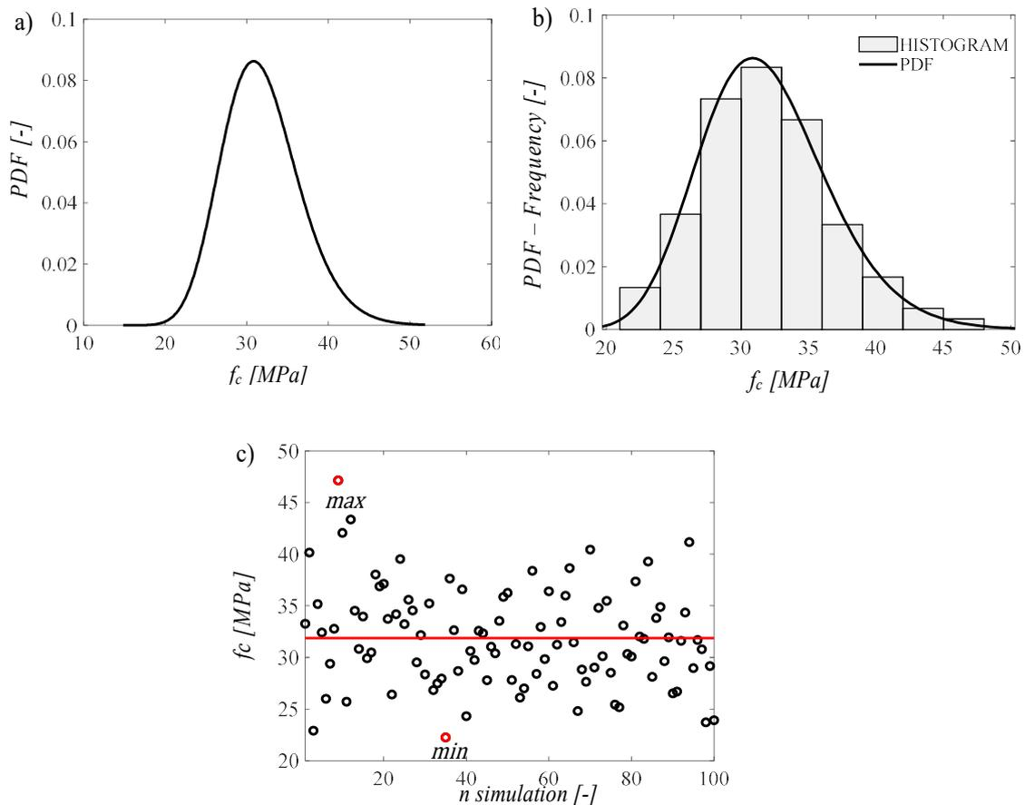
Figure 5.1: Concrete compressive strength - Lognormal distribution: a) Probability density function; b) Histogram and Distribution fit; c) Scatter plot
