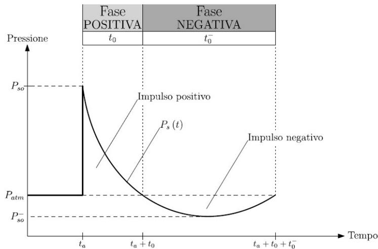
Figure 1.1: Temporal behaviour of the front wave (CNR-DT 214/2018)
