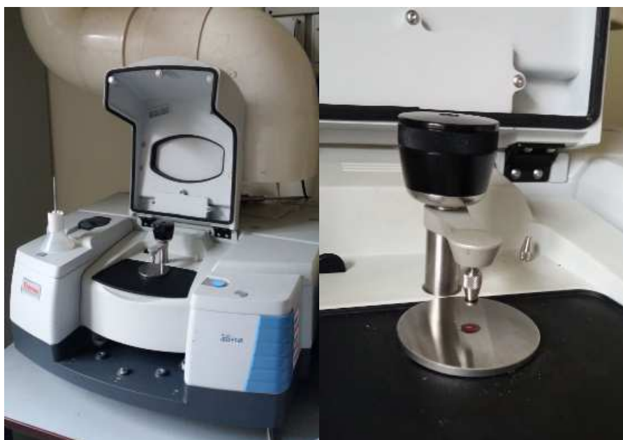
Figure 4.10 FTIR instrument – a zoom on ATR accessory
