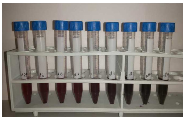
Figure 5.12 Buffered functionalising solutions (TRIS/HCl+CaCl 2 +PPHE) to be characterised through zeta potential
