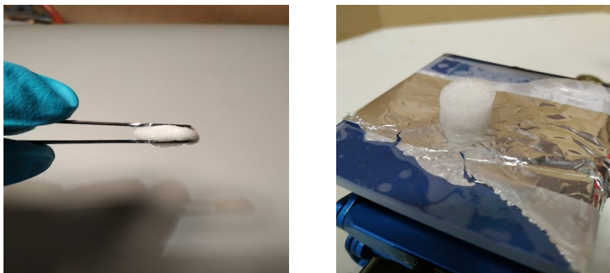
Figure 3.6: compressed state (left), impregnated foam (right)
