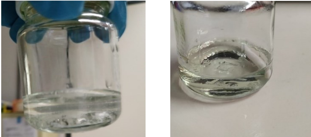
Figure 3.5: formulation before (left) and after (right) stirring at 40°C
