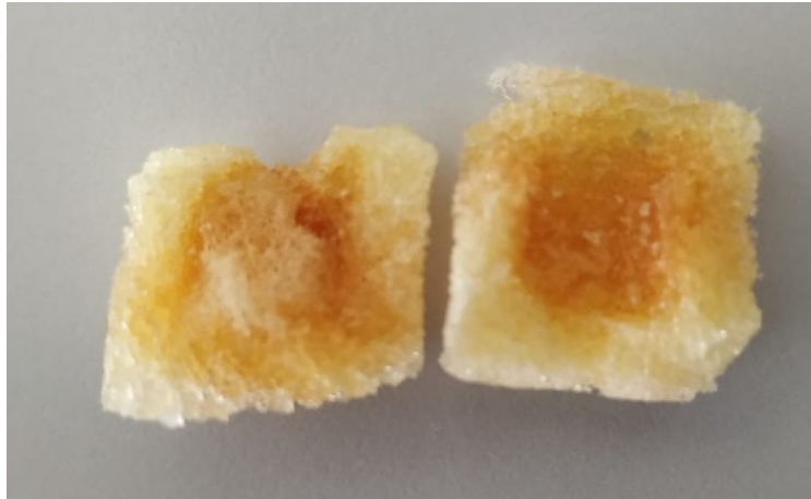
Figure 4.12: uncured foam parts present into the sample for formulation 5.
