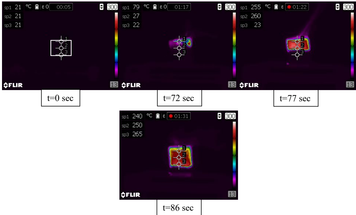
Figure 4.2: IR thermal images related to formulation 5. (IOC8 SbF6=0,5%wt, TPED=0,5%wt) At 40mW/cm 2
