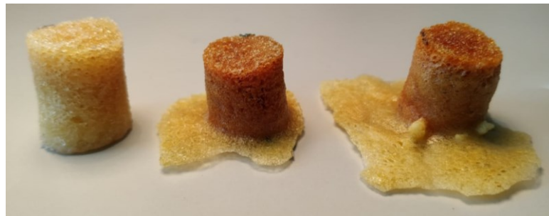
Figure 4.10: external resin flow due to high heating rate. Composition 5. (left), composition 8. (centre), composition 9. (right)
