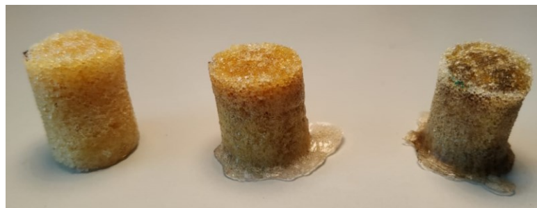
Figure 4.11: black colour and resin outflow present in formulation 5. (left), 6. (centre) and 7. (right)
