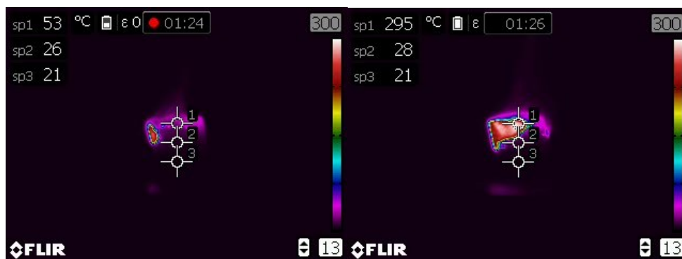
Figure 4.5: example of the delaying of the starting point (2 seconds) formulation 6. At 40mW/cm 2
