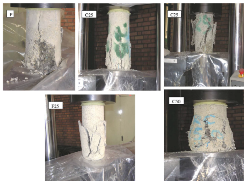
Figure 25: Failure types of specimens
