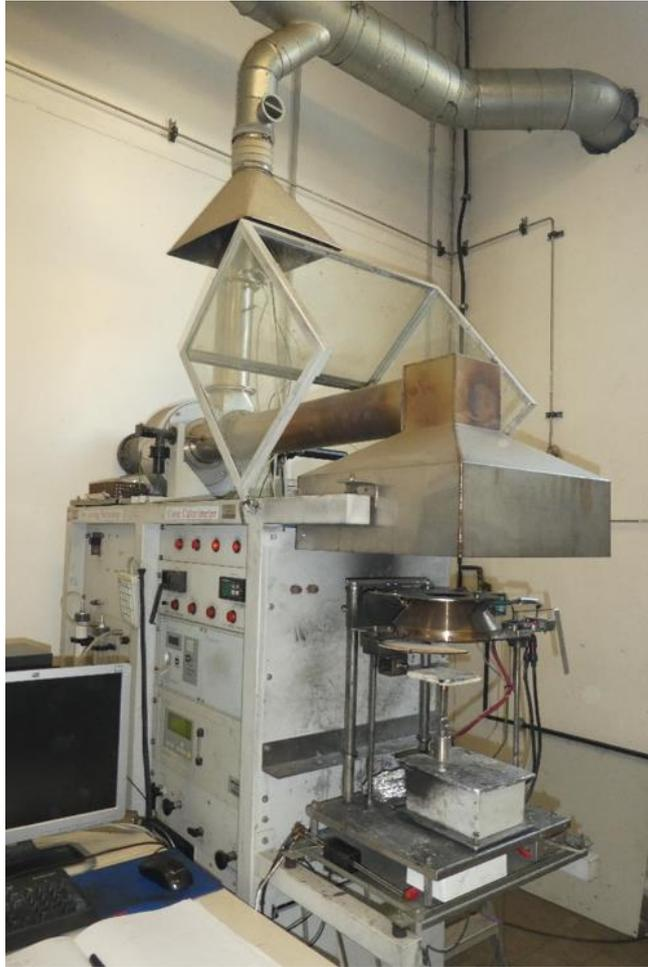
**Figura 2.14** – Cono calorimetro Fire Testing Technology Limited (FTT).
