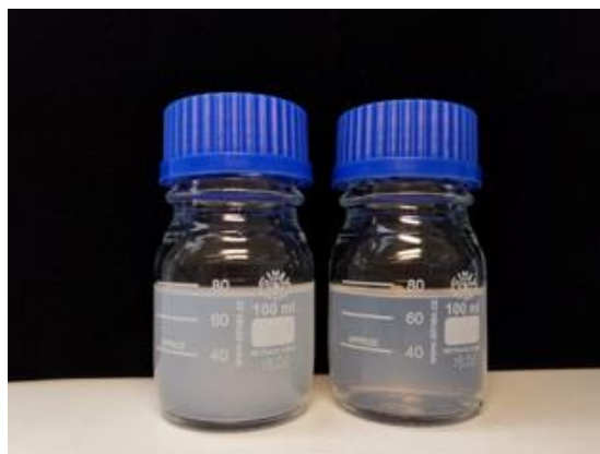
Figure 13. From the left: non-sonicated CNC stock dispersion, sonicated CNC stock dispersion.
