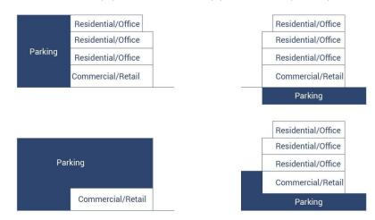
Figure 3.11 - Methods to incorporate parking to buildings Source: Author's elaboration
