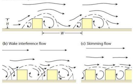
Figure 4.5 a), b), c) - Wind flows behaviors according to different H/W ratios Source: (Oke, Mills, Christen, & Voogt, 2017, p. 88)
