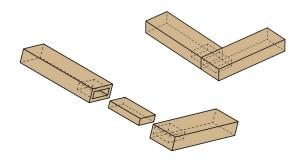
Figure 17-B:The list of several common structures of mortise and tenon
