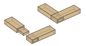
Figure 17-A: The list of several common structures of mortise and tenon
