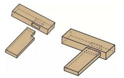
Figure 17-F. The list of several common structures of mortise and tenon
