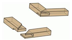
Figure 17-E.The list of several common structures of mortise and tenon
