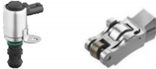
Figure 5.16: Deactivation Control Valve (left) and Deactivation Roller Finger Follower (right) [17]
