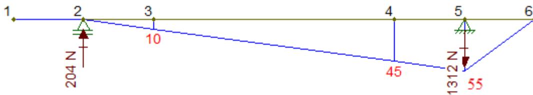
Figure 6.26: Bending moment diagram – YX plane
