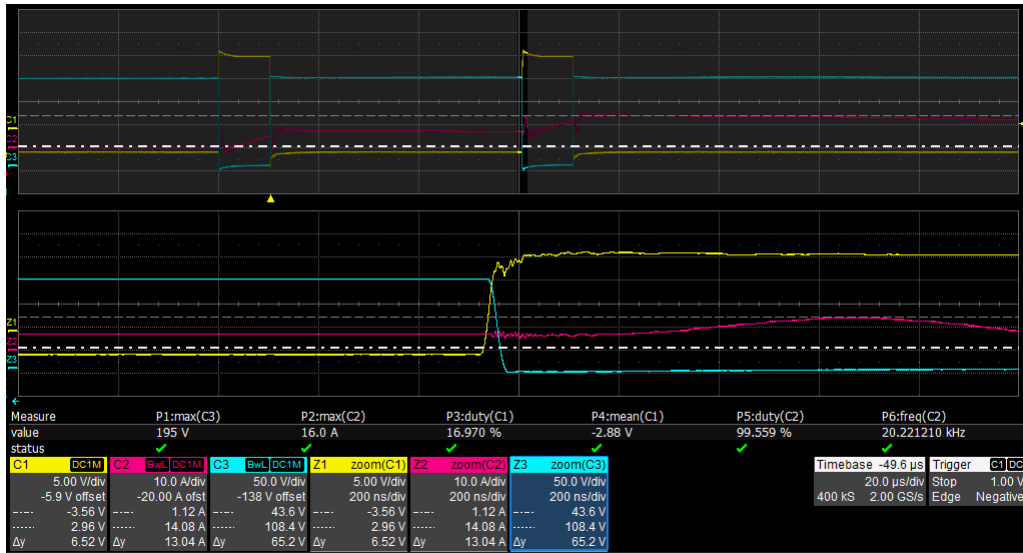
Figure 6.24. Prototype connected to a DC-bus of 200V and driven with two pulses of 10μs distanced by 50μs. Zoom of the start-up with output current different from zero.
