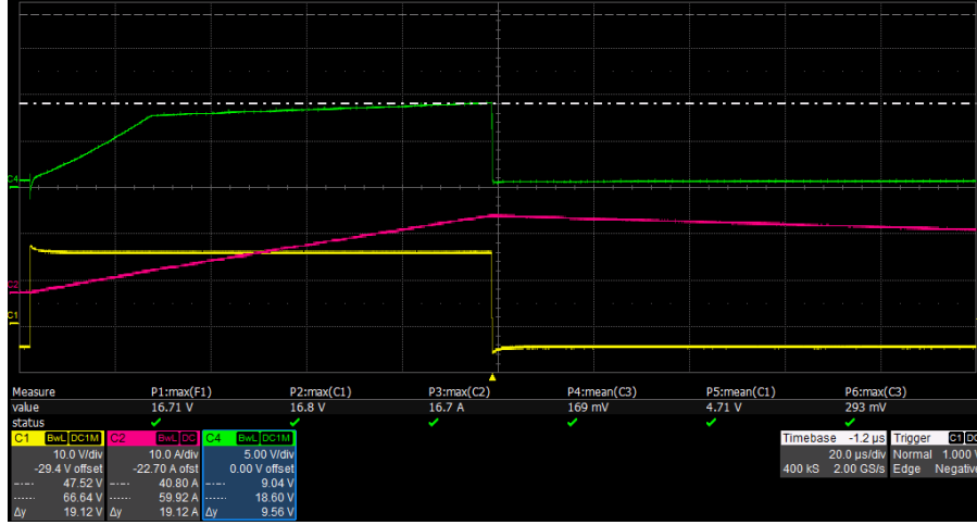
Figure 6.31. Prototype connected to a DC-bus of 200V. The waveform reported are: gate of the low-side transistor (yellow), DESAT pin (green), output current (red).
