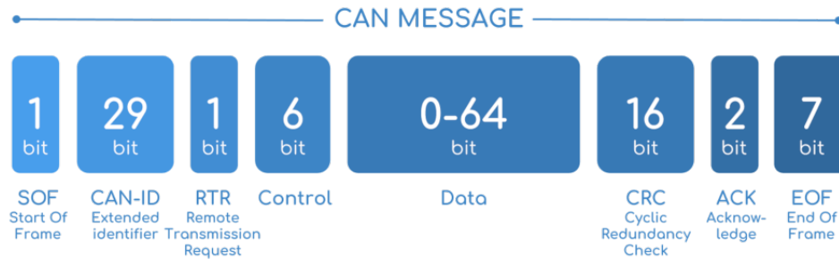
Figure 3.9: CAN bus message data structure
