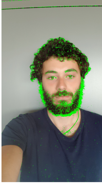
Figure 2.21: Harris detector output image
