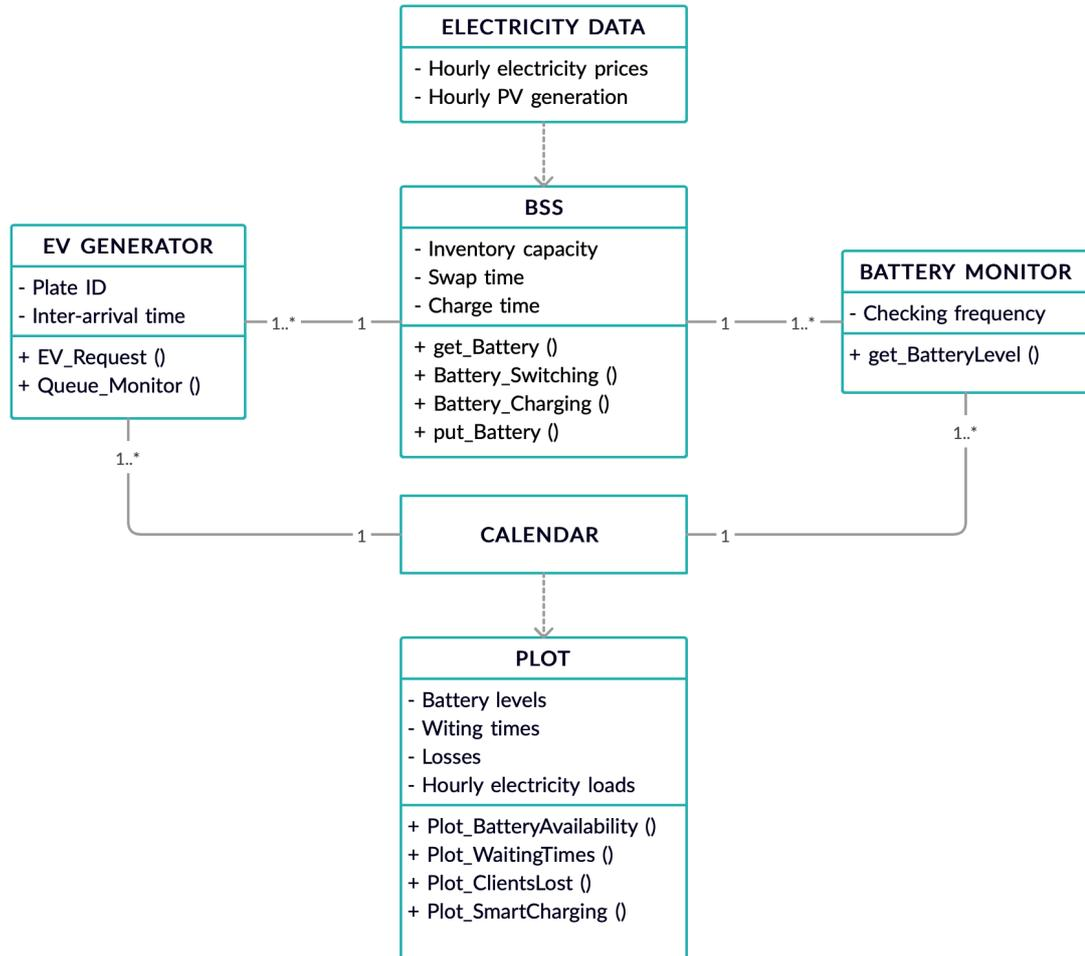
Figure 3.1. Class Diagram of the BSS Simulator Architecture.
