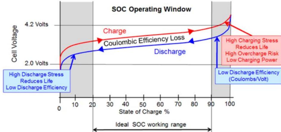
Figure 2.2. Recommended operating range of SoC for lithium-ion batteries [35][66]
