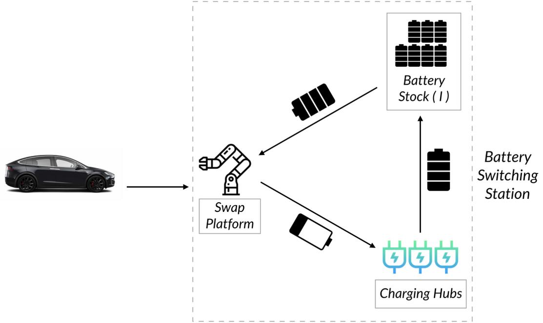
Figure 2.3. Operation of the Battery Switching Station Model.
