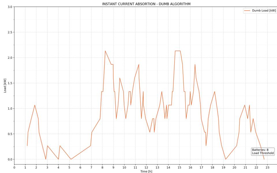
Figure 3.2. Instant Current Absorption without Smart-Charging Algorithm.
