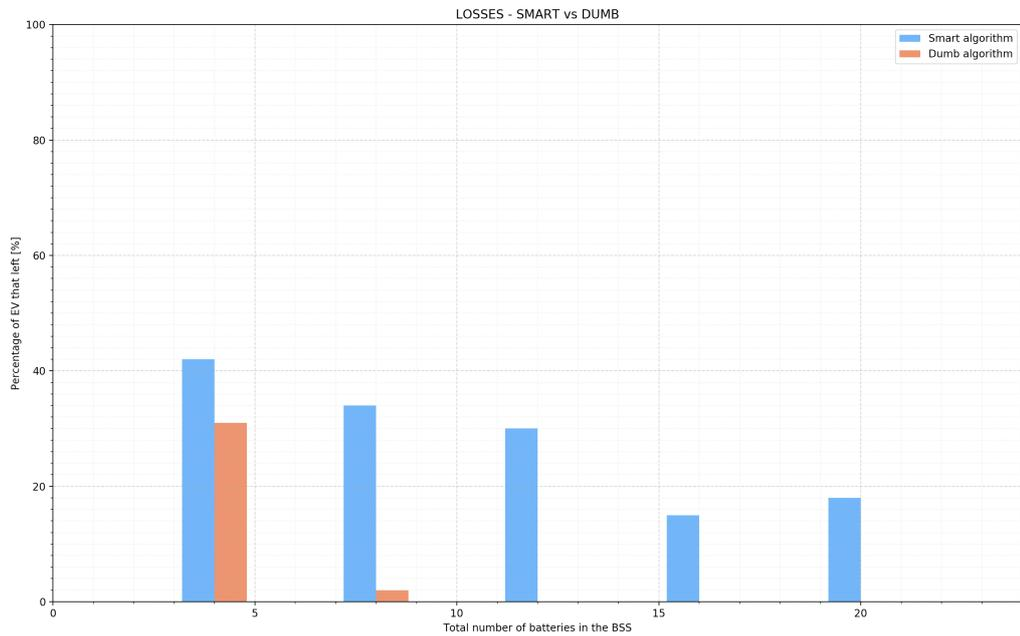
Figure 3.6. Client (EVs) losses - Comparison of BSS with 4, 8, 12, 16 and 20 batteries in stock.
