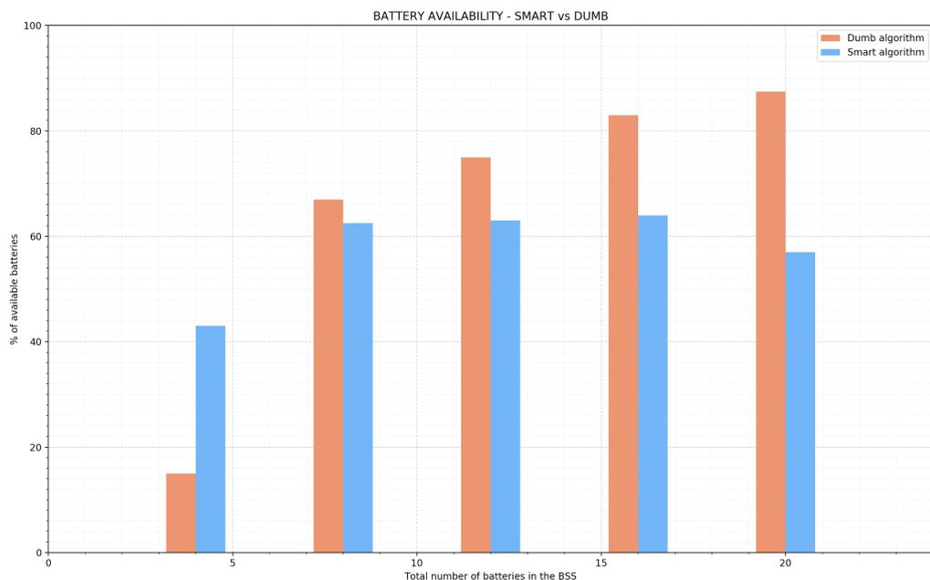
Figure 3.8. Probability of finding an available battery - Comparison of BSS with 4, 8, 12, 16 and 20 batteries in stock (QoS constraint).
