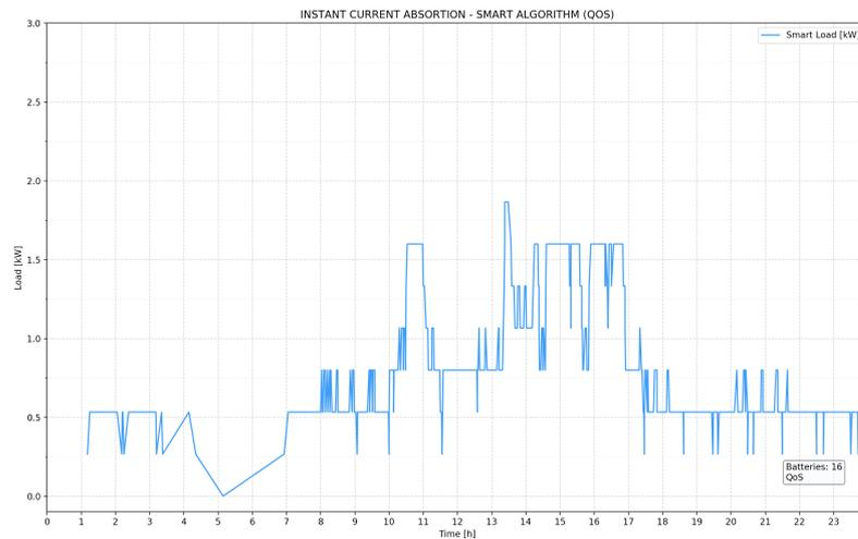
Figure 3.12. Instant Current Absorption with Smart-Charge Algorithm and QoS constraint.
