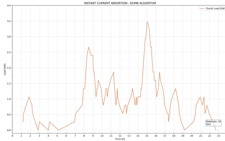
Figure 3.11. Instant Current Absorption without Smart-Charging.
