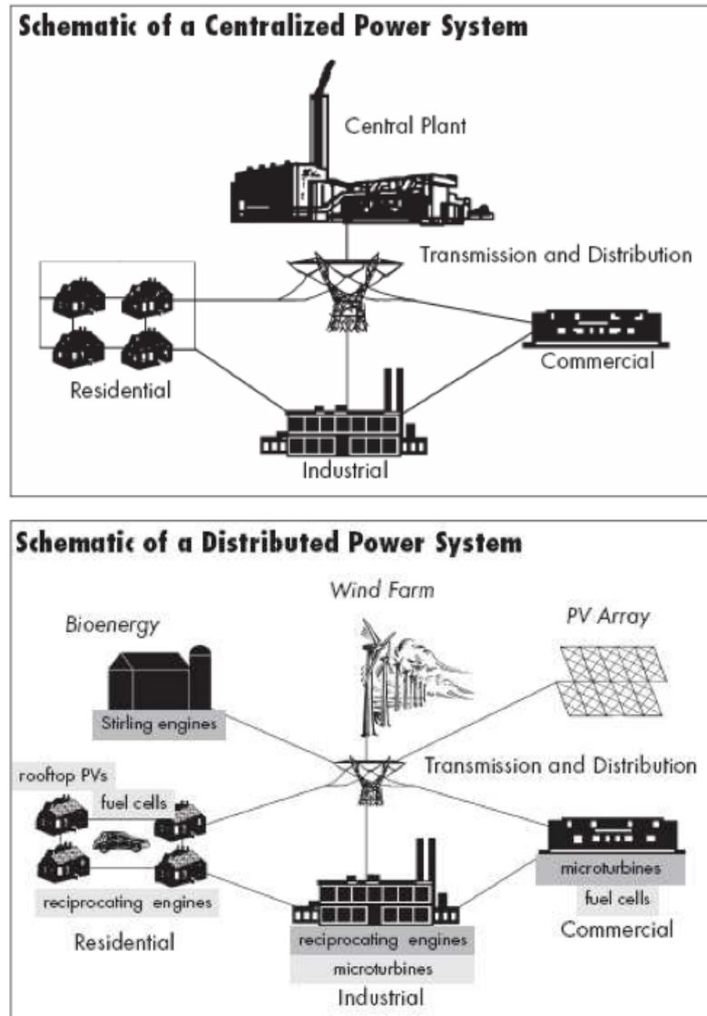
Figure 1.3. From centralised to distributed power system.
