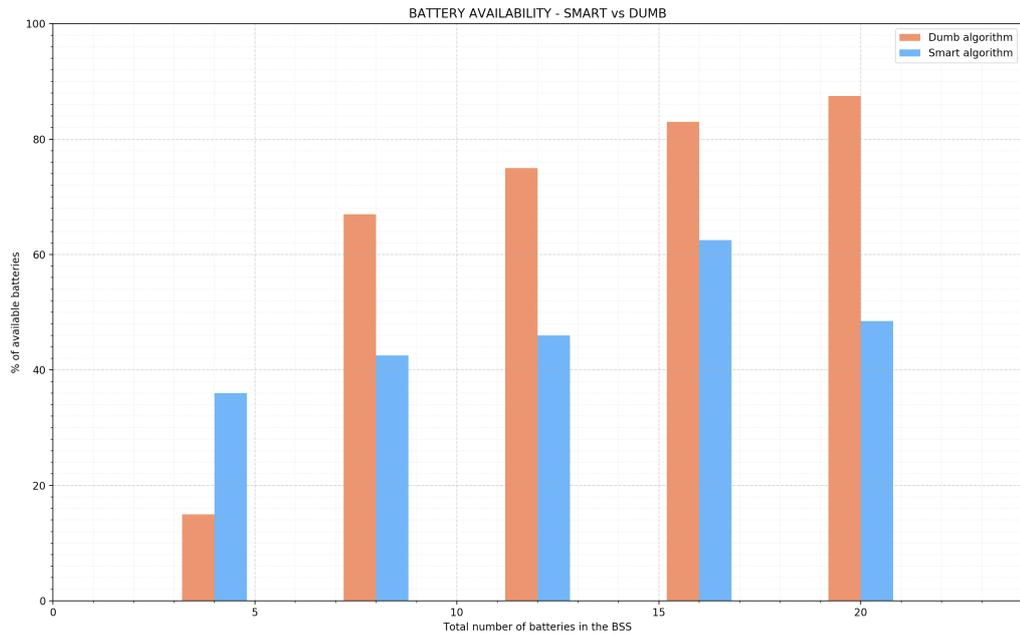
Figure 3.5. Probability of finding an available battery - Comparison of BSS with 4, 8, 12, 16 and 20 batteries in stock.
