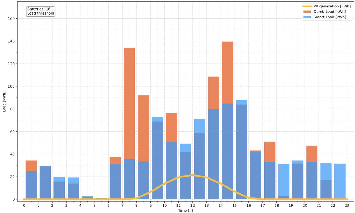
Figure 3.13. Hourly Current Absorption - Smart-Charge Algorithm with QoS constraint.
