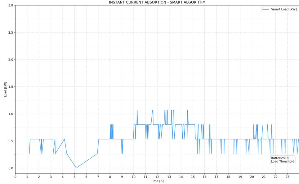
Figure 3.3. Instant Current Absorption after the application of the Smart-Charging Algorithm.
