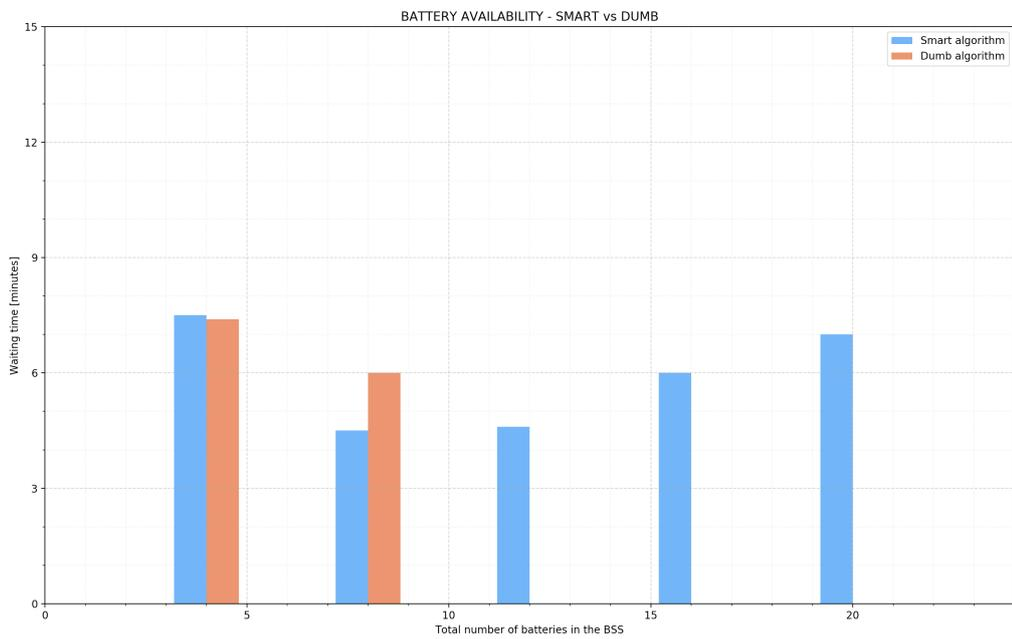
Figure 3.10. Client (EVs) losses - Comparison of BSS with 4, 8, 12, 16 and 20 batteries in stock.
