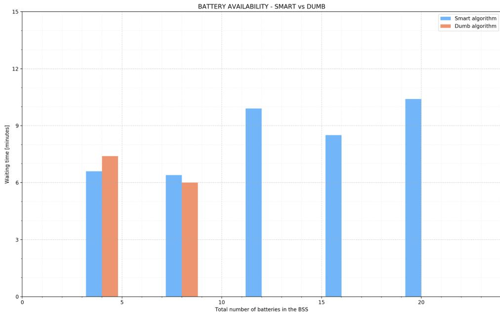
Figure 3.7. Average waiting times of EVs that wait to receive service - Comparison of BSS with 4, 8, 12, 16 and 20 batteries in stock.
