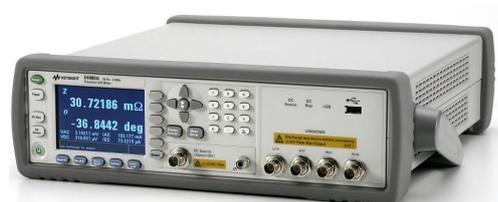
**(b)** LCR E4980A by Agilent used for impedance measurements of coil and electrodes.
