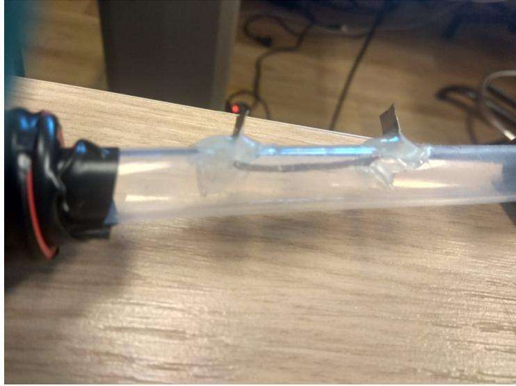
**Figure 29:** Electrode in the tube fixed with hot glue to avoid motion and fluid losses.
