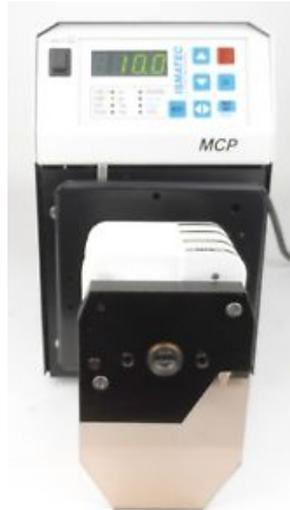
*Figure 27: Peristaltic pump needed to force the fluid motion.*
