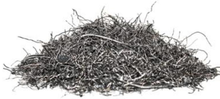
*Figure 5 Recycled steel fibres from End-of-Life tyres*
