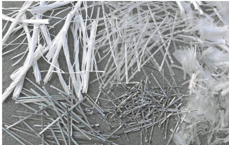
*Figure 2 Examples of fibres' materials*
