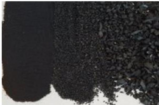
*Figure 4 Recycled rubber in various sizes*
