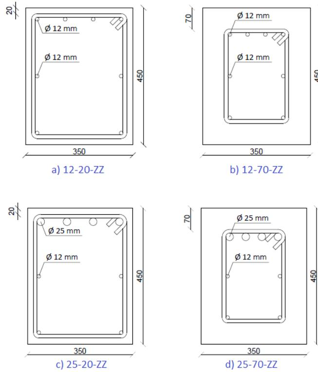
Figure 22 Cross-sections of the analysed beams (dimensions in mm); ZZ is the fibre content: 0%, 0.5% or 1.0%
