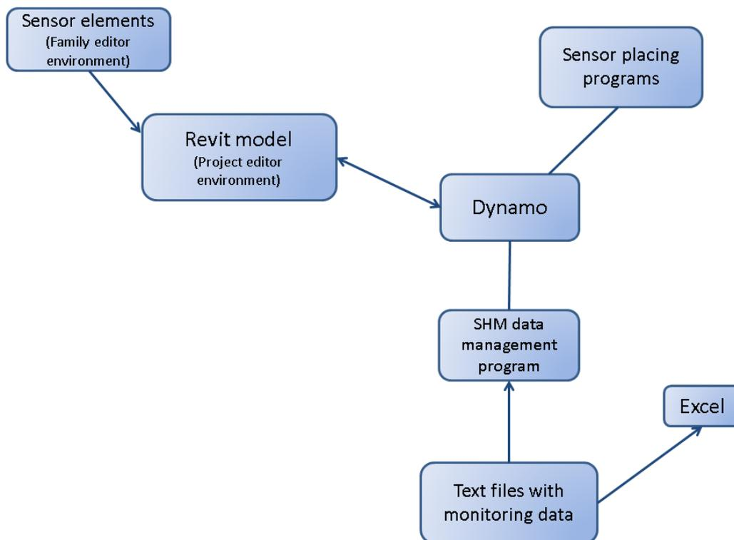
Figure 30: Work methodology scheme. Stura Bridge.
