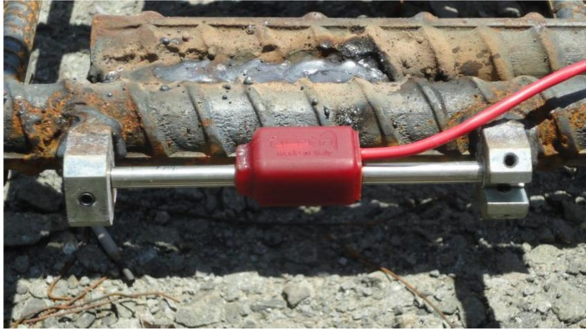
Figure 4: VW strain sensor.
