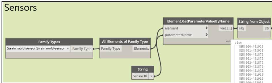
Figure 61: Bridge SHM data modelling. Sensors selection.
