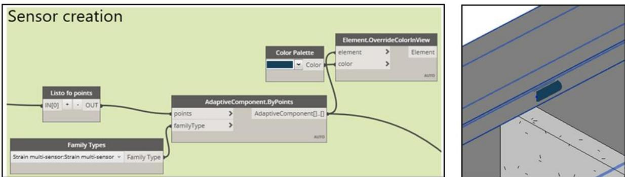
Figure 46: Bridge SHM strain multi-sensor placing. Sensors creation.
