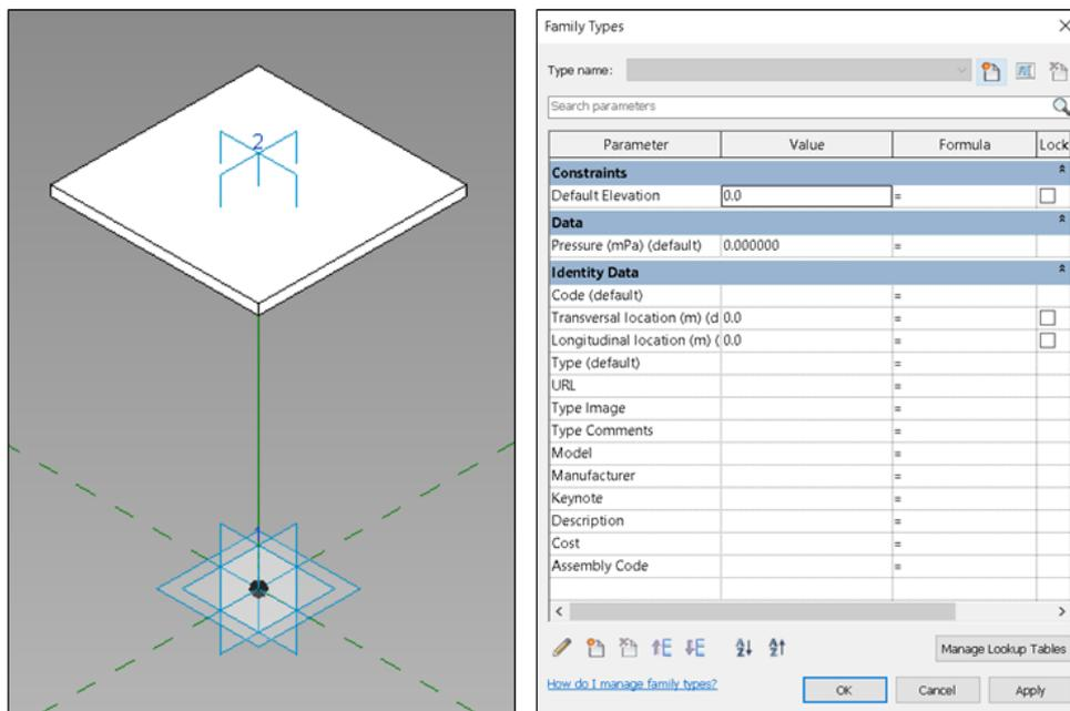
Figure 98: Pressure cell family creation. Left: shape. Right: parameters.
