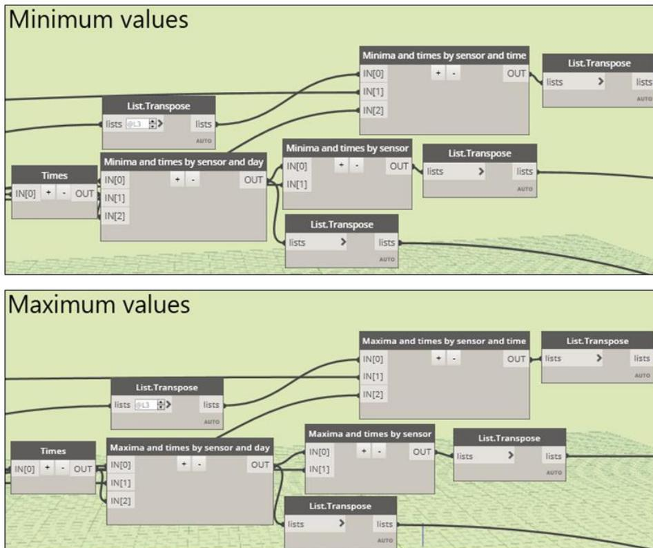
Figure 77: Bridge SHM data management. Maximum and minimum measurements.
