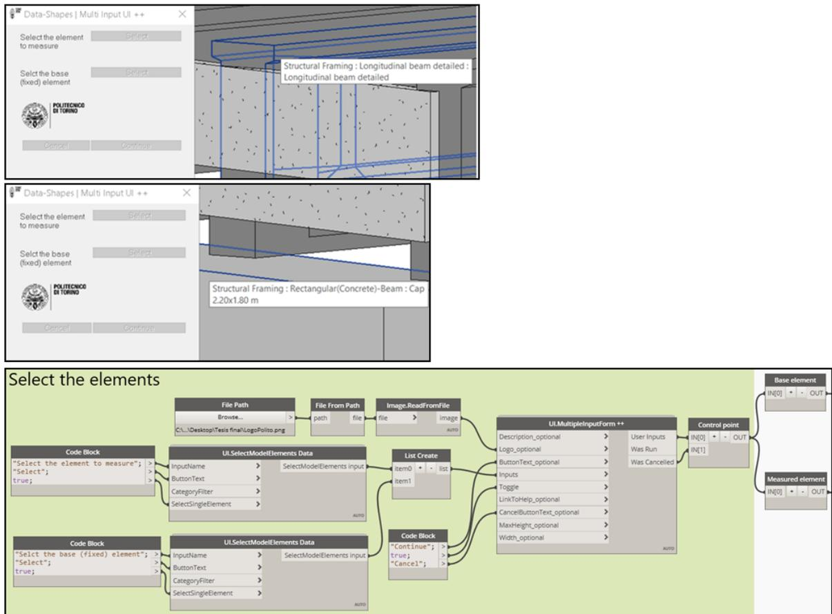
Figure 56: Bridge SHM displacement multi-sensor placing. Selection of the elements.
