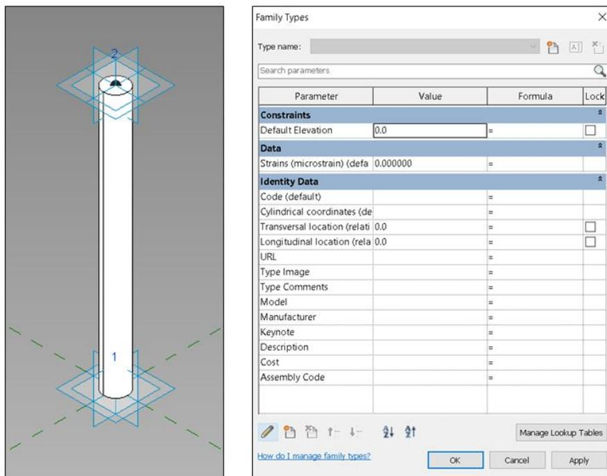
Figure 97: Extensometers family creation. Left: shape. Right: parameters.
