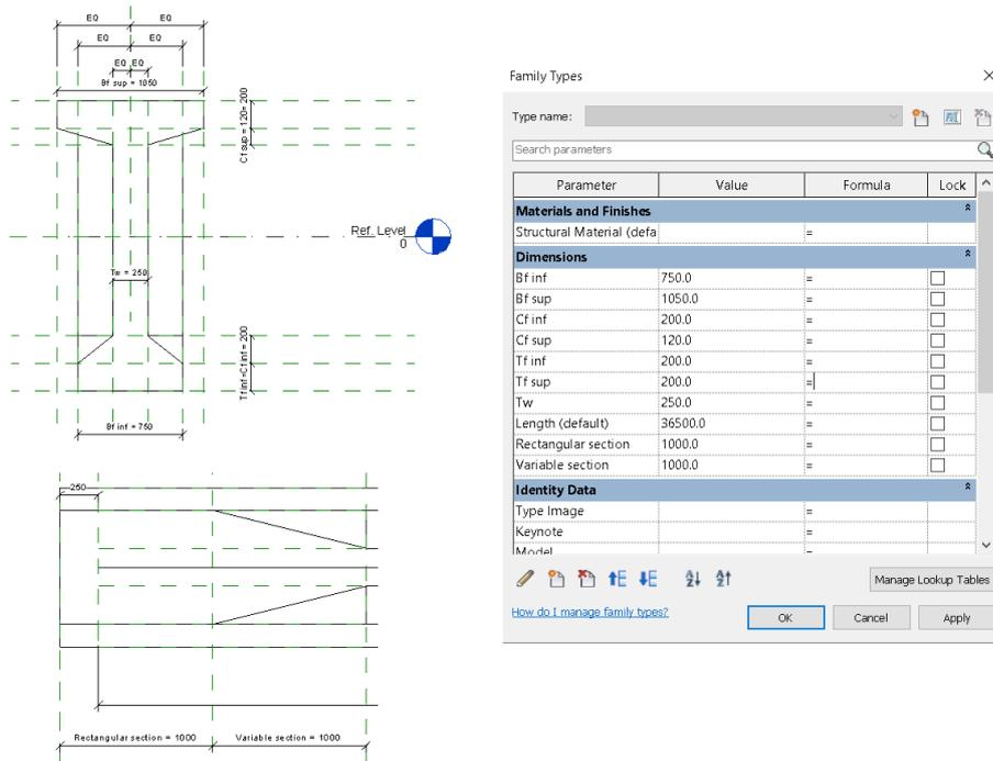
Figure 34: Longitudinal beams family. Stura Bridge.
