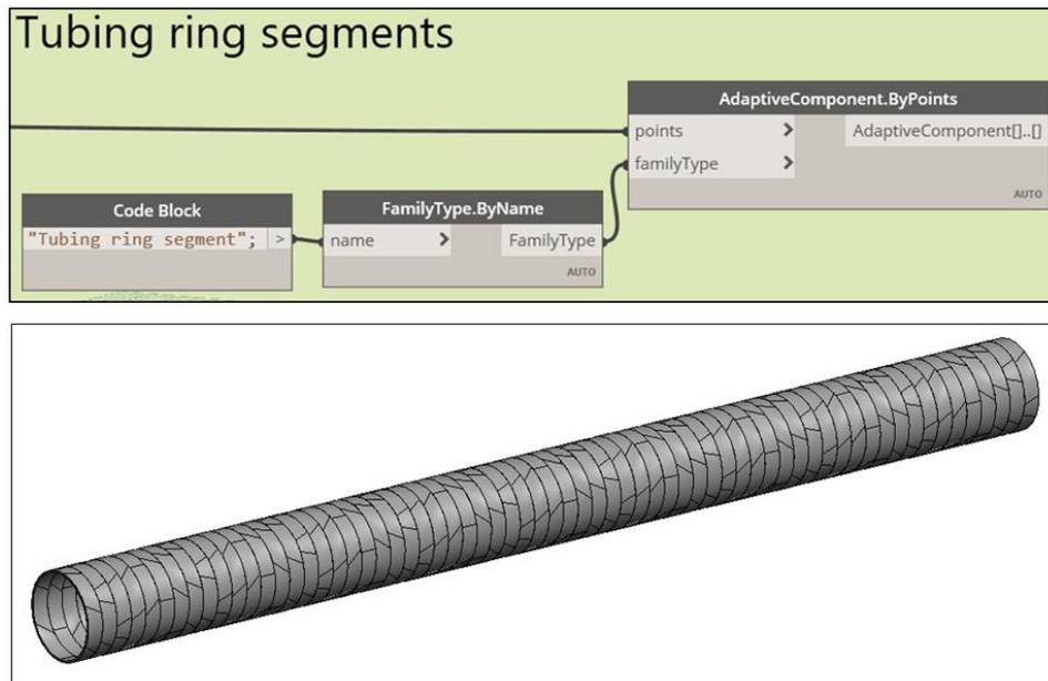
Figure 89: Tunnel creation program. Tubing ring segments placing.
