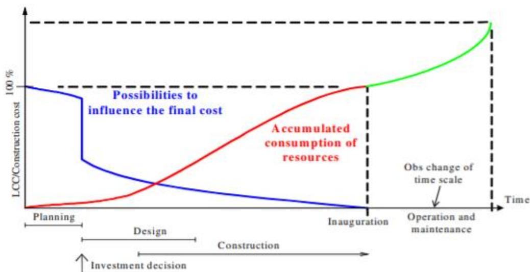
Figure 9: Impact of stages in the final construction cost.
