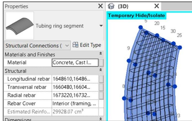
Figure 95: Tunnel reinforcement. Tubing ring segments reinforcement parameters.
