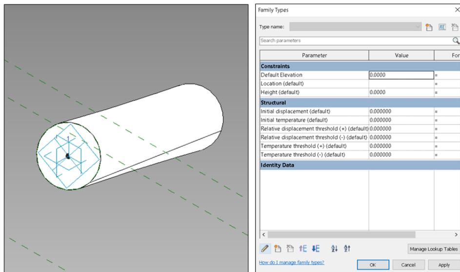
Figure 38: Displacement multi-sensor family. Adaptive comp. shape and parameters.
