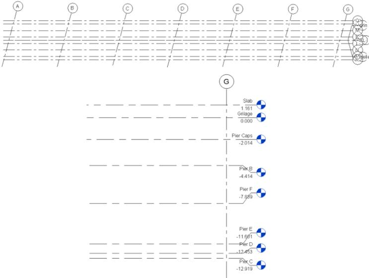
Figure 32: Axes (above) and levels (below) of the model.
