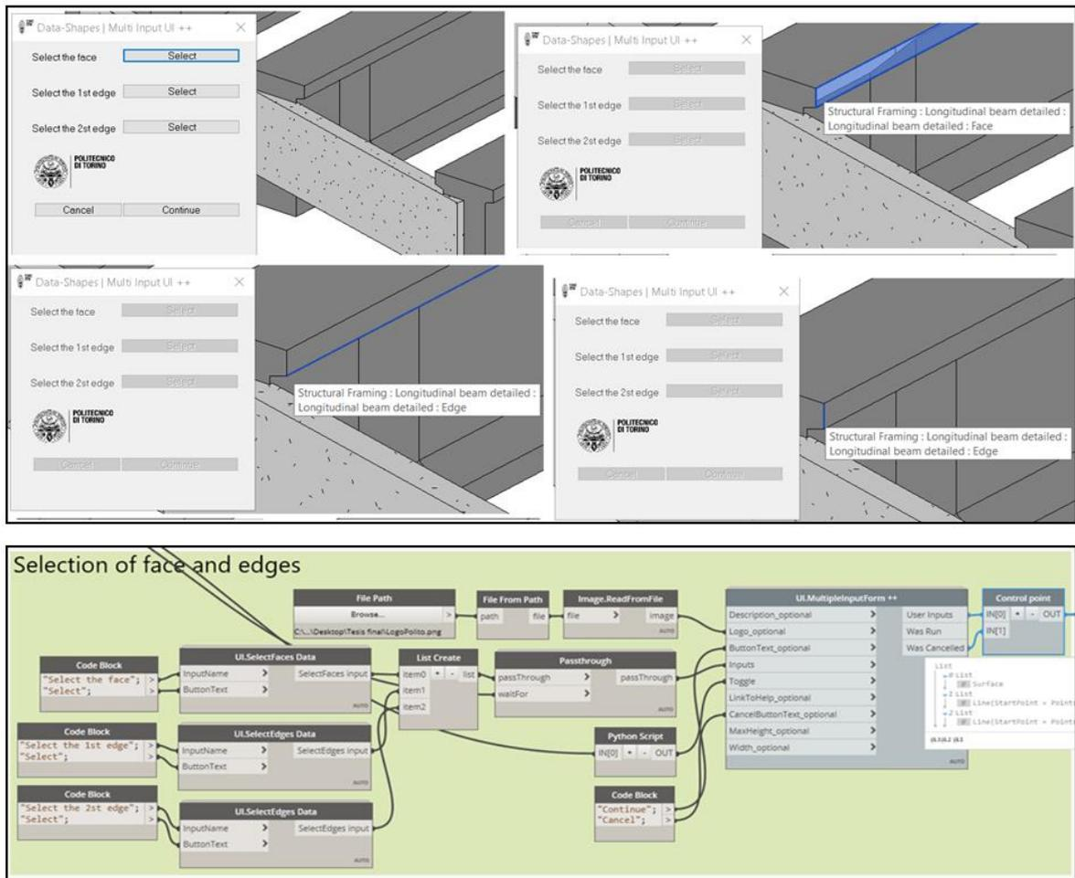
Figure 40: Bridge SHM strain multi-sensor placing. Face and edges selection.
