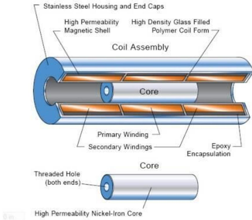
Figure 5: LVDT sensor. Scheme.
