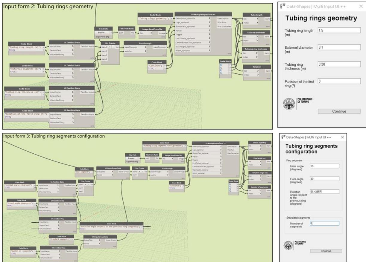
Figure 87: Tunnel creation program. Geometrical inputs.
