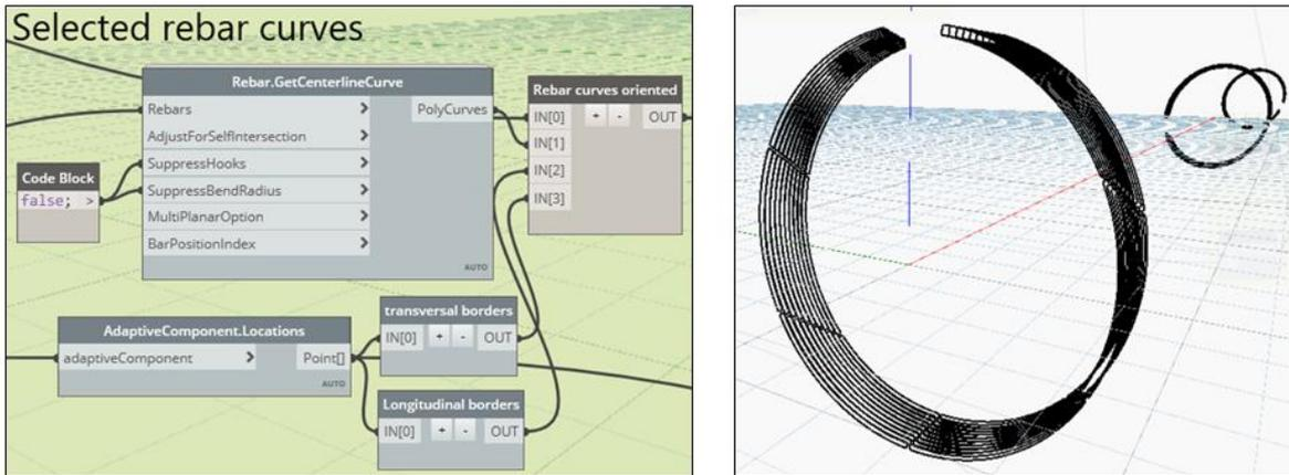
Figure 112: Tunnel SHM smart-sensors program. Rebar curves extraction.
