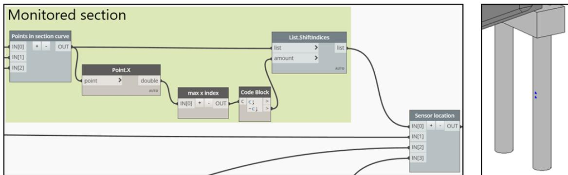
Figure 53: Bridge SHM strain multi-sensor placing. Creation of the placing points.
