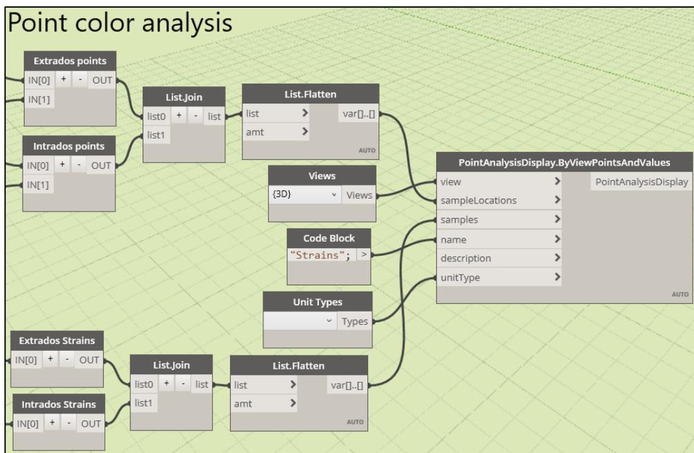
Figure 128: Smart-sensor data visualization. Point color analysis.
