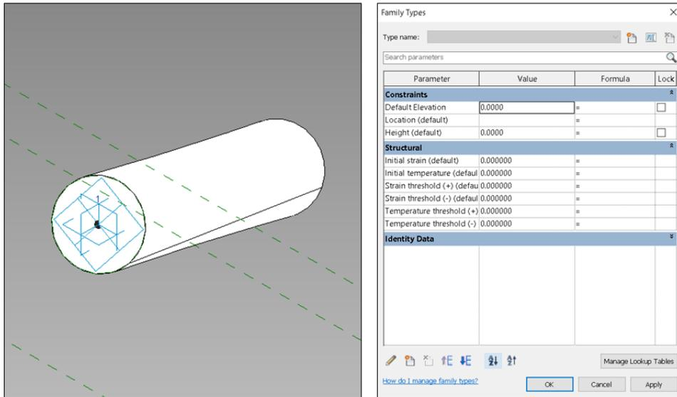
Figure 37: Strain multi-sensor family. Adaptive component and parameters.
