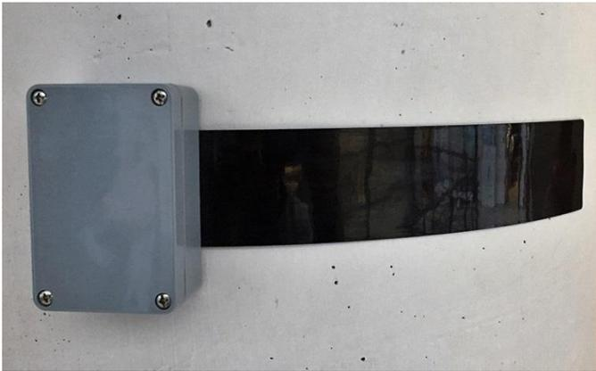
Figure 3: Foil strain gauge included in a multisensory device. SH BOX.
