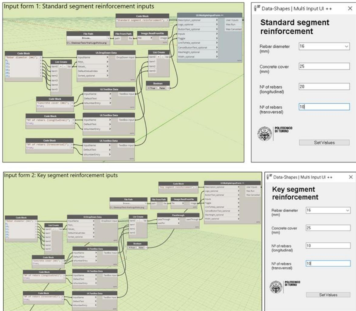
Figure 91: Tunnel reinforcement. Geometrical inputs.
