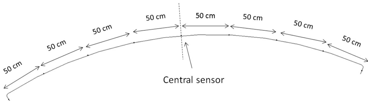
Figure 109: Smart sensor disposition. Transversal rebar.
