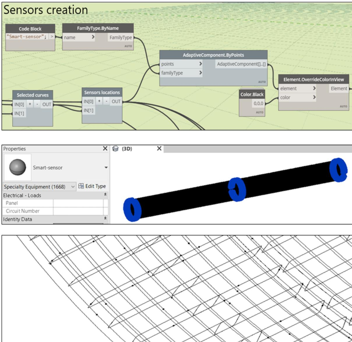
Figure 114: Tunnel SHM smart-sensors program. Smart-sensors creation.
