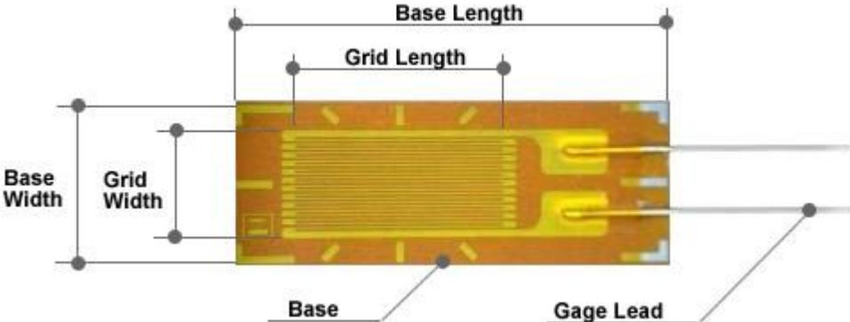
Figure 2: Foil strain gauge. Sensing sheet.
