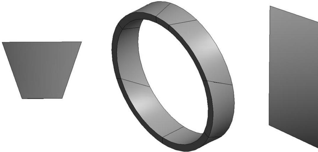
Figure 25: Tube pieces. Middle: Ring. Left: Key segment. Right: Standard segment.
