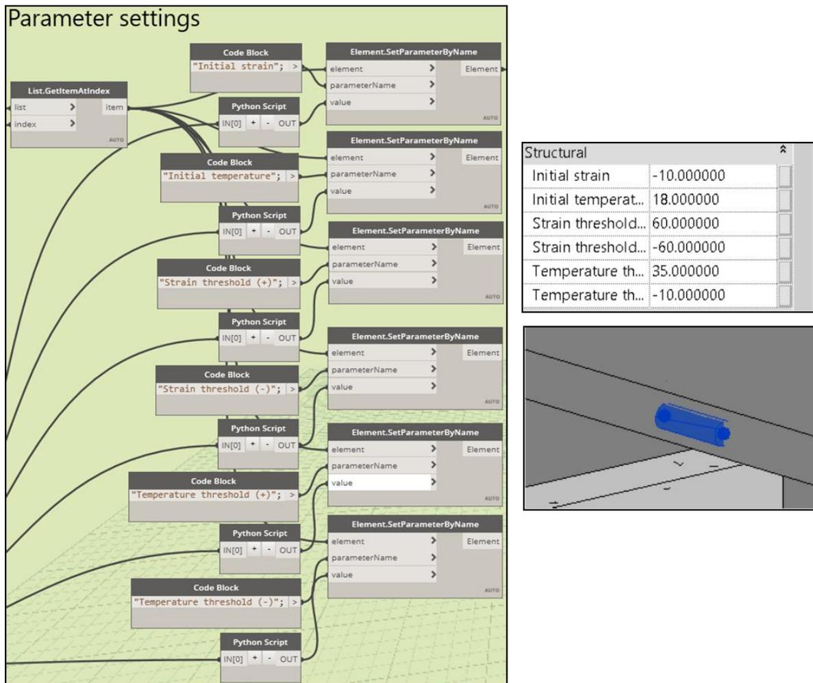
Figure 67: Bridge SHM initial values setting. Parameters setting.
