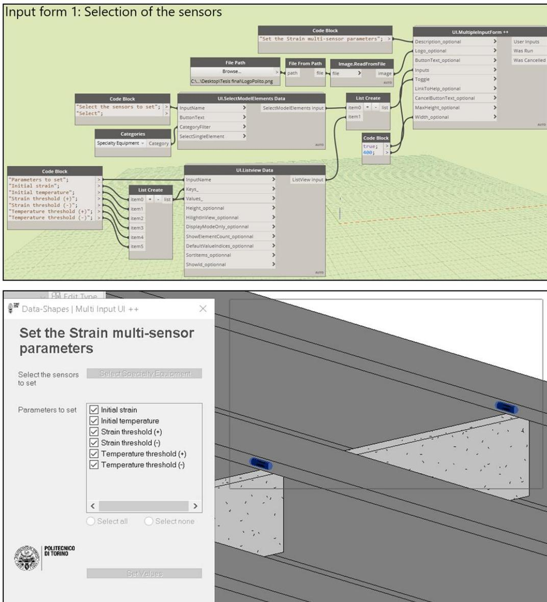
Figure 65: Bridge SHM initial values setting. Selection of the sensors.
