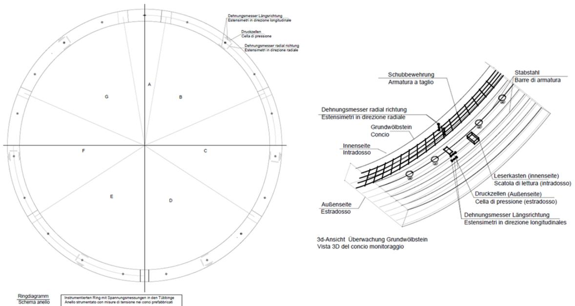
Figure 26: Tunnel monitoring system.
