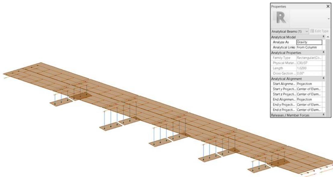
Figure 36: Revit prototype analytical model.
