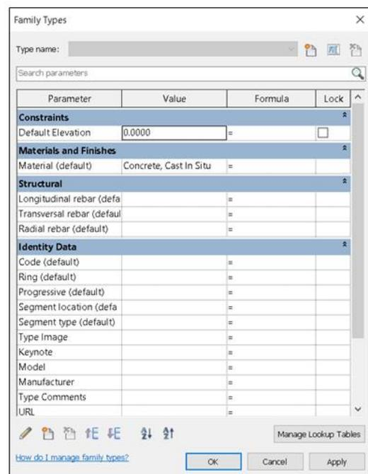
Figure 84: Tubing ring segment family. Adaptive component and parameters.
