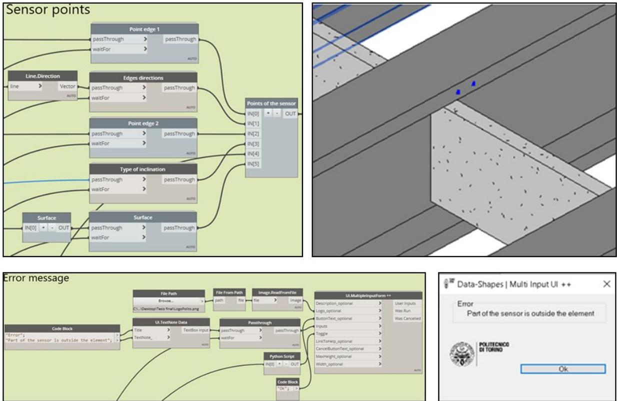
Figure 45: Bridge SHM strain multi-sensor placing. Points and error controlling.
