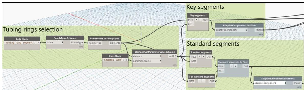
Figure 92: Tunnel reinforcement. Tubing ring segments selection and filtering.
