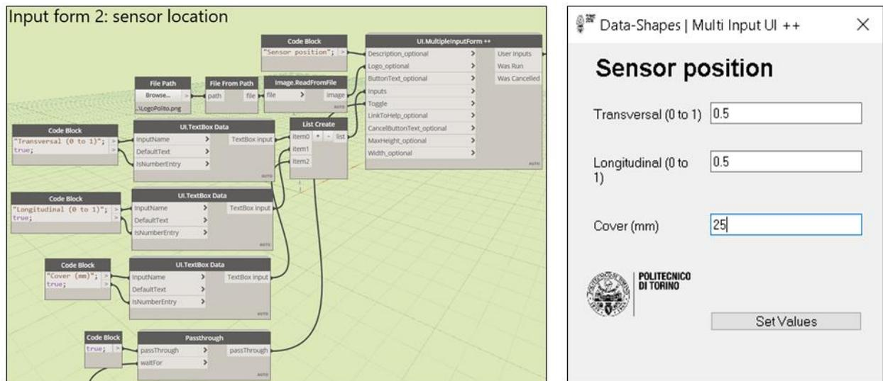
Figure 104: Tunnel SHM extensometers program. Location of the extensometers.
