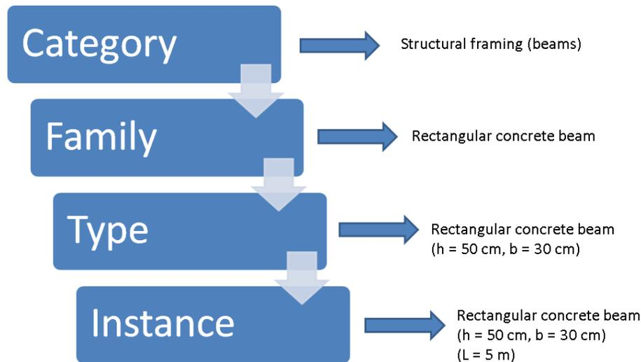
Figure 28: Revit elements hierarchy.
