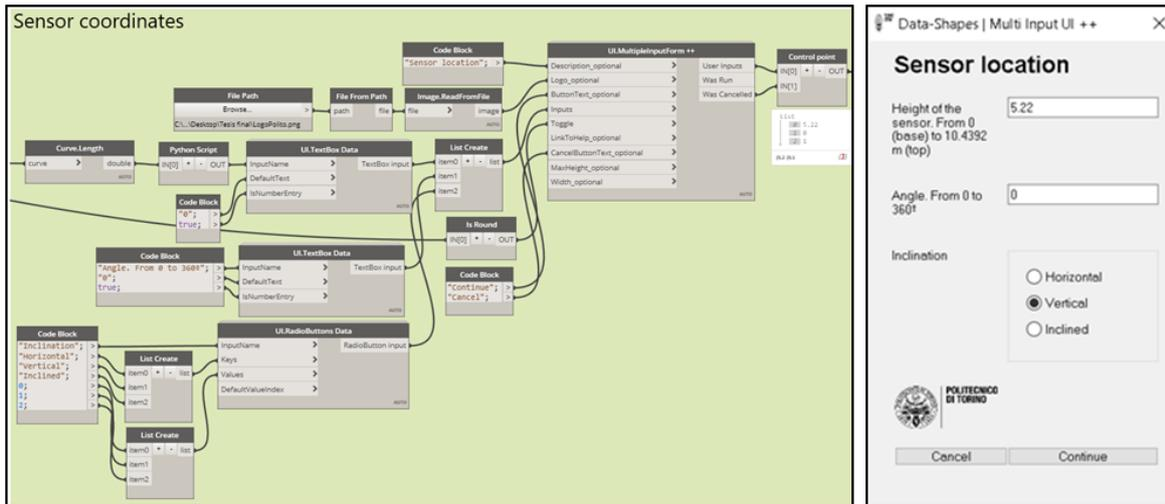
Figure 52: Bridge SHM strain multi-sensor placing. Sensor coordinates.
