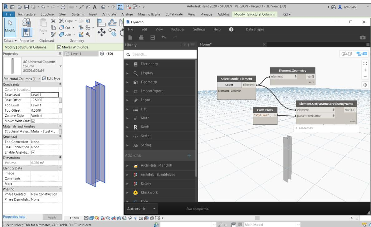
Figure 29: Real example of a Dynamo script.
