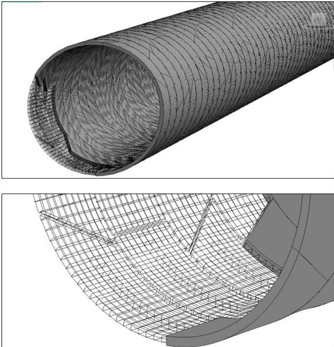
Figure 96: Tunnel reinforcement. Visualization.
