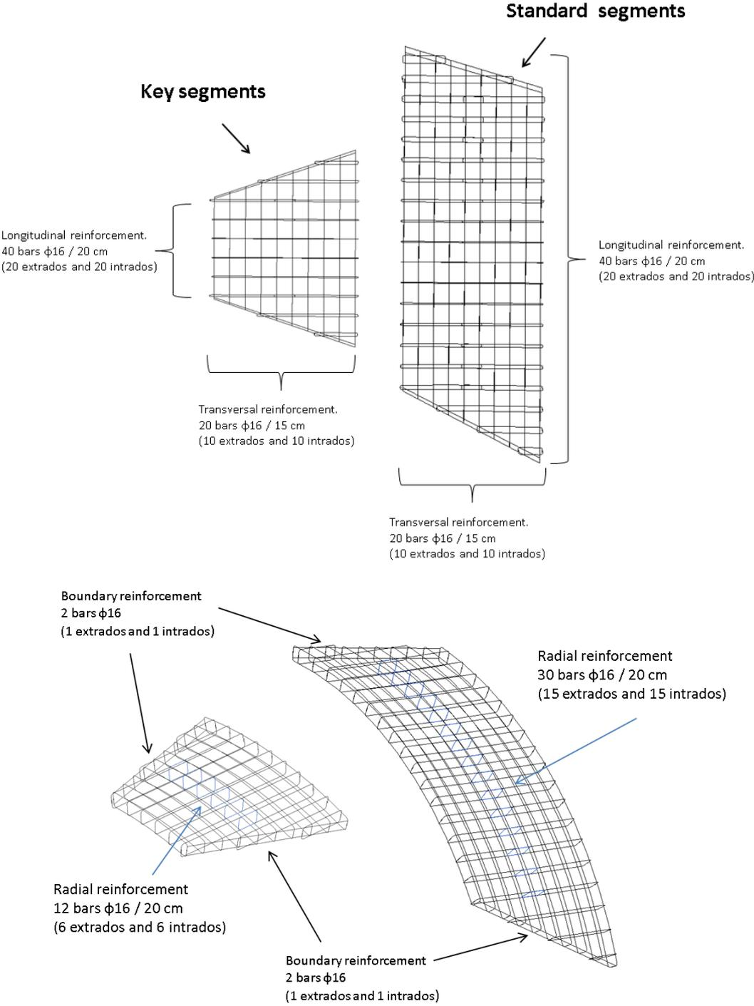
Figure 27: Brenner base tunnel. Reinforcement of the segments.
