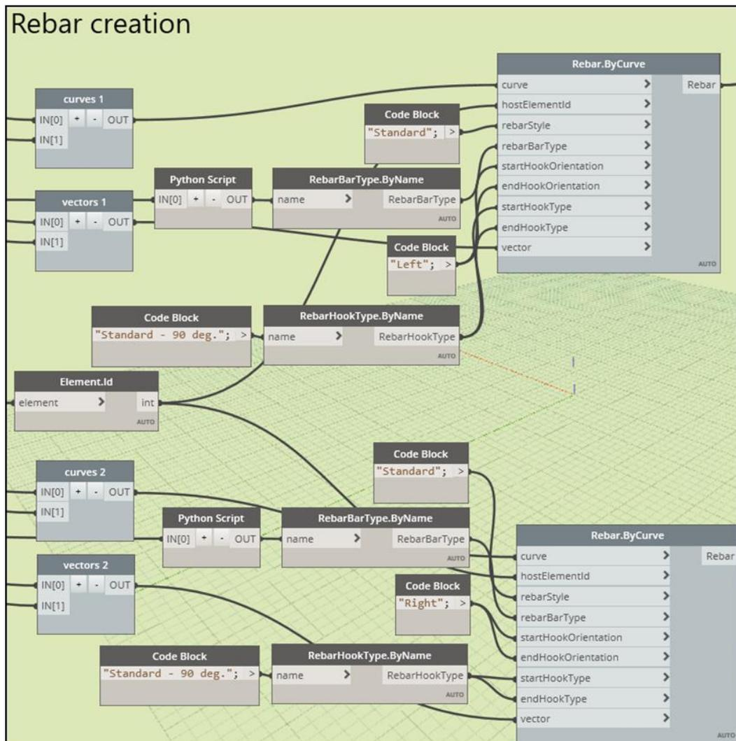
Figure 94: Tunnel reinforcement. Rebar creation.
