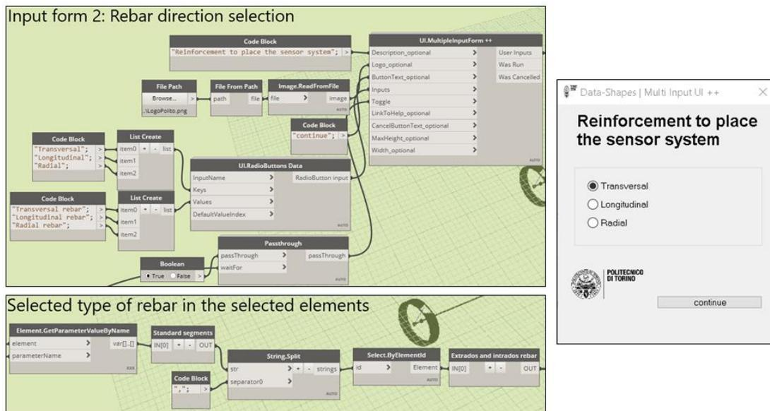
Figure 111: Tunnel SHM smart-sensors program. Reinforcement type selection.
