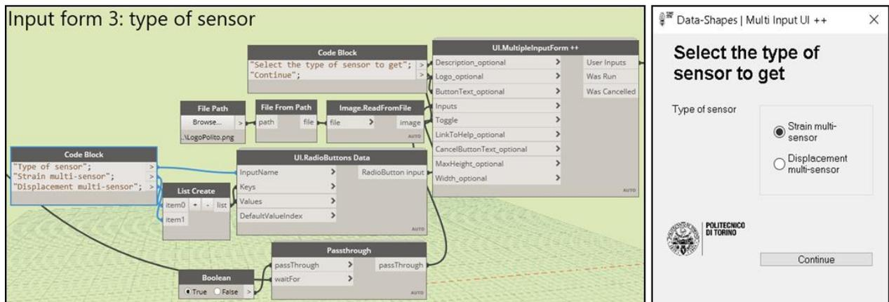
Figure 73: Bridge SHM data management. Selection of the sensor type.
