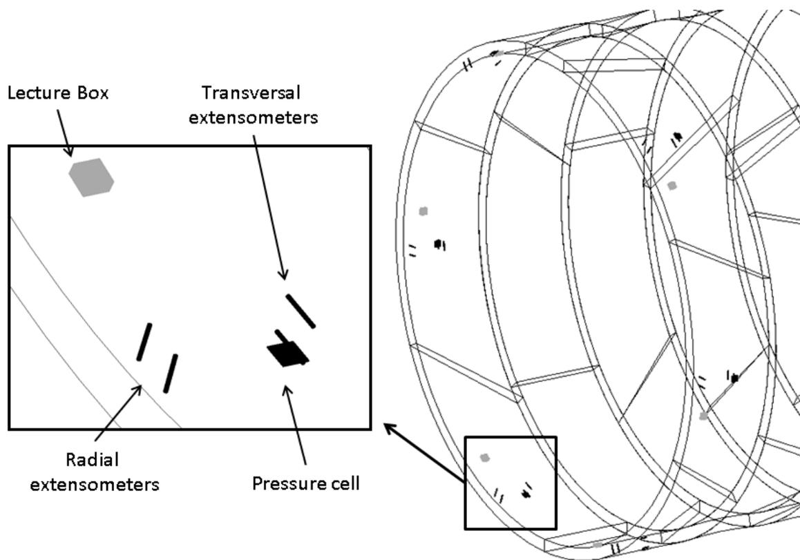
Figure 107: Tunnel SHM system.
