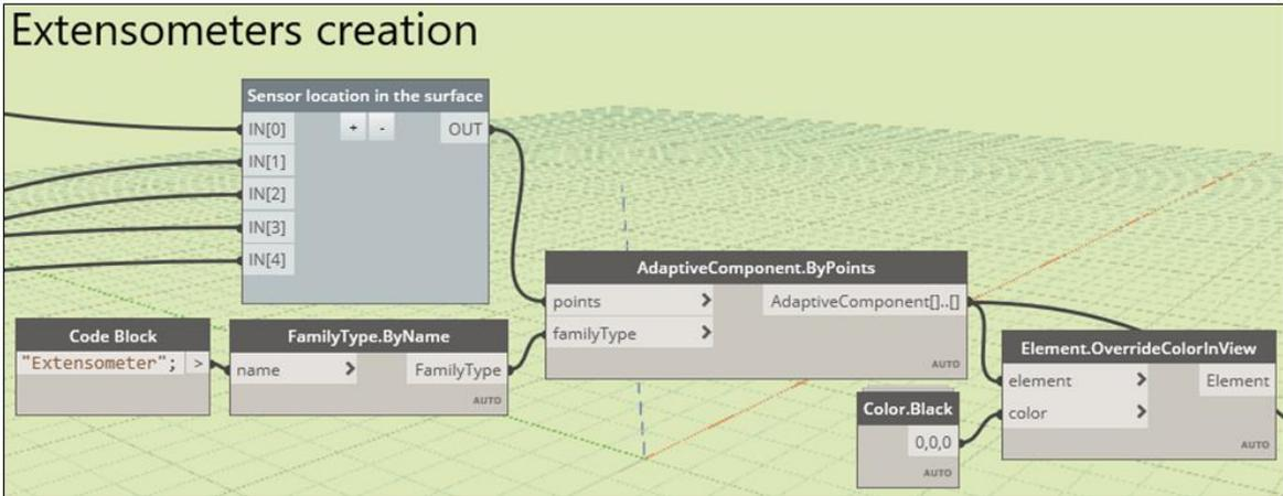
Figure 105: Tunnel SHM extensometers program. Extensometers creation.
