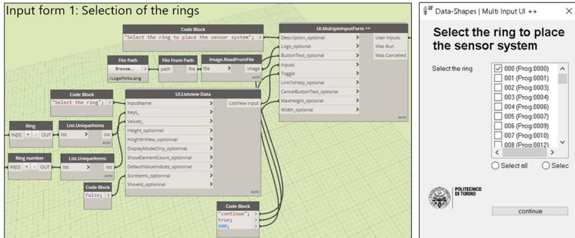
Figure 108: Tunnel SHM smart-sensors program. Rings selection.
