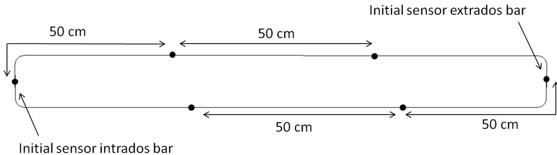
Figure 110: Smart sensor disposition. Transversal rebar.
