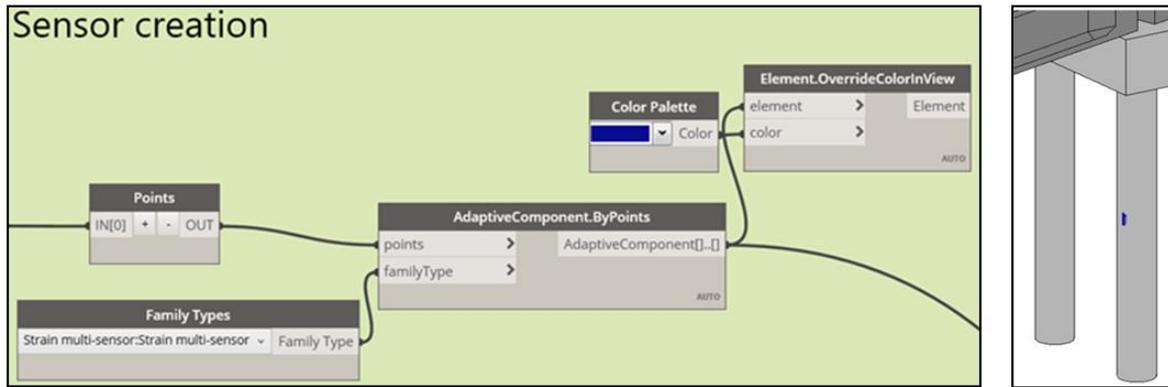
Figure 54: Bridge SHM strain multi-sensor placing. Sensor creation.
