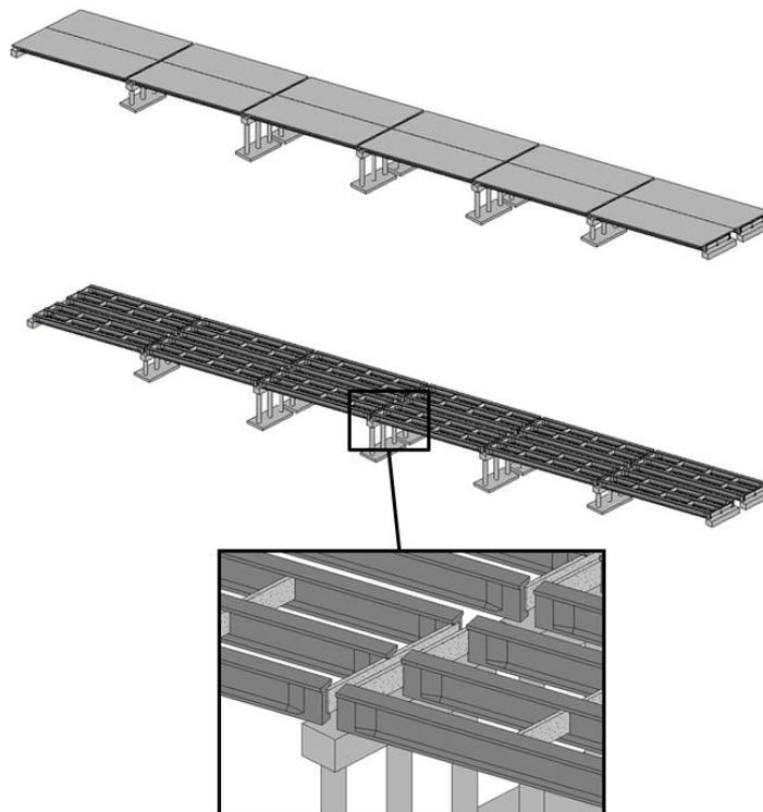
Figure 35: Revit model of the Stura Bridge. Complete (above). Hidden slab (below).
