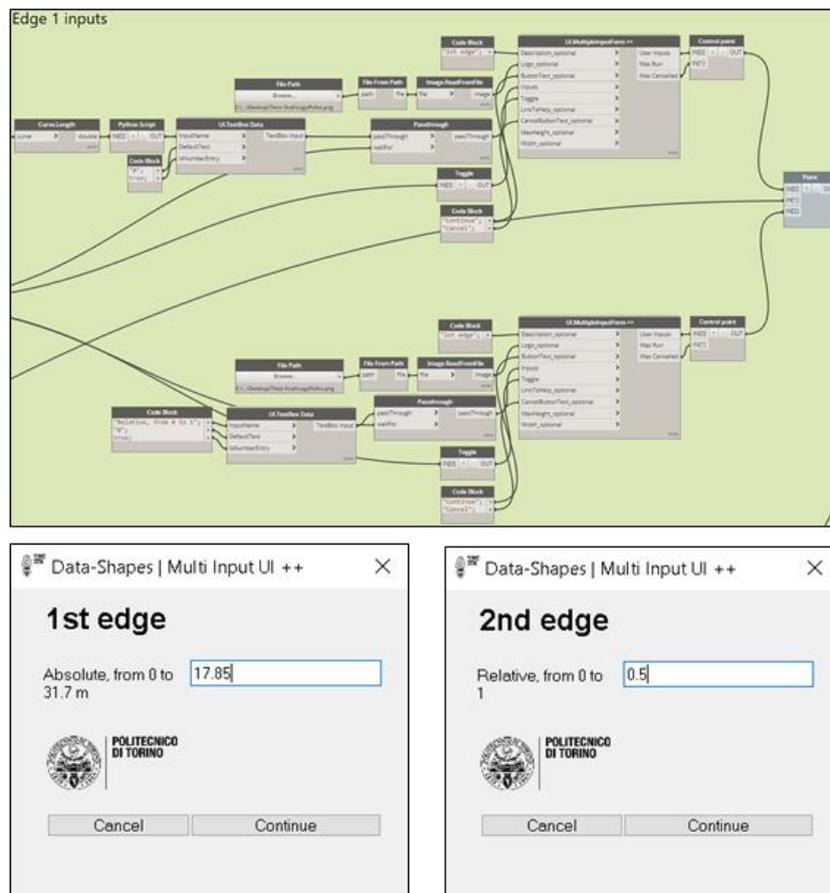
Figure 43: Bridge SHM strain multi-sensor placing. Coordinates introduction.
