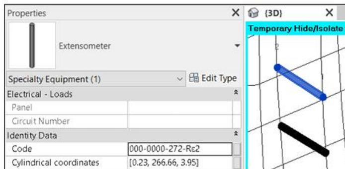
Figure 106: Tunnel SHM extensometers program. Parameters setting.
