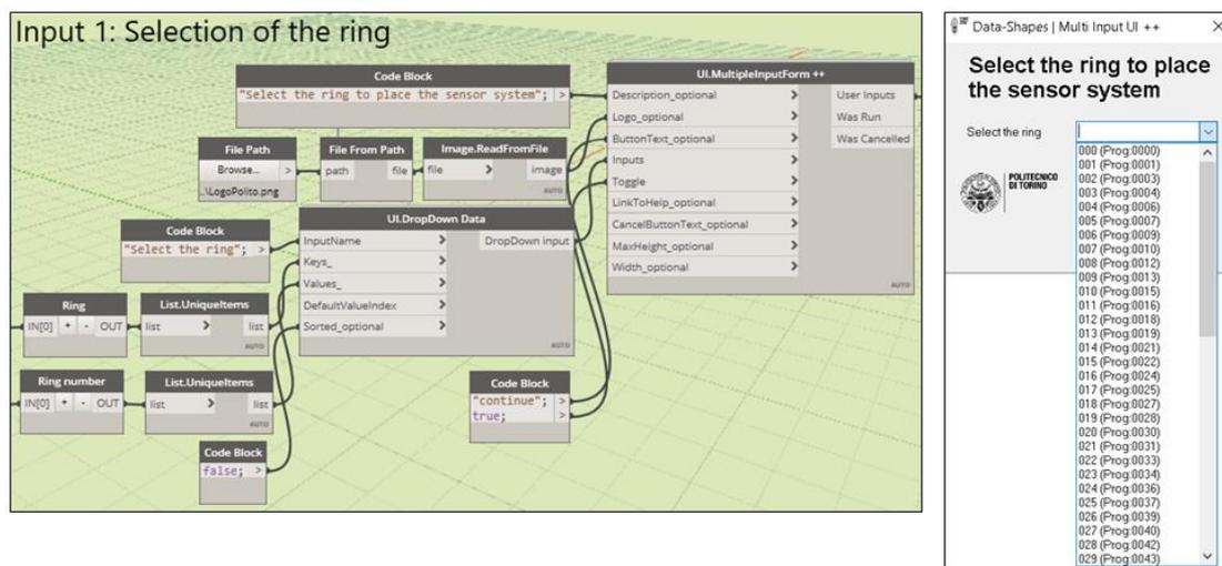
Figure 102: Tunnel SHM extensometers program. Selection of the ring.
