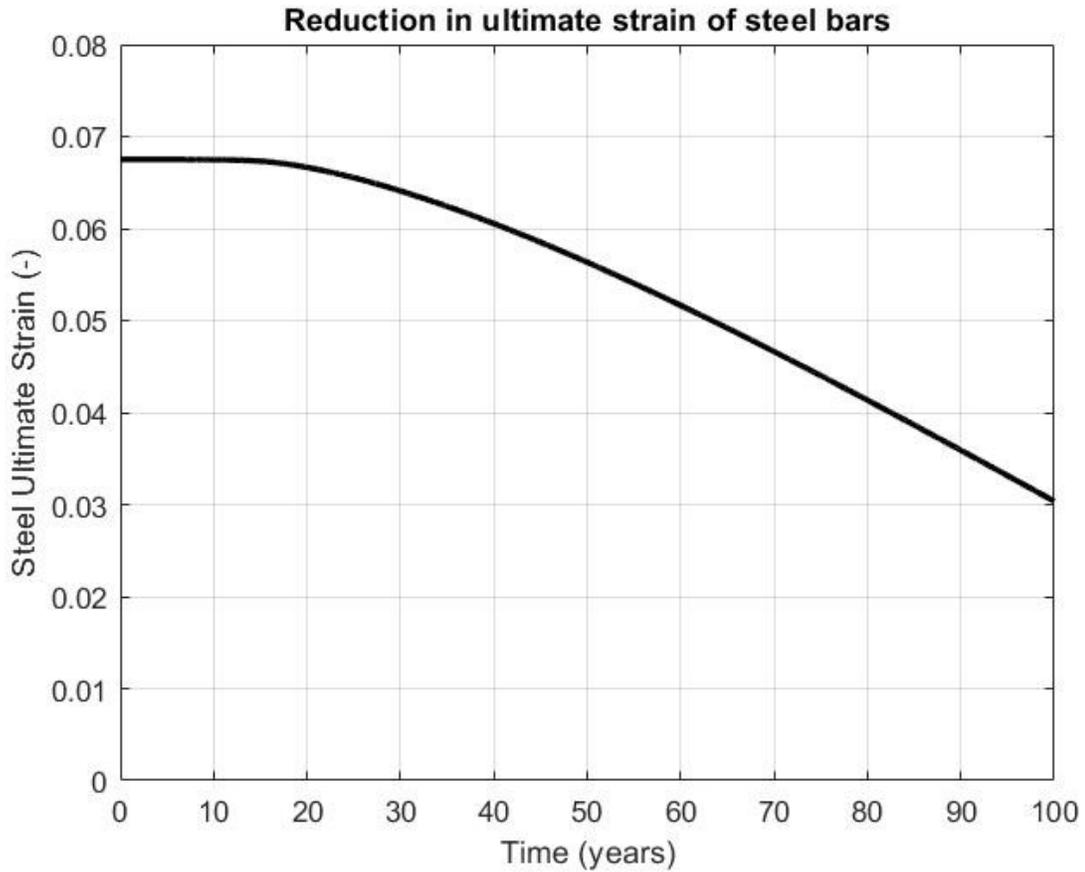
Figure 6.1: Reduction in ultimate strain of steel bars
