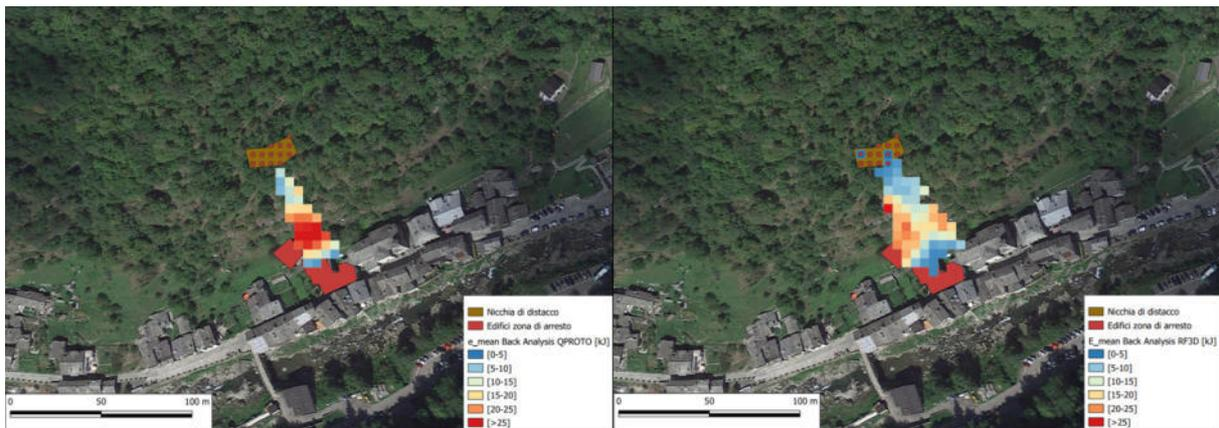
Figura 5.4-18: Confronto aree invasione/energie QPROTO (sx) e Rockyfor3D (dx)
