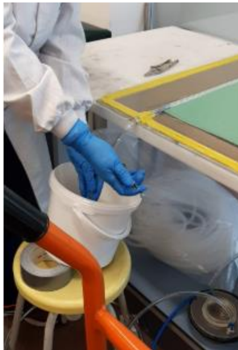
Figure 3.7: feeding step of the vacuum-bag system.
