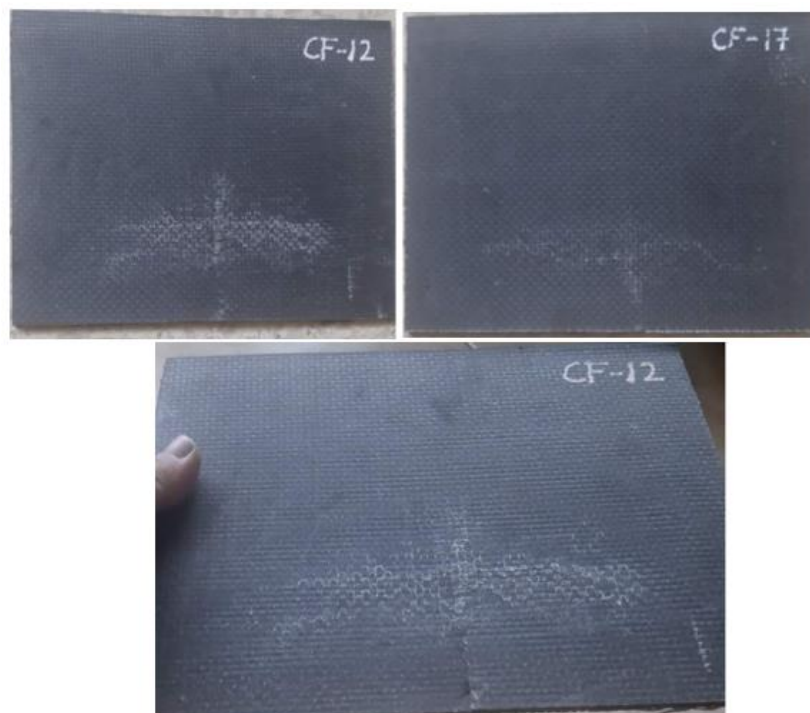
Figure 4.6: Carbon fiber samples photos after test and showing of the T shape fracture.
