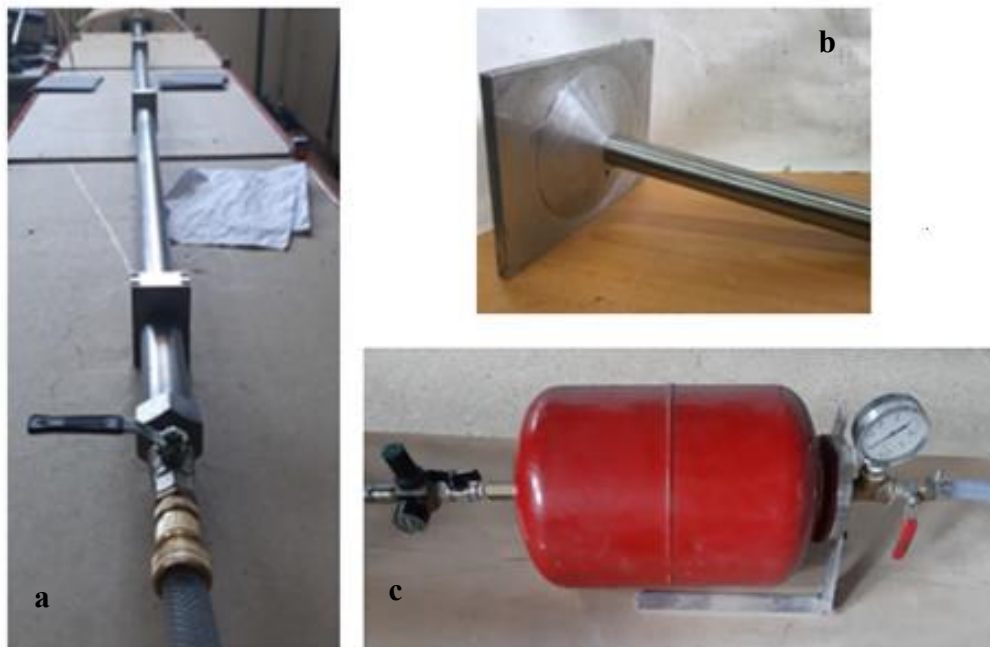
Figure 3.18: some elements of the experimental device a)bar with valve;b)piston and incident bar; c)air pressure tank.
