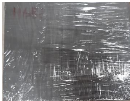
Figure 3.14: sample enveloped in the plastic film after the saturation in salt-water.
