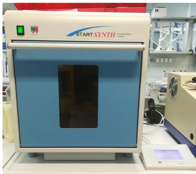
Figure 3.1: The microwave oven used for the synthesis of the materials: a Milestone START-Synth with temperature and pressure control.
