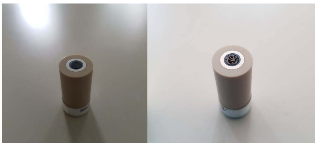
Figure 5.4: Successful (left) and failed (right) preparation of the paste for GC/Pt electrode.
