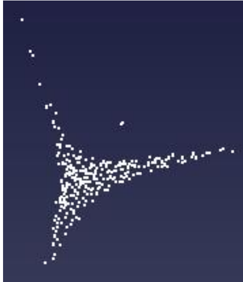
Figure 10: Representation of the geometry obtained from the intersection of the original cube with 3 hyperbolic cylinders.
