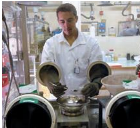
Figure 2: An operator weighting powder using a glove box in the CEA Cadarache research center. Image coming from the website: http://www.cea.fr/english/Pages/research-areas/nuclear-energy/nuclear-fuel.aspx?Type=Chapitre&numero=3 .
