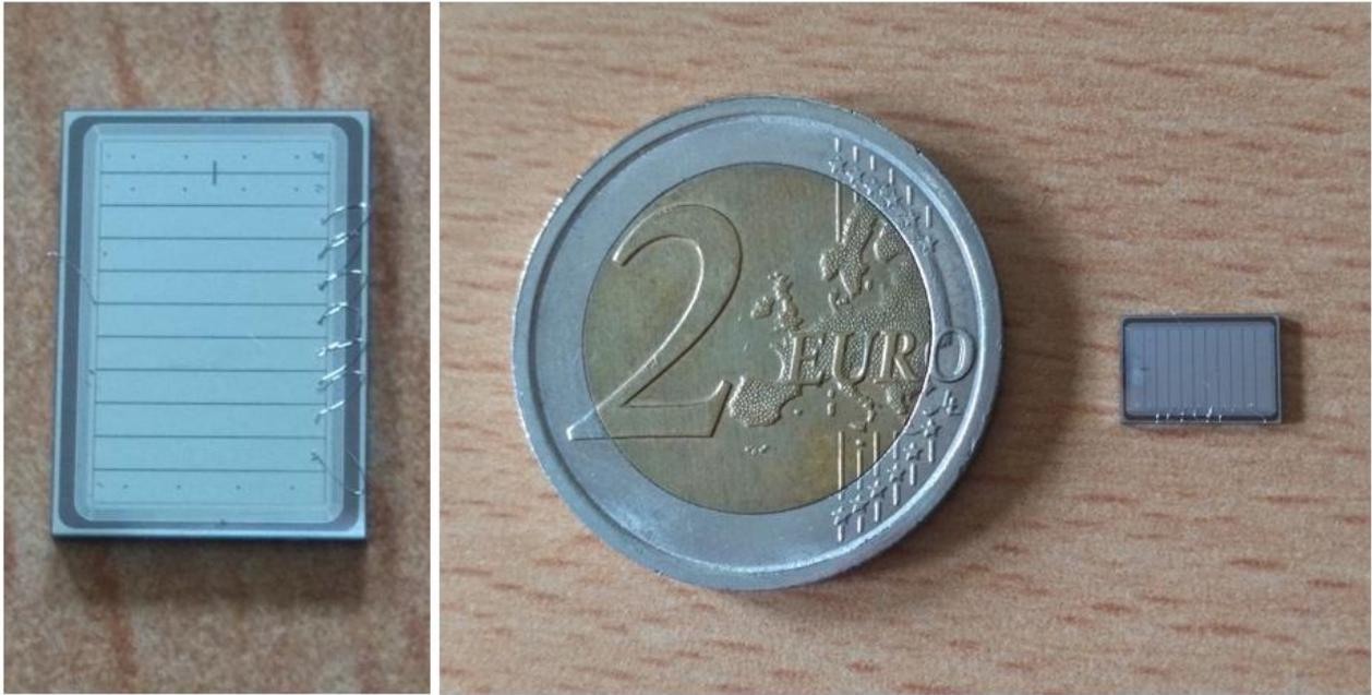
Figure 2.3: FBK UFSD detector segmented in 11 strips.
