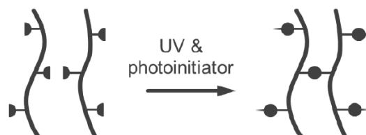
Figure 24: Scheme of photocurable polymer with pendant photosensitive groups [18].
