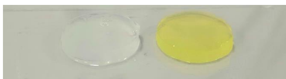
Figure 100: EDA3350_3% hydrogel sample control (Left) and after 1d of FD4 absorption (Right).
