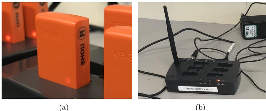
Figure 4.1: Some components of the Xsens MVN: a) Wireless Motion Tracker (MTw); b) Awinda Station.
