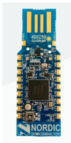
Figure 3.2: nRF52840 Dongle of Nordic Semiconductor®. [22]
