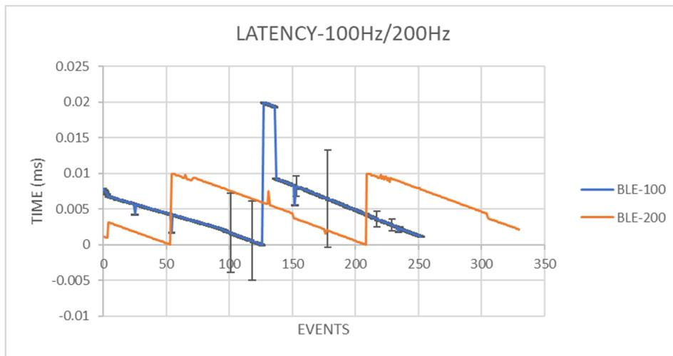
Figure 5.2: BLE Latency Measurement.
