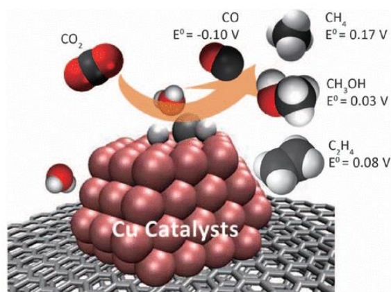
Figure 1.5: Schematic illustration of the CO 2 reduction reaction on Cu catalysts. Taken from (Marken & Fermin, 2018)
