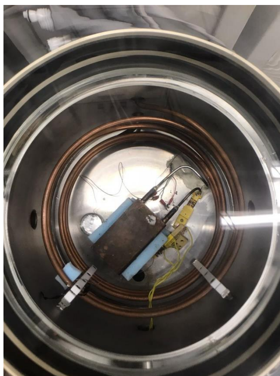
Figure 3.10: Image taken from inside the chamber: detail of the condenser and the shelf.
