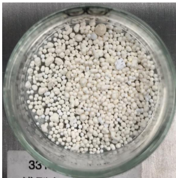
Figure 3.13: Sample dried from the liquid solution 5% w/w trehalose 5% w/w albumin atomized with the vibrating needle.
