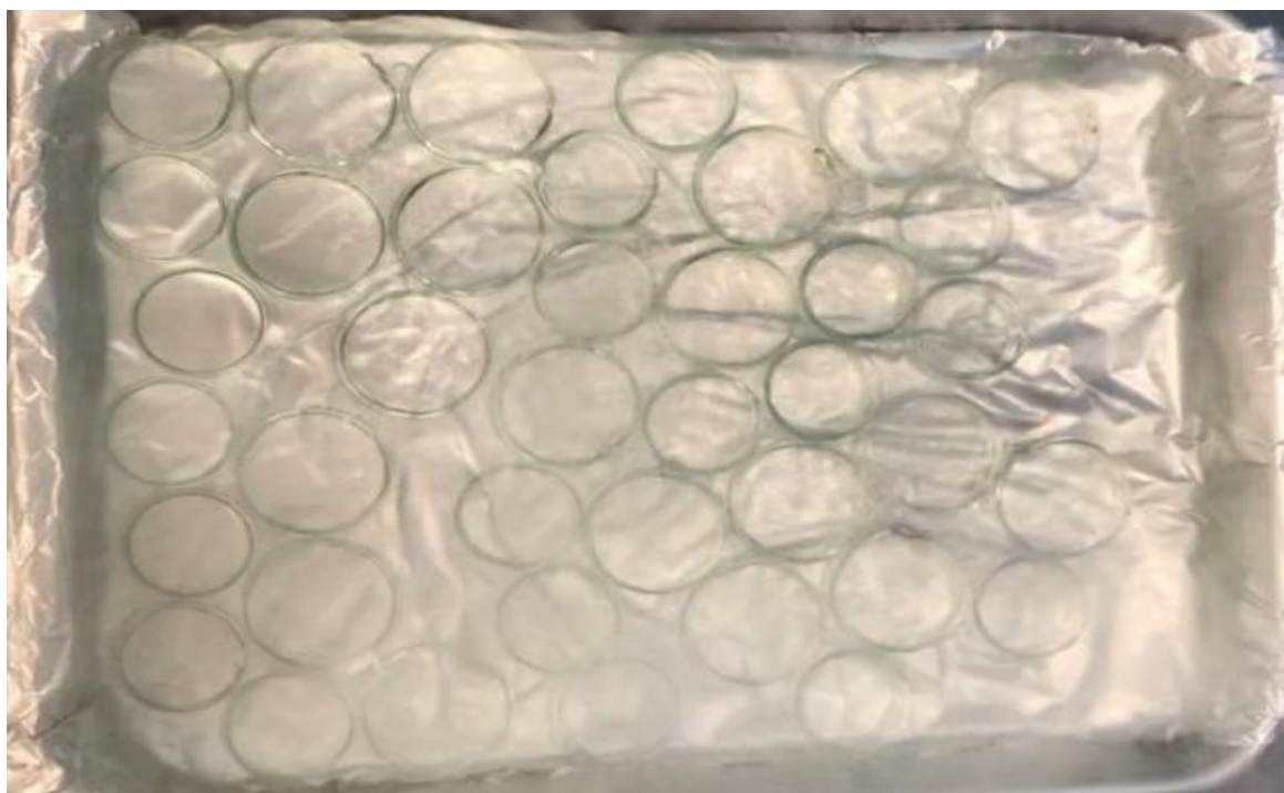
Figure 3.7: Tray used at Kyoto University containing liquid nitrogen to freeze the particles.
