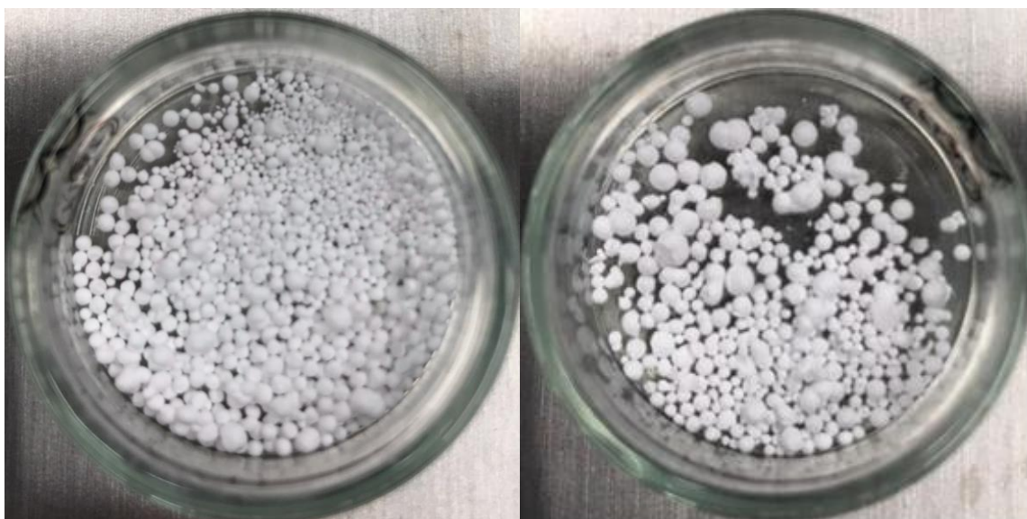
Figure 3.12: samples dried from a liquid solution 10% w/w (left) and 15% w/w (right) of mannitol. Both obtained atomizing with the vibrating needle.
