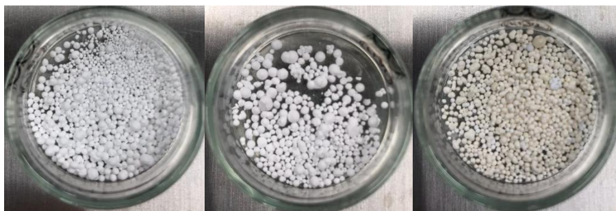
Figure 3.6: Particles obtained with the vibrating atomization method. The particles look more spherical hence to facilitate the investigation of its internal surface.
