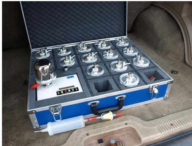
Figure 1.4 - Chambers, syringe, and Radon detector (Arco, 2017)
