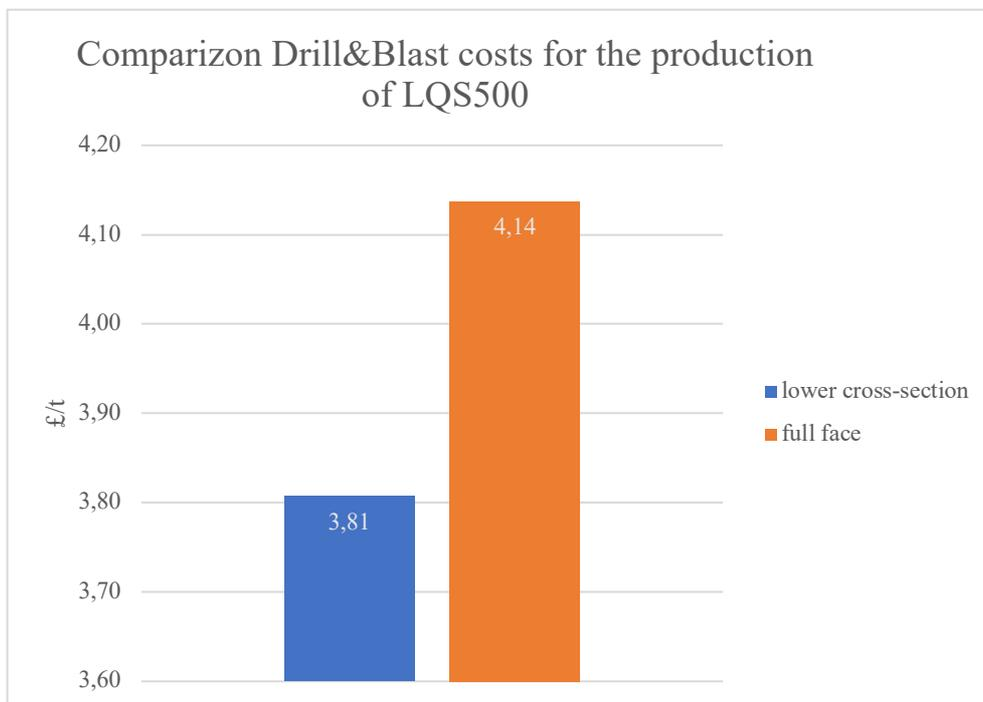
Figure 5.8 Comparison between the cost/t of the two blasting schemes
