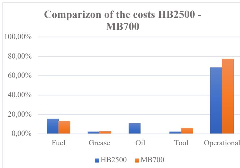
Figure 5.11 Comparison of the cost's distribution between HB2500 and MB700
