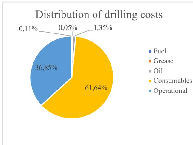
Figure 5.2 Cost Distribution - Drill and Blast - Drilling costs
