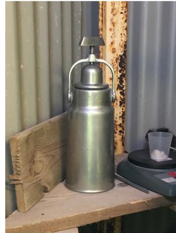
Figure I.12 Speedy Protimeter test flask
