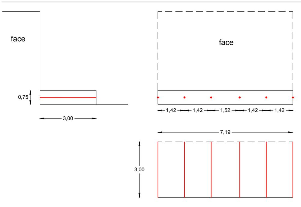
Figure IV.13 New blasting scheme for bench blasting
