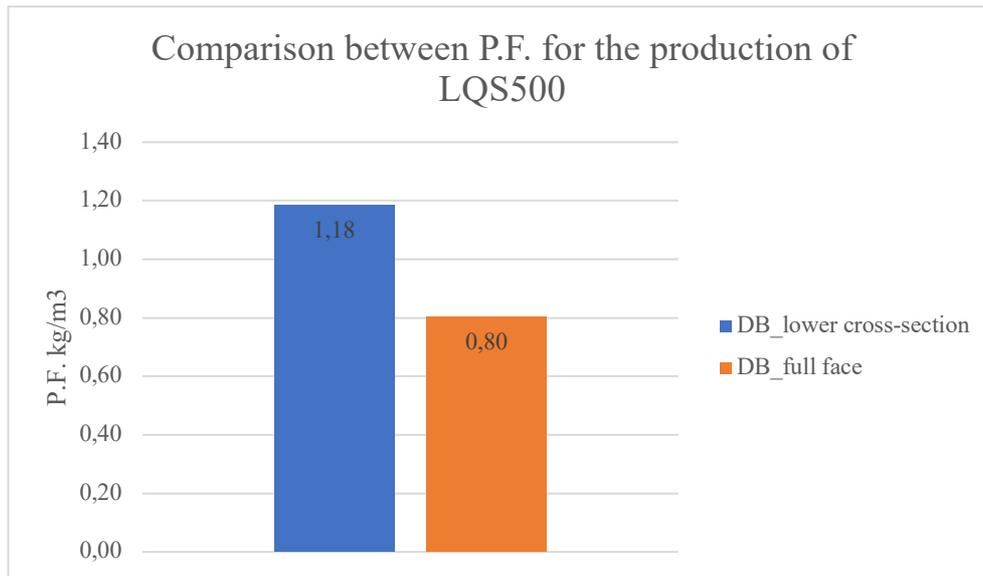
Figure 5.7 Comparison between the P.F. of the two blasting schemes
