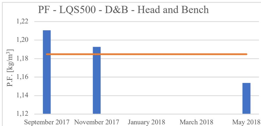
Figure IV.5 Distribution P.F. - LQS 500 - D&B - Head and Bench
