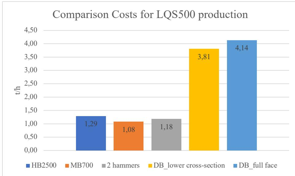
Figure 5.12 Comparison of the costs [£/t] for each technique
