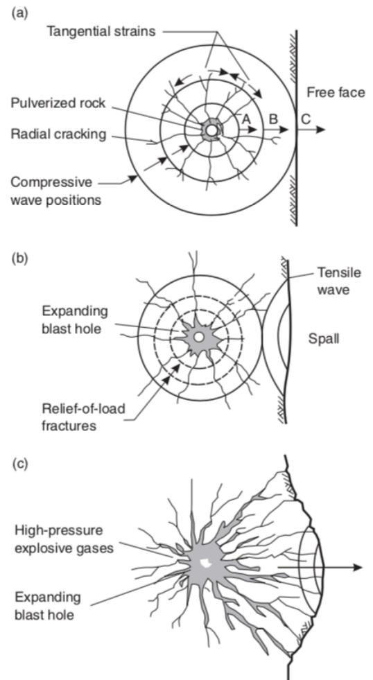
Figure III.1 Mechanism of rock breakage by explosives
