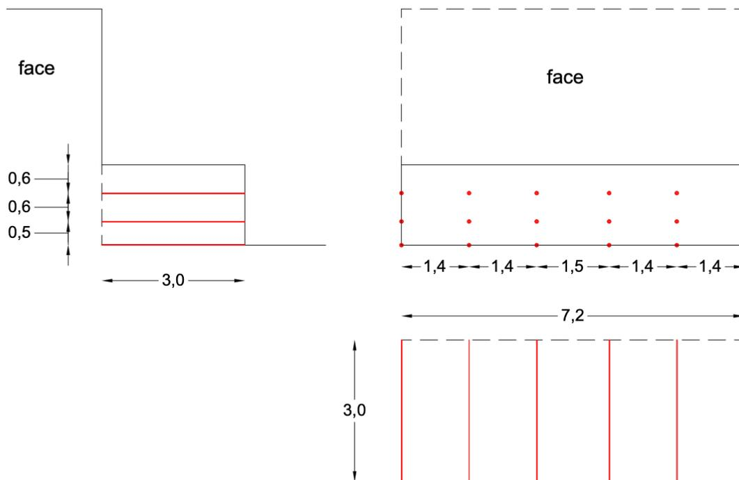
Figure IV.6 Scheme of the bench exploitation with drill and blast
