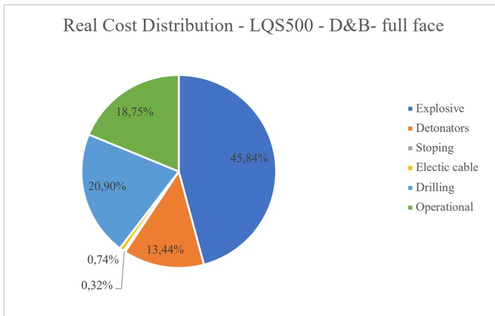
Figure 5.6 Percentage distribution of the blast - Full face – real production
