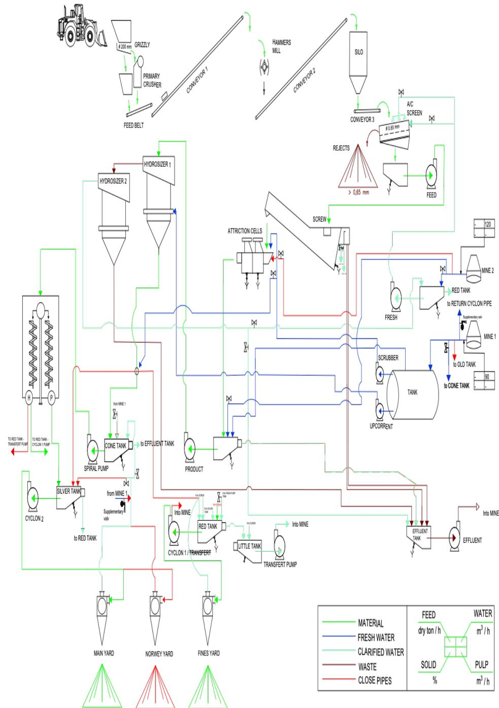
Figure I.6 Treatment Plant Flowsheet - LQS85 treatment
