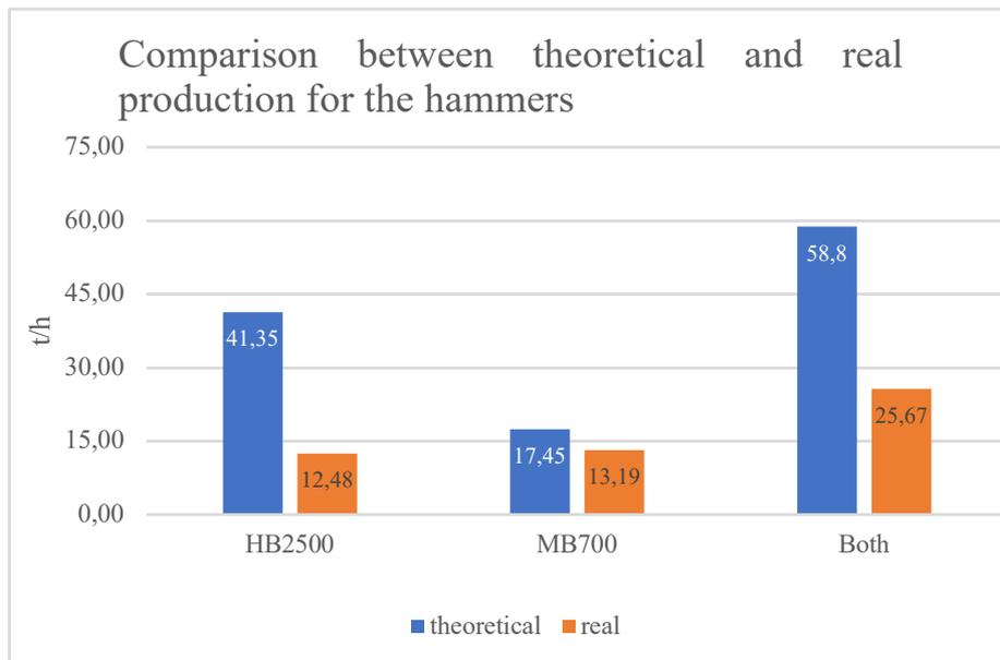
Figure IV.9 Comparison between theoretical and real production for the hammers
