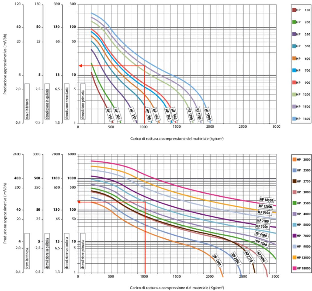
Figure IV.7 Indeco's indicative values for the production with hydraulic hammer
