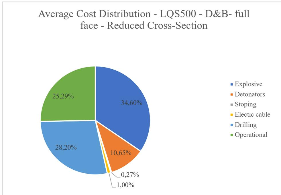
Figure 5.3 Percentage Distribution of the Costs - D&B - full face analysis, reduced cross-section
