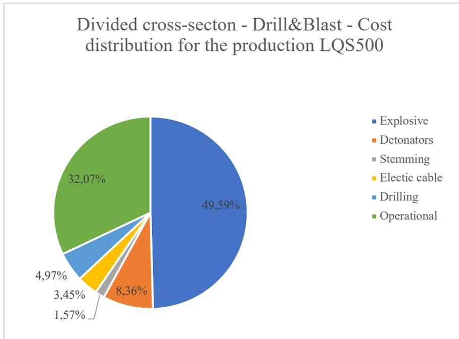
Figure 5.1 Percentage distribution of the costs – D&B – Lower cross-section
