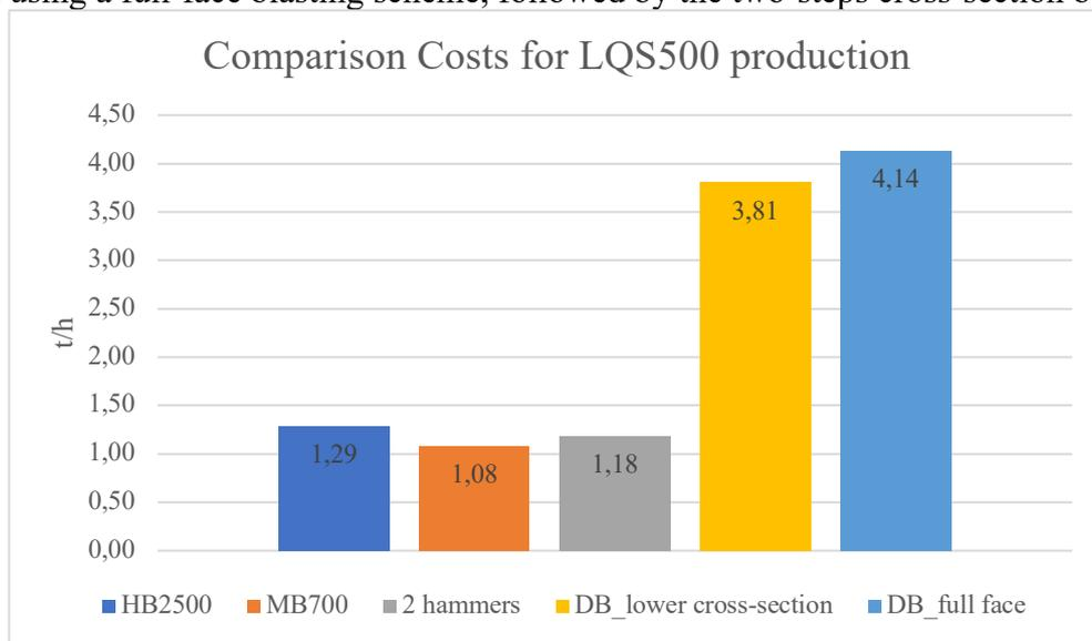
Figure IV.14 Comparison between the average production of the different techniques
