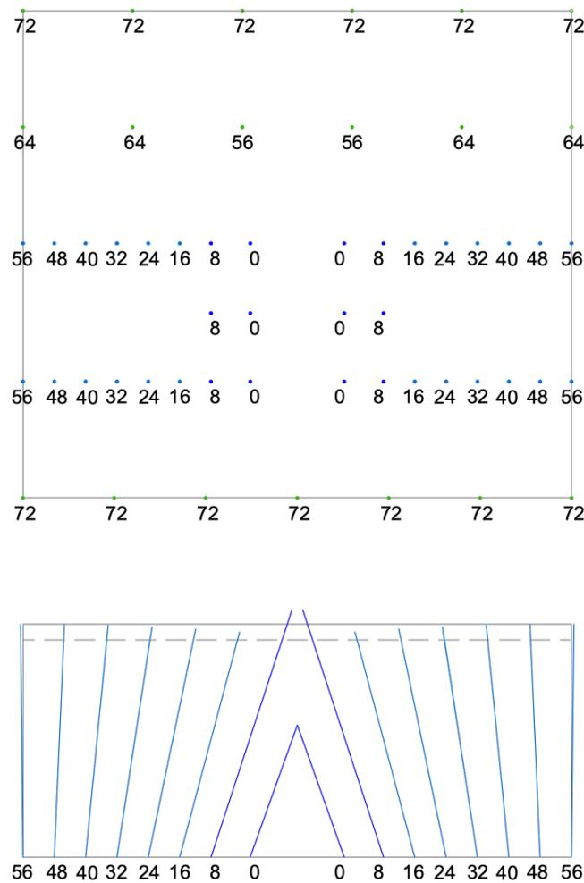
Figure IV.10 Blasting scheme for the production of LQS500
