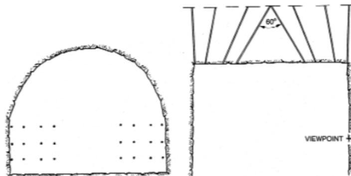
Figure IV.1 V-cut theoretical scheme
