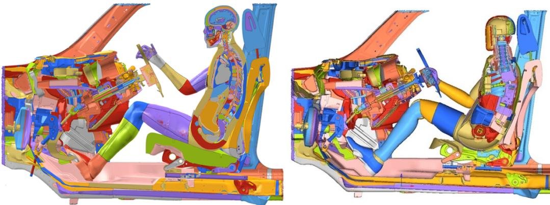
Figure 5.44. Positioned THUMS (left) vs THOR (right) - side  $xz$  section view – ODB– 0 ms
