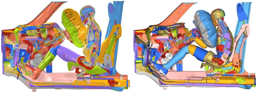
**Figure 5.49.** Positioned THUMS (left) vs THOR (right) - side  $xz$  section view – ODB – 75 ms
