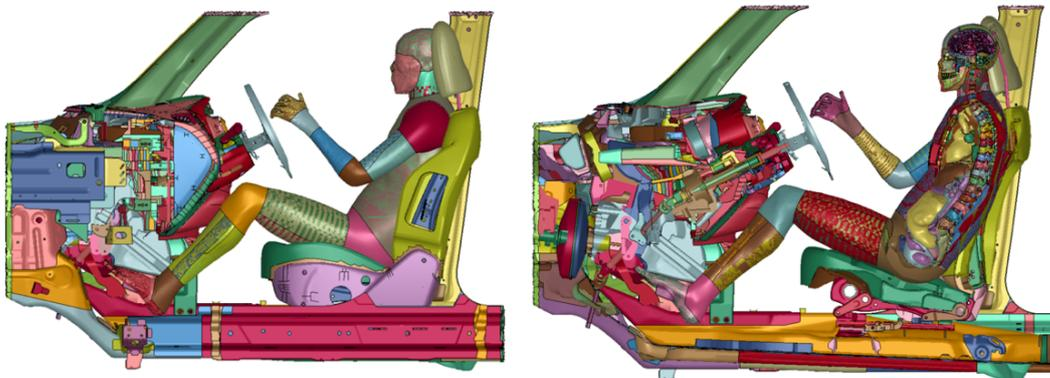
**Figure 3.10.** Original THUMS in vehicle FE model – side  $xz$  (left) and section (right) views
