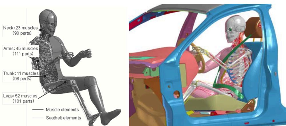
**Figure 1.37.** THUMS Version 5 - Occupant model (left) [8] and seated in a passenger car FE model (right) [9]
