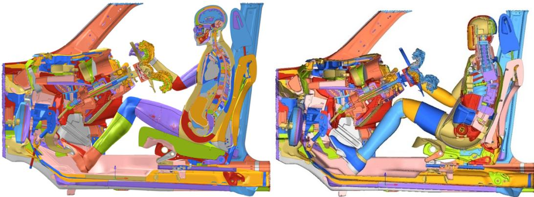
**Figure 5.9.** Positioned THUMS (left) vs THOR (right) - side  $xz$  section view – FWRB – 15 ms
