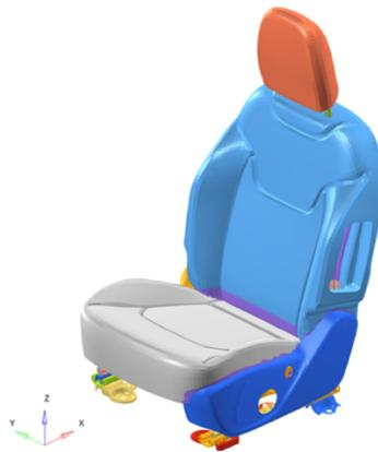
**Figure 4.15.** Undeformed vehicle seat FE model
