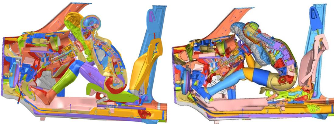
**Figure 5.15** Positioned THUMS (left) vs THOR (right) - side *xz* section view – FWRB – 100 ms
