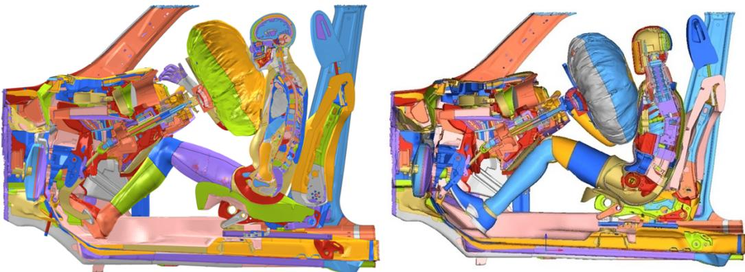
**Figure 5.48.** Positioned THUMS (left) vs THOR (right) - side  $xz$  section view – ODB – 60 ms
