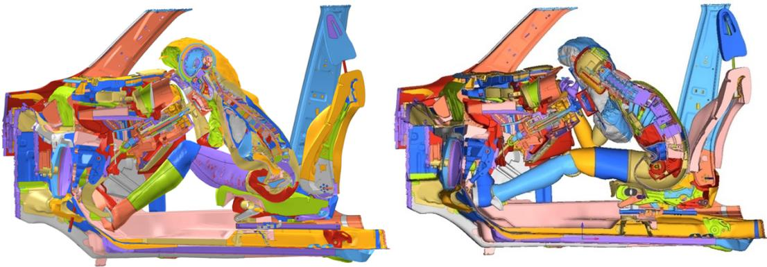
**Figure 5.53.** Positioned THUMS (left) vs THOR (right) - side  $xz$  section view – ODB – 130 ms
