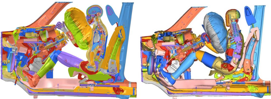
**Figure 5.11.** Positioned THUMS (left) vs THOR (right) - side  $xz$  section view – FWRB – 45 ms
