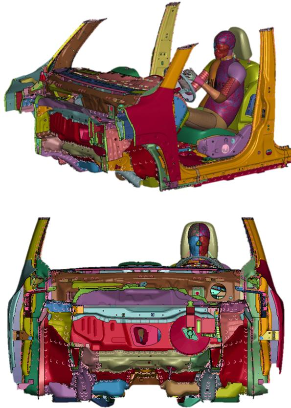
Figure 3.11. Original THUMS in vehicle FE model – isometric (above) and frontal (below) views
