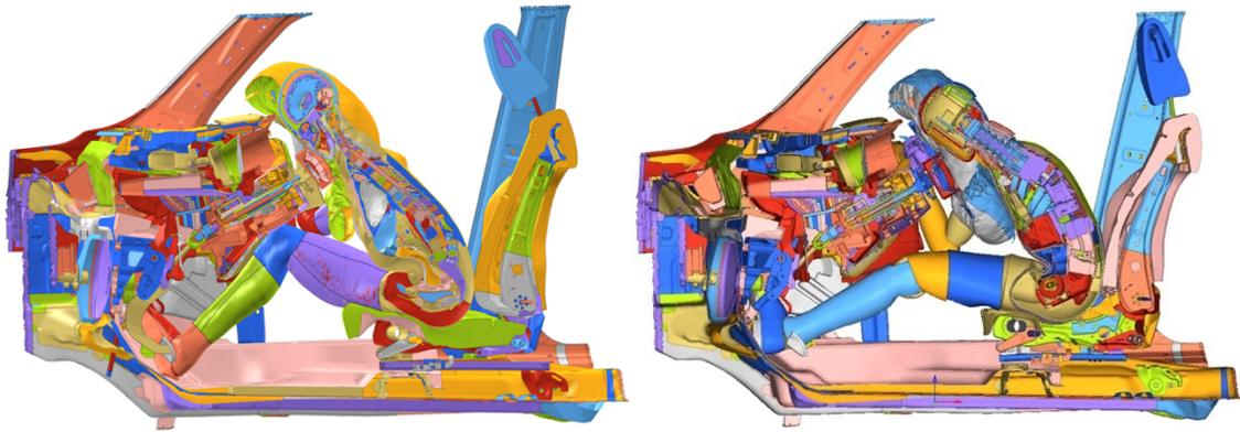
**Figure 5.52.** Positioned THUMS (left) vs THOR (right) - side  $xz$  section view – ODB– 120 ms
