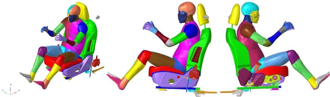
**Figure 4.25.** Positioned THUMS model – Seatbelt creation – Starting point of the realization process – isometric (left), side left plane,  $xz$  (middle) and side right plane  $-xz$  (right)
