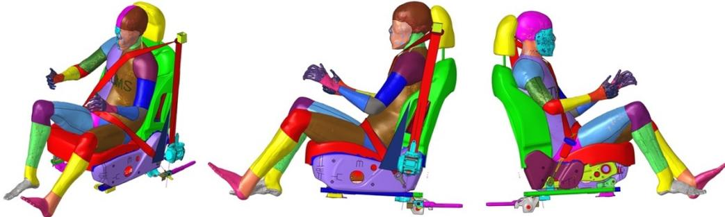
**Figure 4.28.** THUMS OOP – Seatbelt creation – Definitive Seatbelt on Positioned THUMS process – isometric (left), side left plane,  $xz$  (middle) and side right plane  $-xz$  (right)
