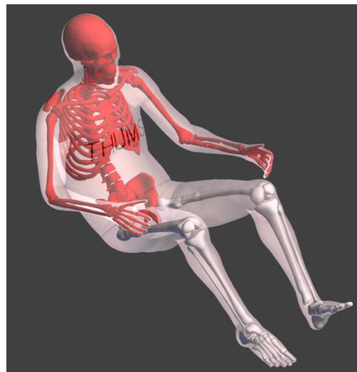
**Figure 3.14.** PIPER software – HBM Positioning: Fixed Bones represented in red – The reported configuration is the one used, for instance, to correctly position the legs, without moving the other bones
