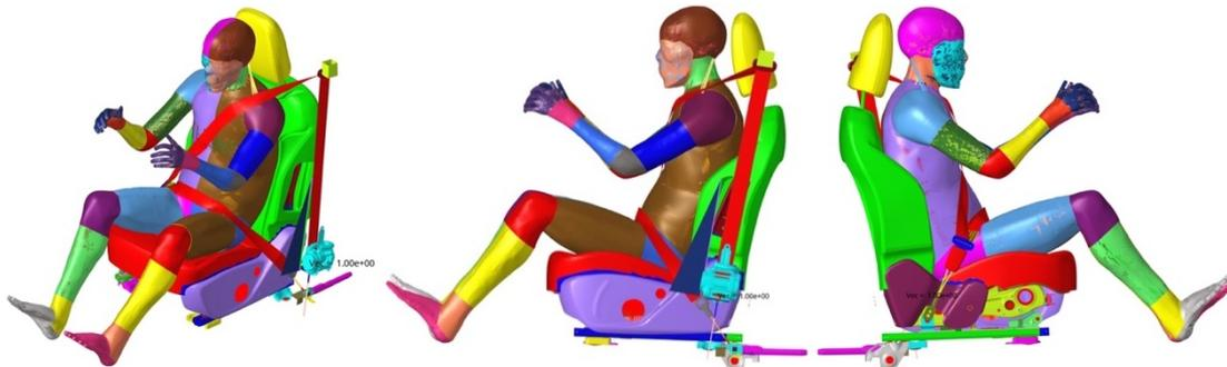
Figure 4.27. Positioned THUMS model – Seatbelt creation – Definitive Seatbelt on Positioned THUMS process – isometric (left), side left plane, *xz* (middle) and side right plane *-xz* (right)
