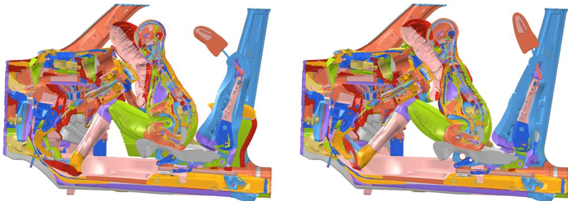
**Figure 6.9.** THUMS in OOP (left) vs THUMS in driving posture (right) - side  $xz$  section view – FWRB – 75 ms
