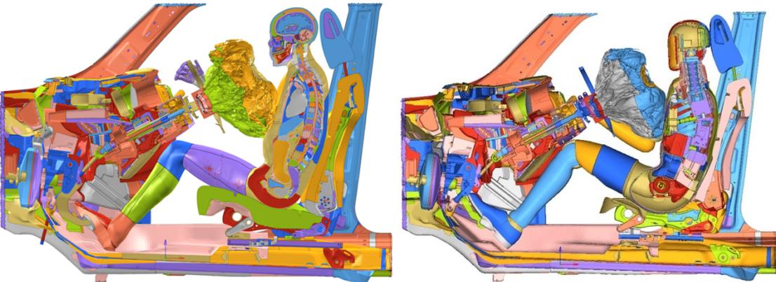
**Figure 5.10.** Positioned THUMS (left) vs THOR (right) - side  $xz$  section view – FWRB – 30 ms
