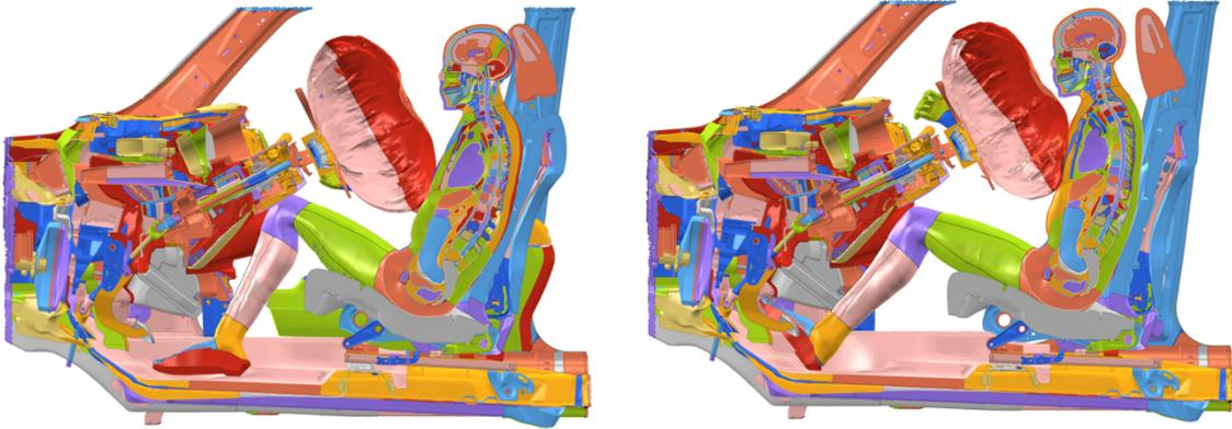
Figure 6.41. THUMS in OOP (left) vs THUMS in driving posture (right) - side  $xz$  section view ODB – 45 ms
