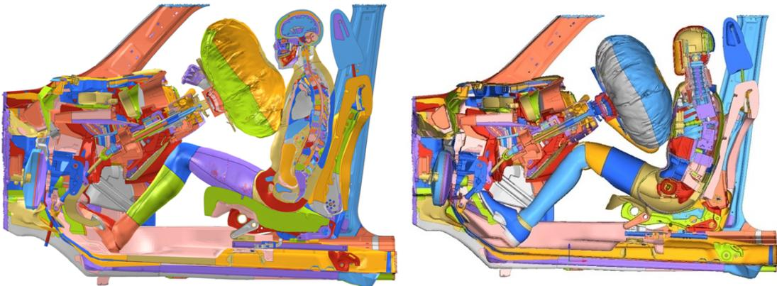
**Figure 5.47.** Positioned THUMS (left) vs THOR (right) - side  $xz$  section view – ODB – 45 ms
