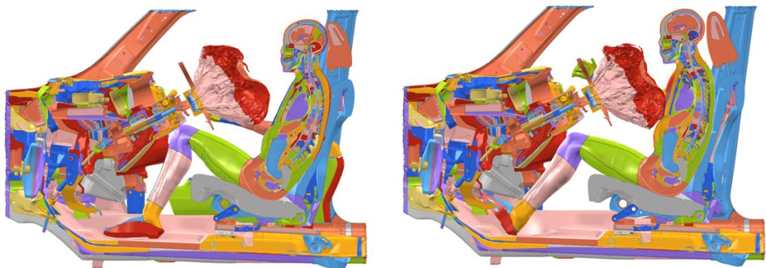
**Figure 6.40.** THUMS in OOP (left) vs THUMS in driving posture (right) - side  $xz$  section view – ODB – 30 ms
