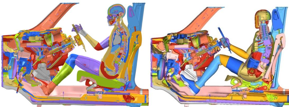
Figure 5.8. Positioned THUMS (left) vs THOR (right) - side xz section view – FWRB – 0 ms
