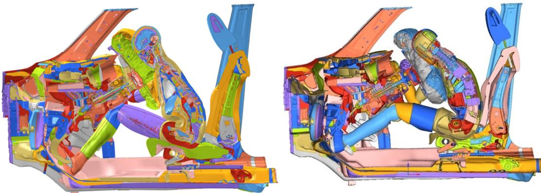
**Figure 5.51.** Positioned THUMS (left) vs THOR (right) - side  $xz$  section view – ODB – 105 ms
