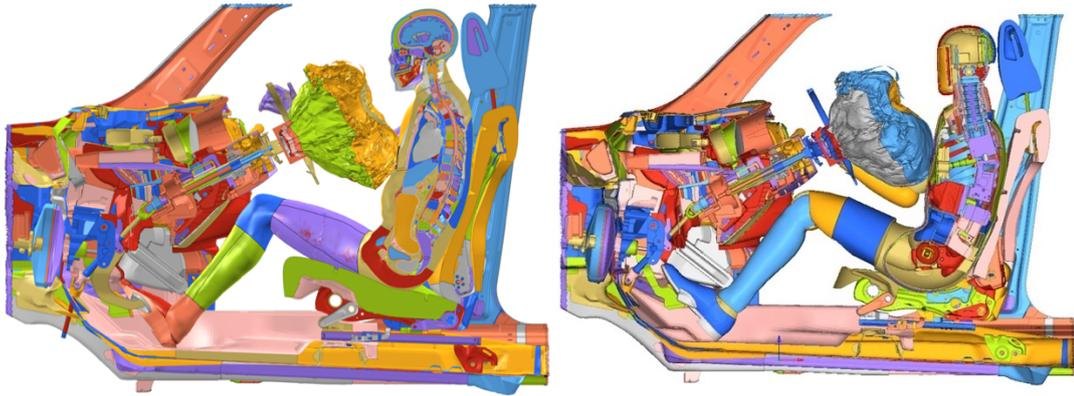
**Figure 5.46.** Positioned THUMS (left) vs THOR (right) - side  $xz$  section view – ODB – 30 ms
