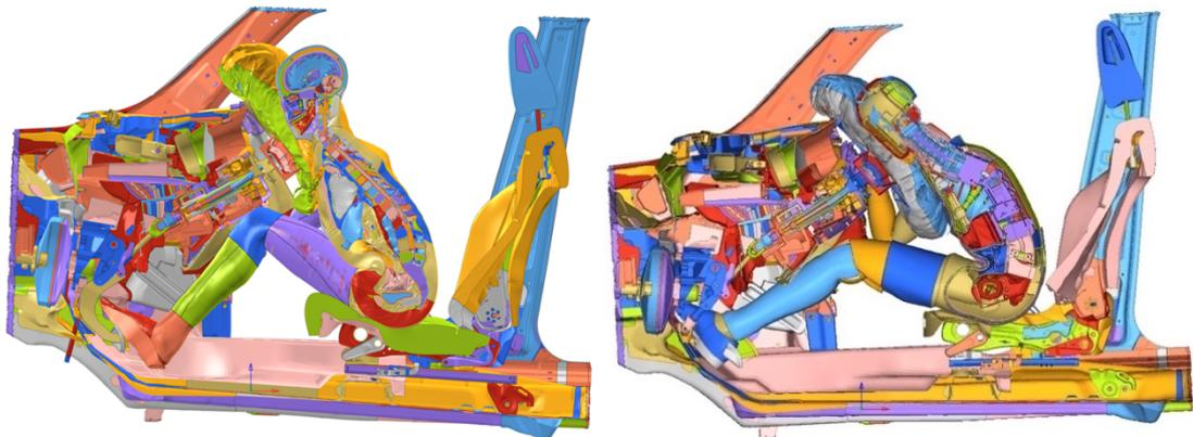
**Figure 5.14.** Positioned THUMS (left) vs THOR (right) - side *xz* section view – FWRB – 90 ms
