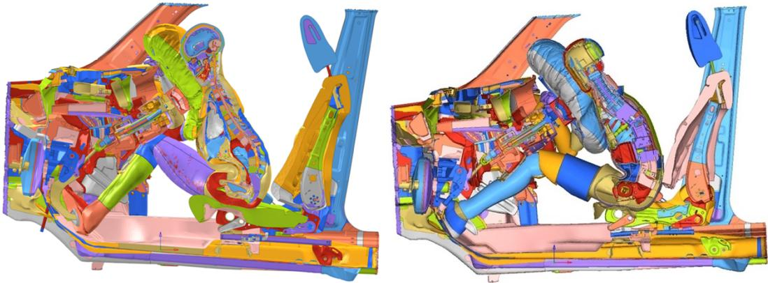
**Figure 5.13.** Positioned THUMS (left) vs THOR (right) - side *xz* section view – FWRB – 75 ms
