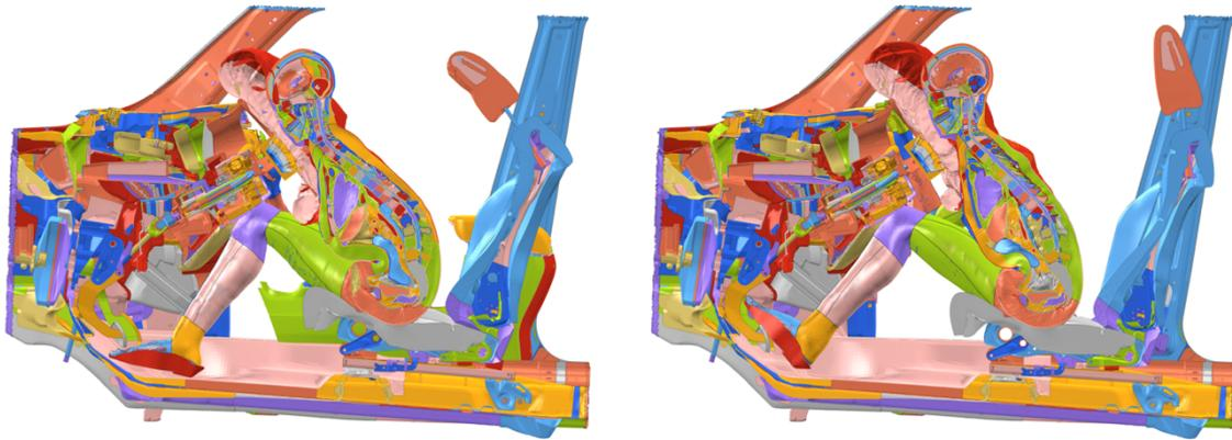
**Figure 6.10.** THUMS in OOP (left) vs THUMS in driving posture (right) - side xz section view – FWRB – 90 ms
