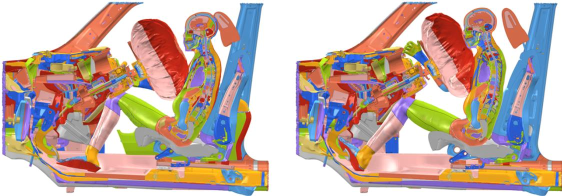
**Figure 6.7.** THUMS in OOP (left) vs THUMS in driving posture (right) - side  $xz$  section view FWRB – 45 ms
