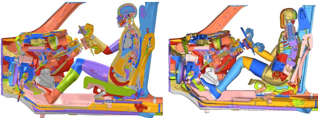
Figure 5.45. Positioned THUMS (left) vs THOR (right) - side  $xz$  section view – ODB – 15 ms
