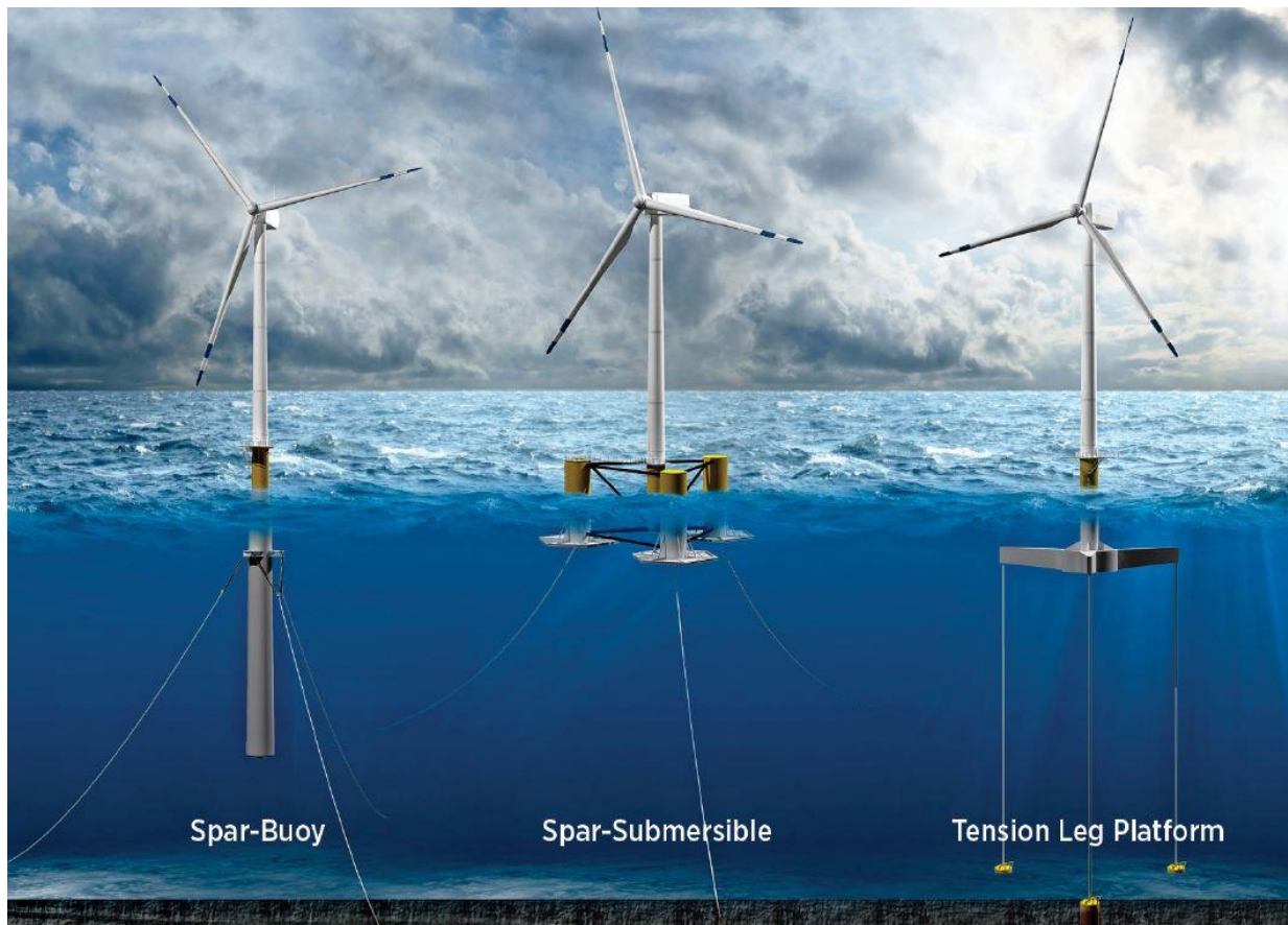
Figure 16: Different types of floating foundations available for offshore wind turbine; source: [12]
