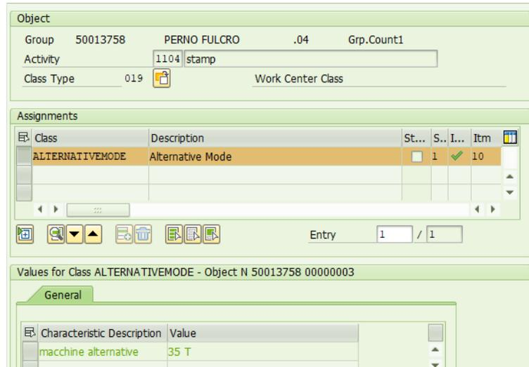
Figure 47. Routing with a group of alternative machines. Own creation.
