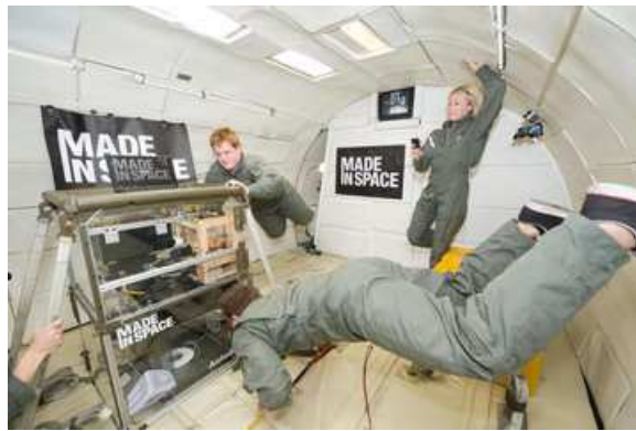
Figure 19. Test of a 3D printer in a zero-gravity chamber
