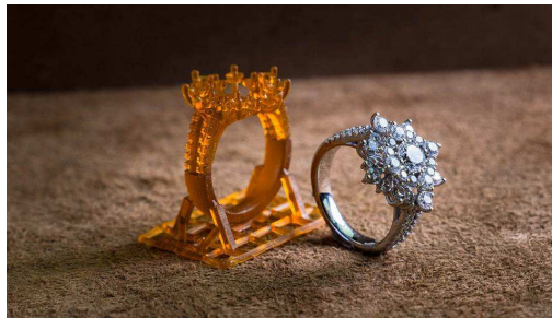
Figure 6. Ring created by casting technology using a DLP printed model (on the left)
