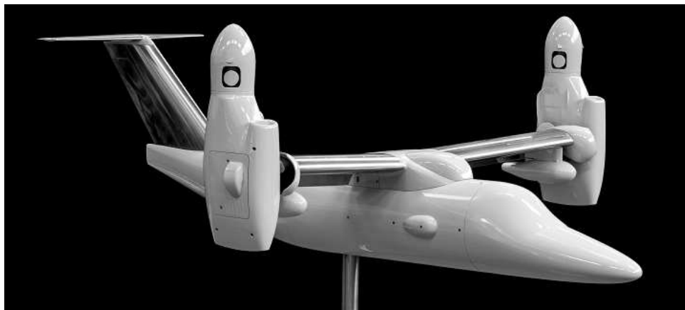
Figure 10. Aircraft Model for Wind Tunnel Testing printed used SLS technology
