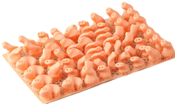
Figure 27. 3D printed hearing aids shells with customized for each patient's ears
