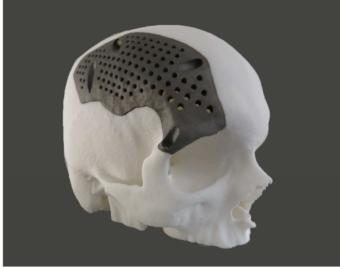
Figure 11. Titanium Skull Section printed by DMLS technology. Customization has a crucial role for prostheses creation.
