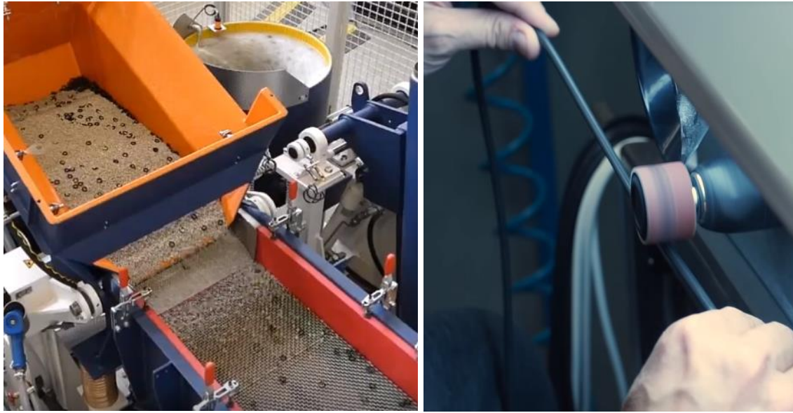
Figure 8. Grit blasting and buffer processes (Precision Polymer Engineering Ltd, 2018).
