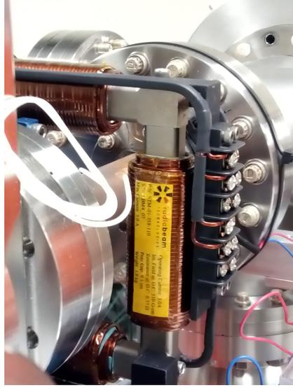
Figure 66: Steering magnets for the deflection of the electron trajectory.
