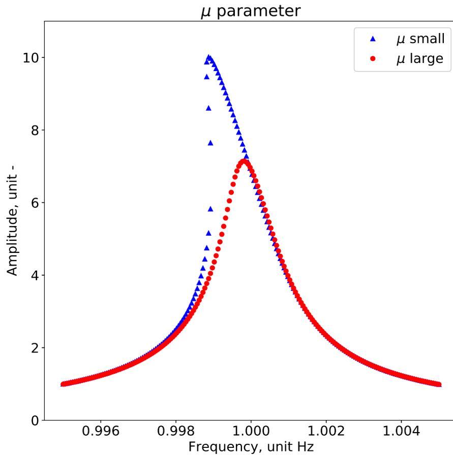
**Figure 3.4:** The parameter  $\mu$  is inversely proportional to the quality factor. This image was generated through Python script
