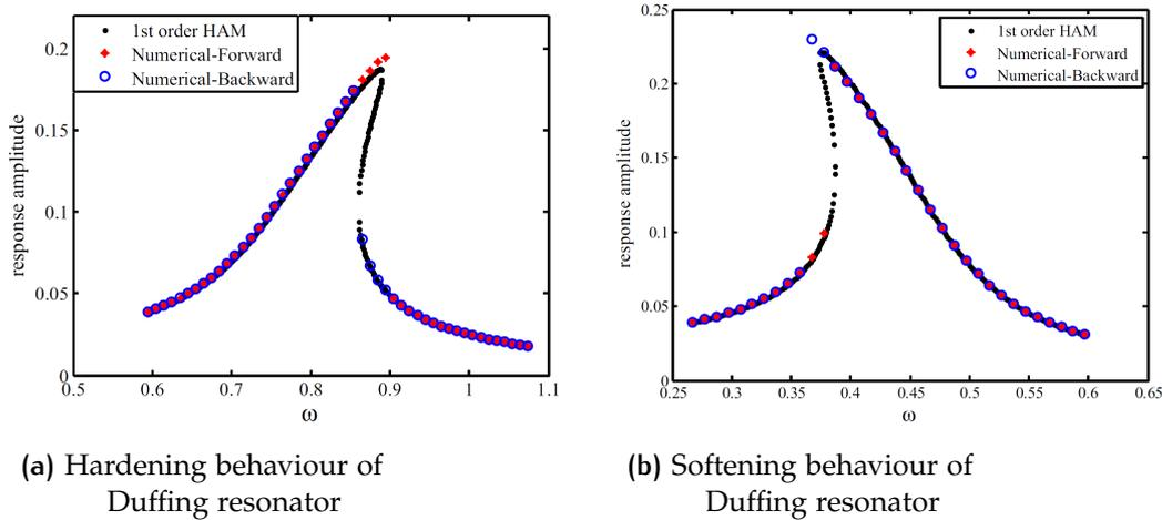
**Figure A.1:** Distortion of the transfer function of a typical non linear resonator. The oscillator's peak lean towards one of the plot's sides. Images were extracted from the article [4, Non linear dynamics of MEMS/NEMS resonators] page 1919
