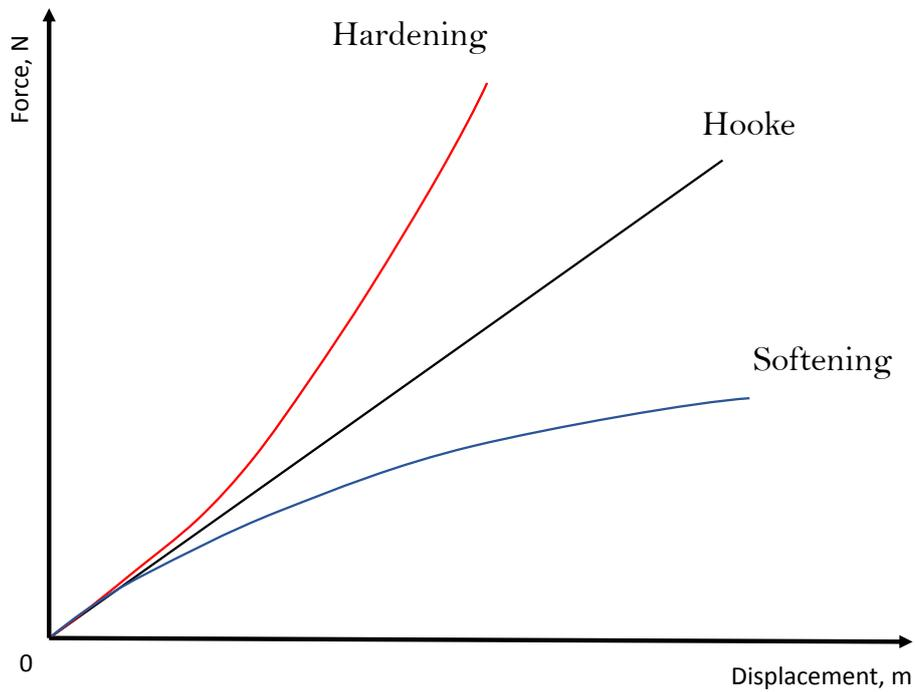
**Figure A.2:** This figure describes the deviation from the Hooke's law. The red curve represents an hardening type spring, the blue curve a softening type and the black line the Hooke's law. This image was generated through Microsoft PowerPoint
