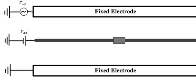
**Figure A.3:** Schematic of a straight beam with double clamped electrodes, a DC potential is applied to the beam while an oscillating actuation potential is applied to the top electrode. Images were extracted from the article [4, Non linear dynamics of MEMS/NEMS resonators] pag. 1919
