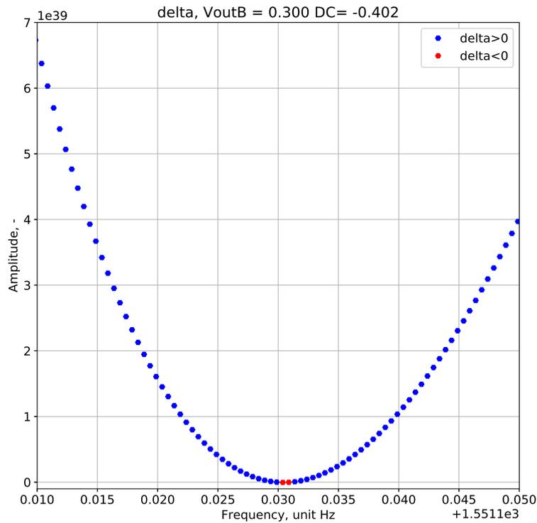
**Figure 4.1:** Delta values of a specific sensor, the red points in the middle of the figure represent the bistability of the device near its resonance frequency. This image was generated through Python script
