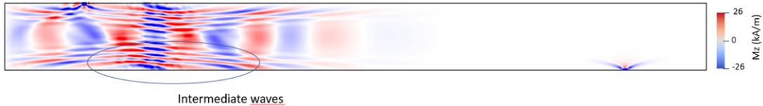
Figure 5.2: The snapshot is taken at 0.5 ns. The intermediate waves become more relevant as the time flows, but far from the antenna the pattern is still the same as that one of the begin.
