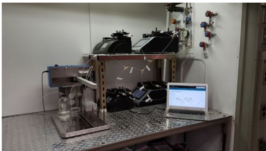
Fig. 2 Photograph of the flow reactor set up
