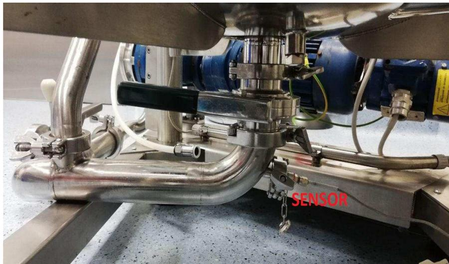
Figure 4.4. Temperature sensor piping
