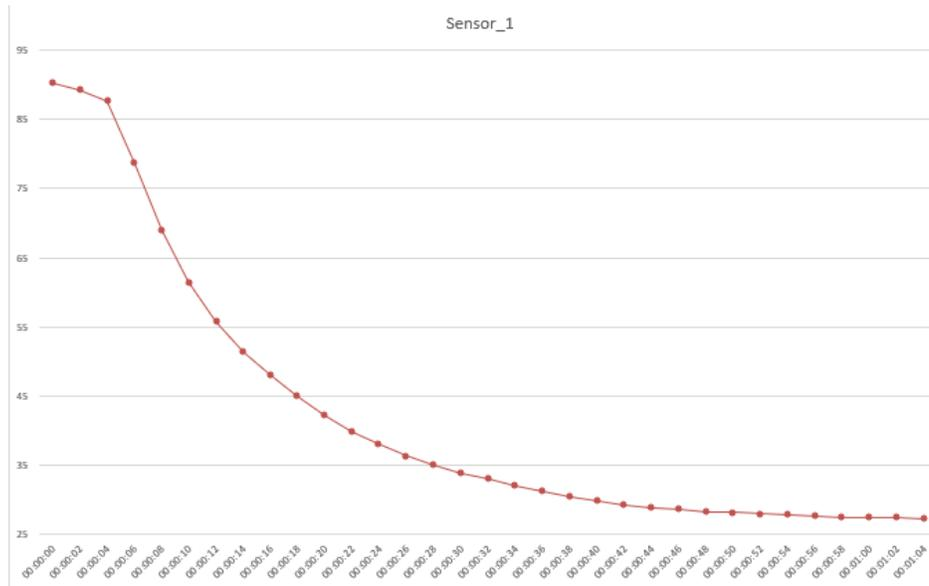
Figure 3.7. Temperature difference 90°-27°C results sensor 1
