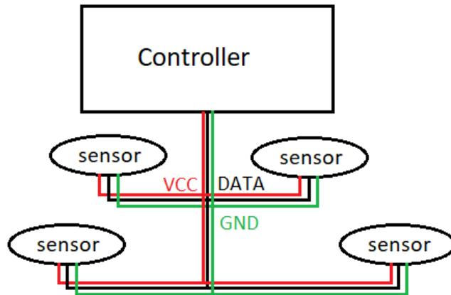
Figure 2.12. Simple example of connection
