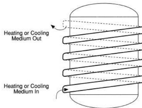
Figure 1.2. Heat transfer with half-pipe approach
