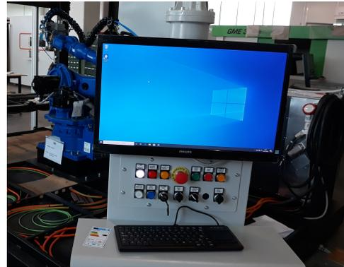
Figure 65 – Control panels of the cell. On the left, the main tab of the menu available on the teach pendant; on the right, the HMI with buttons and Windows environment.
