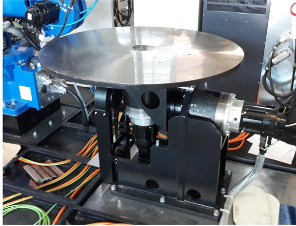
Figure 56 – Detail of the two motors that move the axes of station S2.
