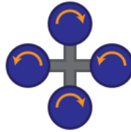
Figure 1.2: Quadcopter rotors direction of rotation. From [29]
