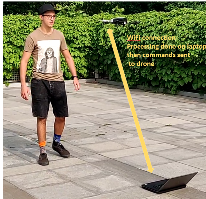
Figure 6.7: IBVS system: processing on laptop and commands sent to drone
