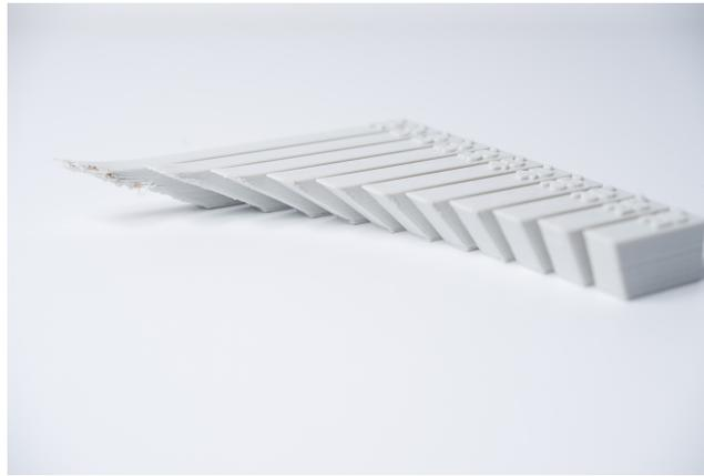
Figure 39 – Printed part with gradually increased inclination, (35)
