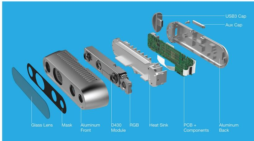
FIGURE 5.5: Internal hardware components of Intel® RealSense™ Depth Camera D435i [34].
