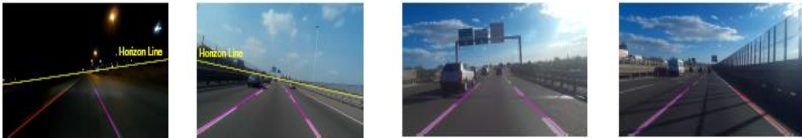
Figure 1. 5 Nava et al [4] demonstrates horizon line identification and lane detection in day light and night situation
